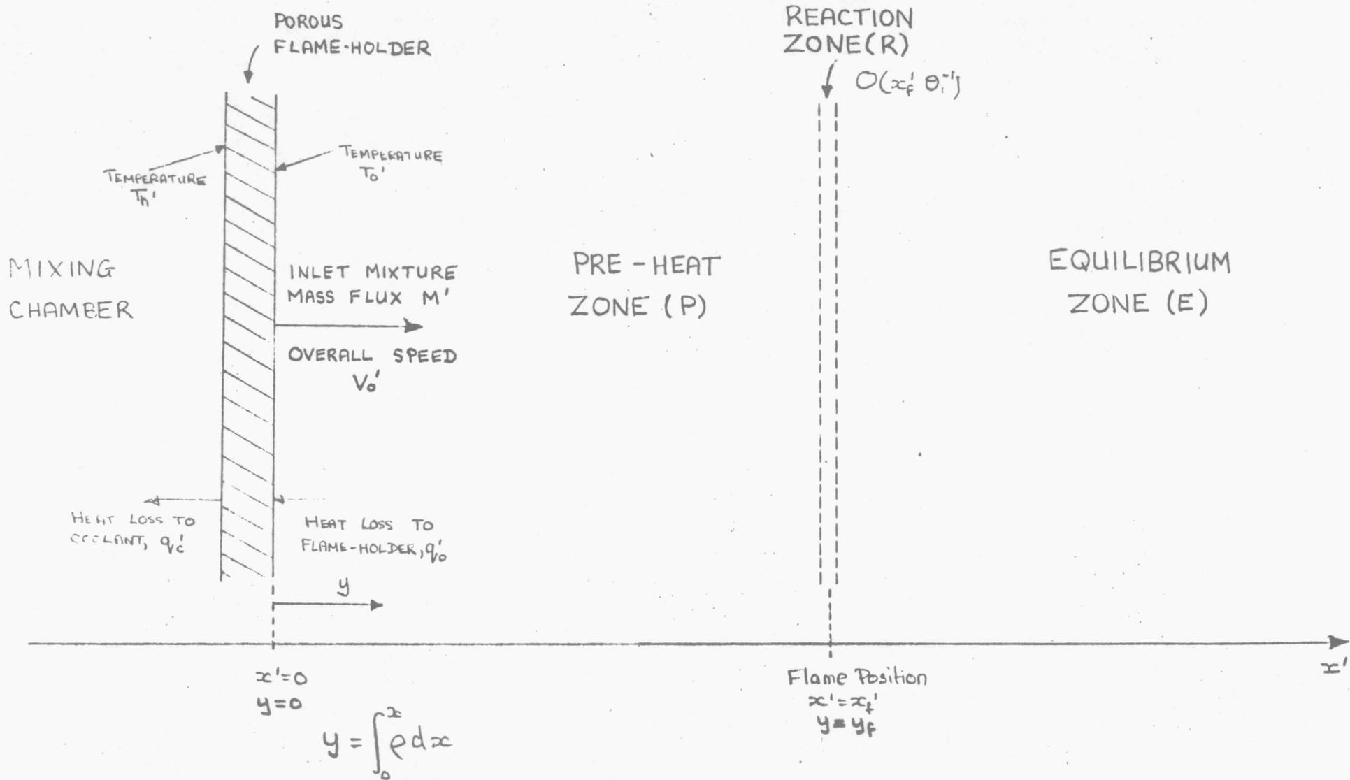
FIG. 1. SCHEMATIC OF ONE-DIMENSIONAL PRE-MIXED FLAME WITH FLAME-HOLDER.
