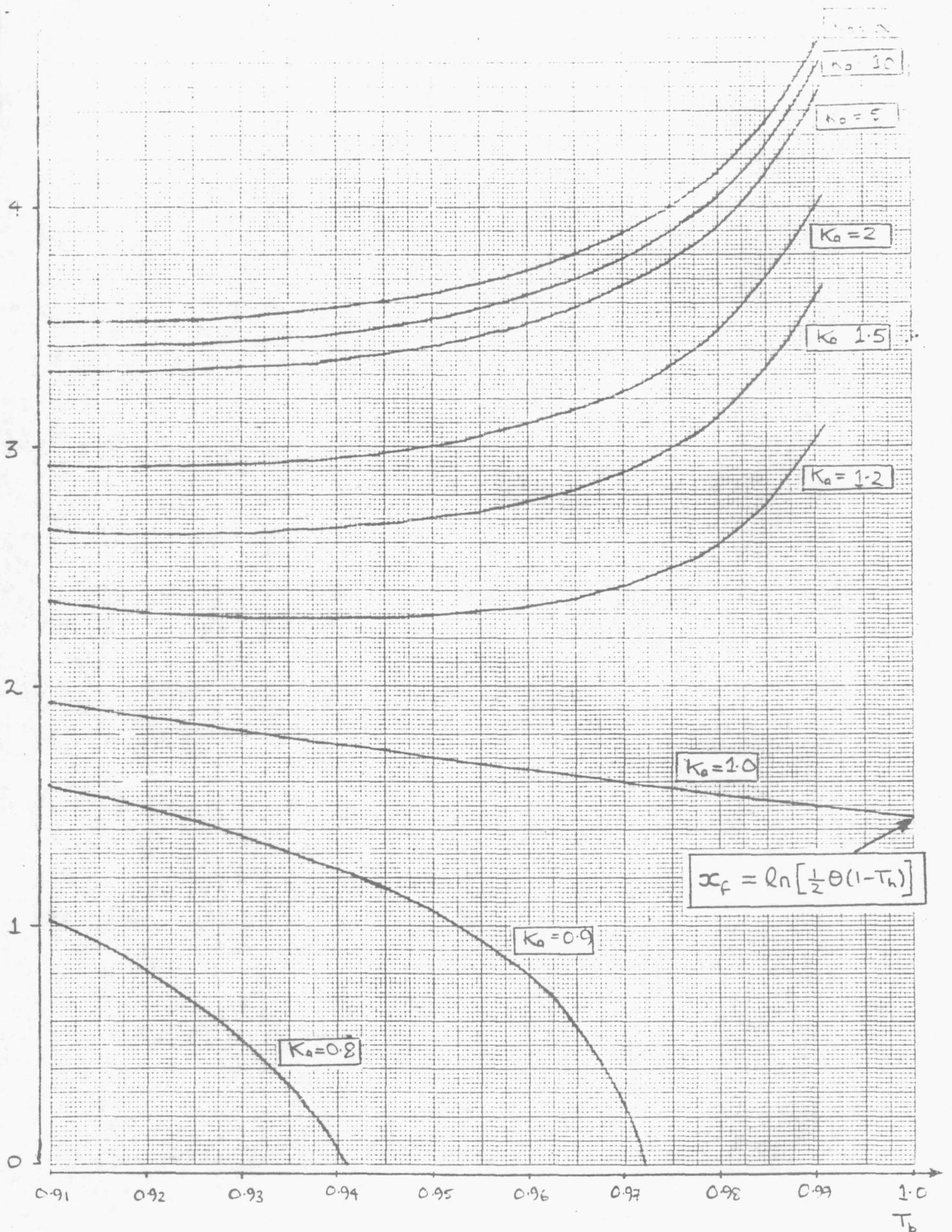
FIG. 4 STAND-OFF DISTANCE VERSUS TEMPERATURE USING EQUATION (6.16).  $\theta = 10$ ,  $T_h = 0.15$ . VARYING CONDUCTANCE  $K_a$ . NOTE USUALLY  $K_a > 5$ .
