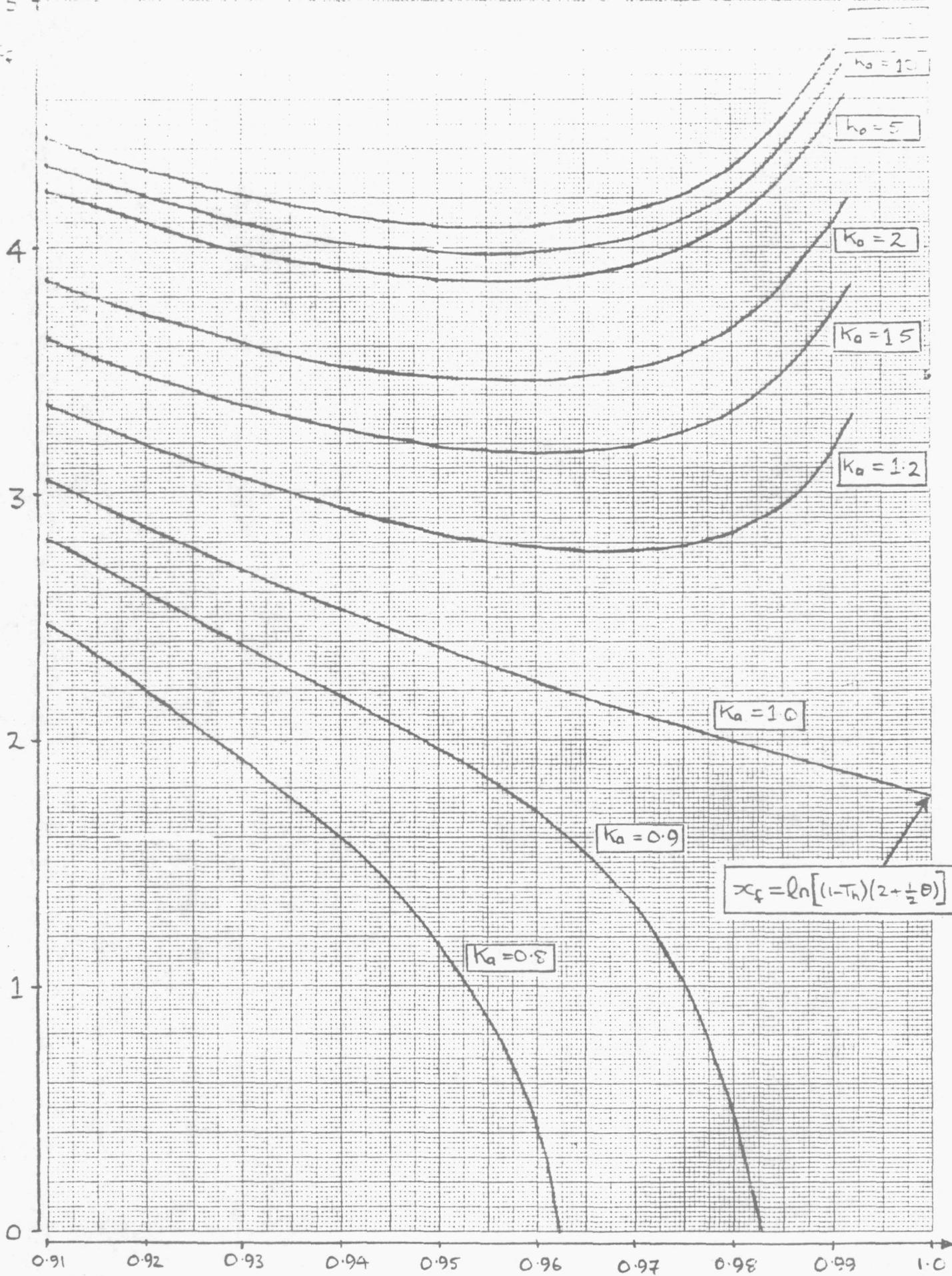
FIG. 3 STAND-OFF DISTANCE VERSUS TEMPERATURE USING EQUATION (6.10b).  $\theta = 10, T_h = 0.15$ . VARYING CONDUCTANCE  $K_a$ . NOTE USUALLY  $K_a > 5$ .
