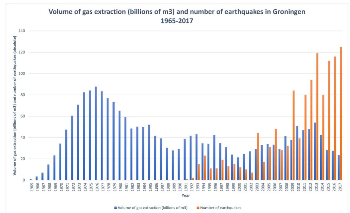
Figure 19. The volume of gas extraction and the number of earthquakes in Groningen
