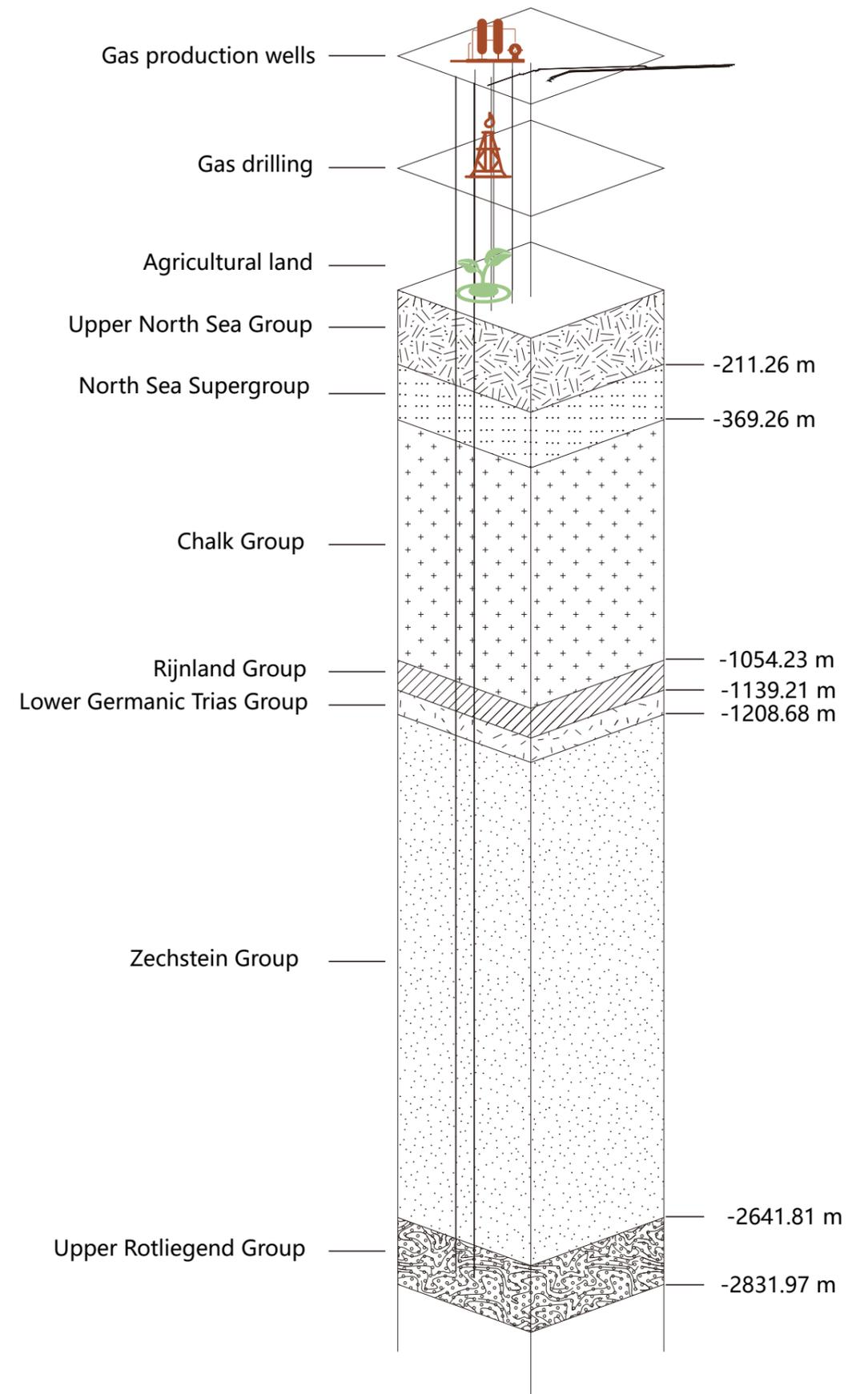
Figure 7. The Groningen gas reservoir are located approximately 3 kilometers below the surface, and the extraction wells and infrastructures built on agricultural lands.
