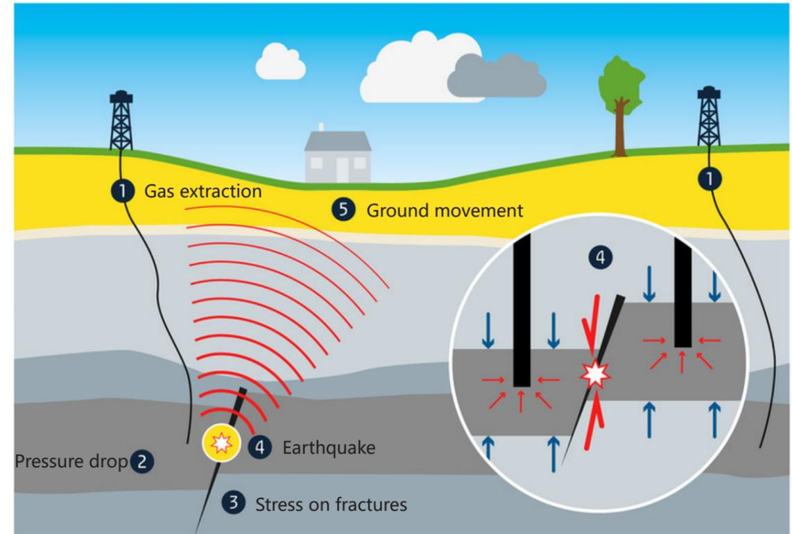
Figure 18. Situation drawing: Groningen gas field earthquake
