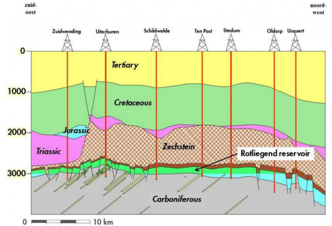
Figure 9. Geological cross section of the natural gas field in Groningen.
