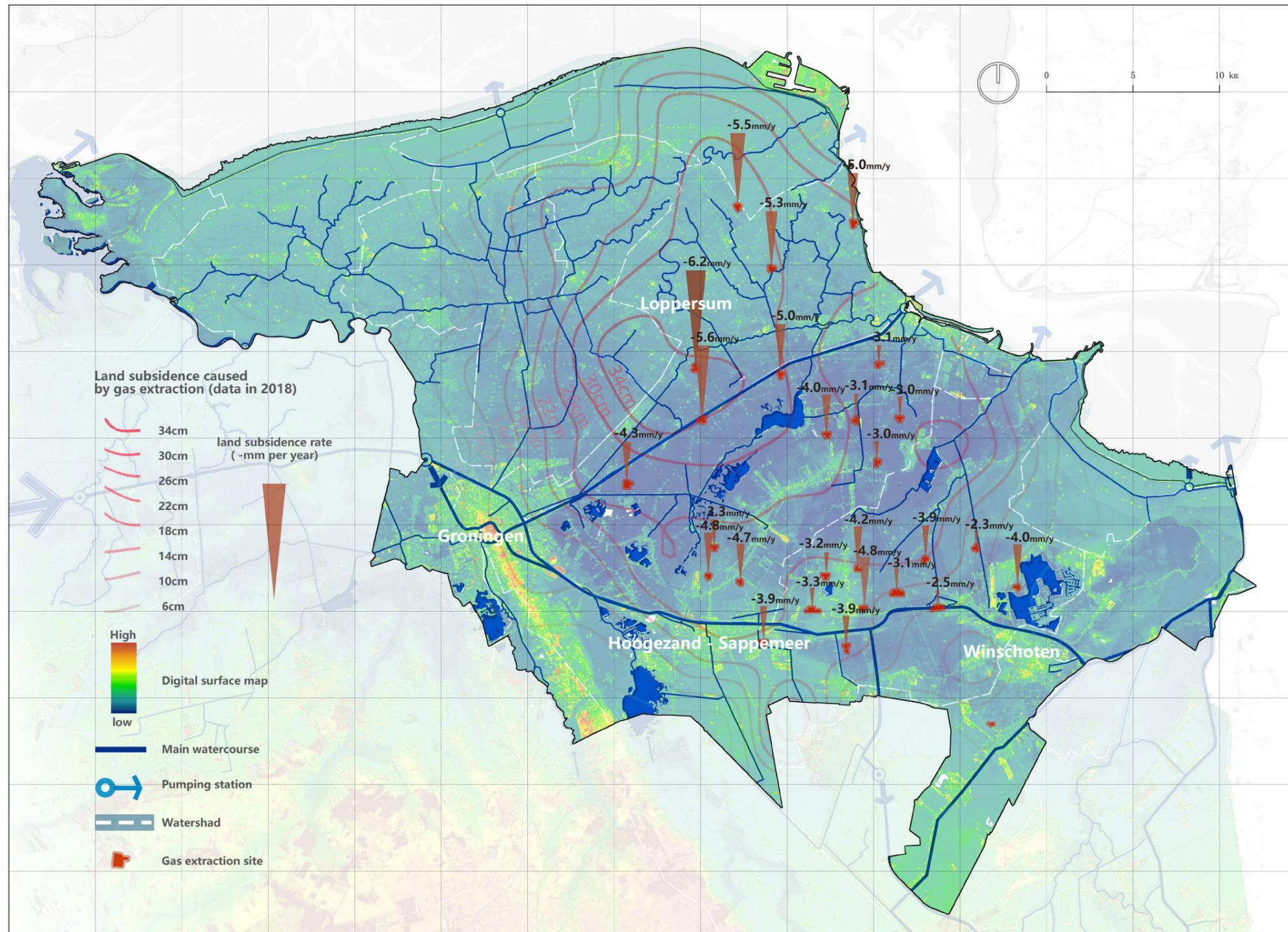
Figure 33. Mapping of main watercourses, land subsidence contour line and subsidence rate data observed in each gas extraction location in Groningen
