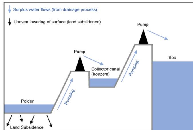
Figure 28. Cross-section of drainage process which illustrates how the discharge of surplus water is complicated by land subsidence
