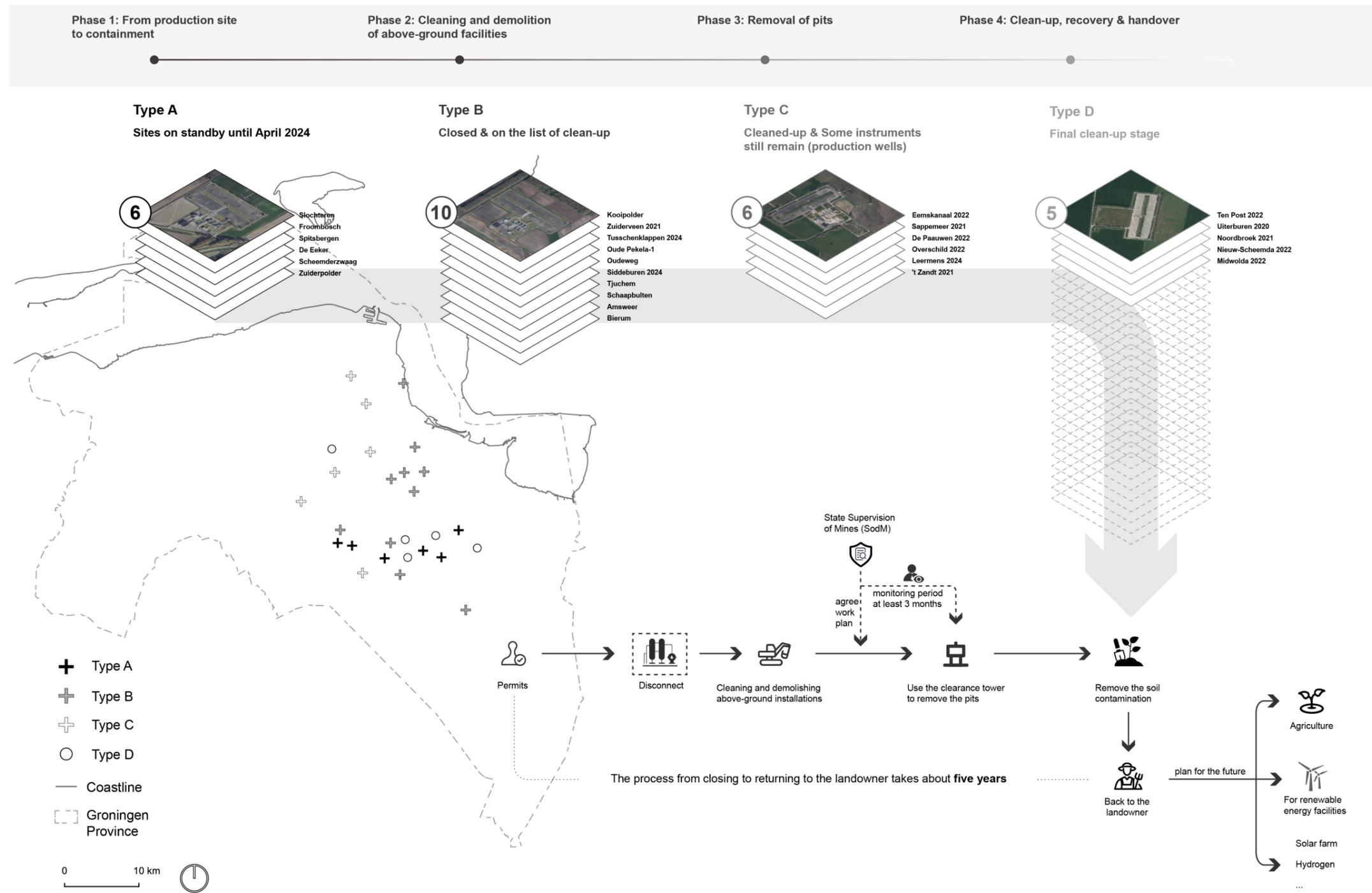
Figure 42. Groningen gas production site decommissioning process
