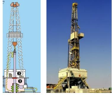
Figure 5. Derrick, drill bit and pipes used for drilling natural gas in Groningen gas field. Image from: https://gasuitgronigen.jouwweb.nl/ Gas drilling
