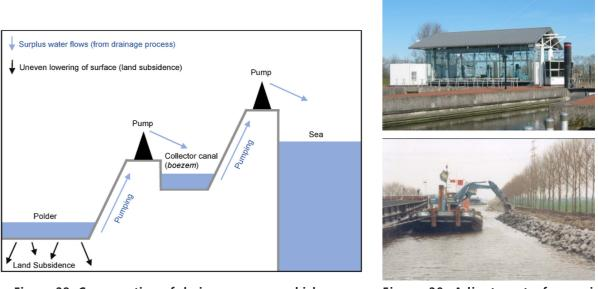
Figure 28. Cross-section of drainage process which illustrates how the discharge of surplus water is complicated by land subsidence Image from: Hannah Porada, 2024
