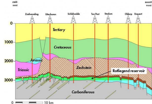
Figure 9. Geological cross section of the natural gas field in Groningen. Please note: for the sake of a good display, the vertical scale (in meters) is a lot larger than the horizontal scale. Image from: Groningen Extraction Plan 2016, NAM.
