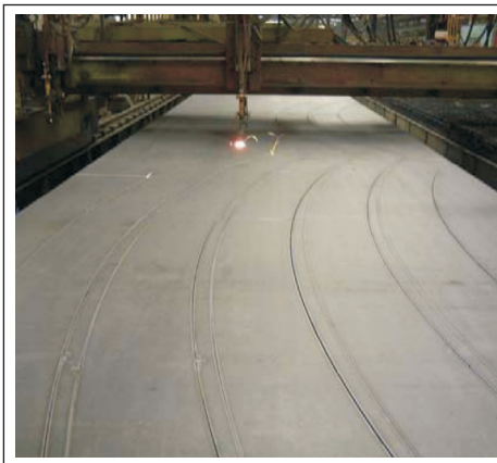
Figure 4.16: Sheet steel cut with flame cutters
