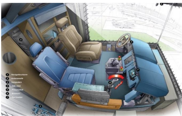
Figure 1: Illustration of HMI Lab. The participant will be sitting on the right (blue) seat and controls the side-stick. The participant will have to look at a tablet on the left.
