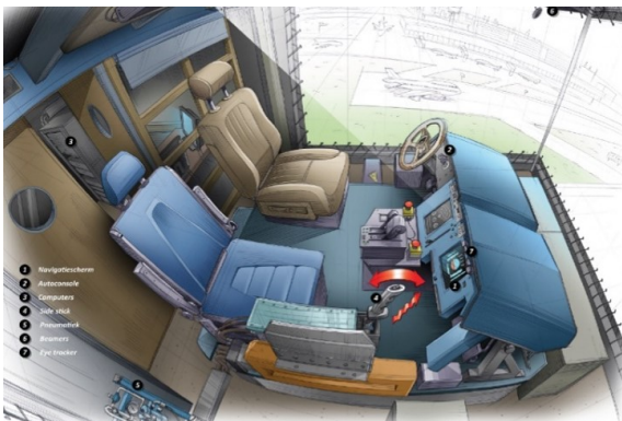
Figure 7.1: Illustration of HMI Lab. The participant will be sitting on the right (blue) seat and controls the side-stick. The participant will have to look at the screen on the left [1].
