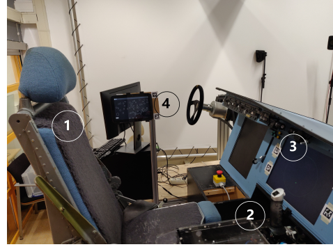
Fig. 1. Experiment set up in the HMI Lab. The participant will be sitting on the right (blue) seat and controls the side-stick.
