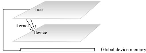
Kernels consist of numerous threads grouped into thread blocks. For us the thread blocks represent the local particle filters, while the threads the particles. Different threads have access to fast limited shared memory inside the thread block and they can write and read data from the slower access global device memory.
