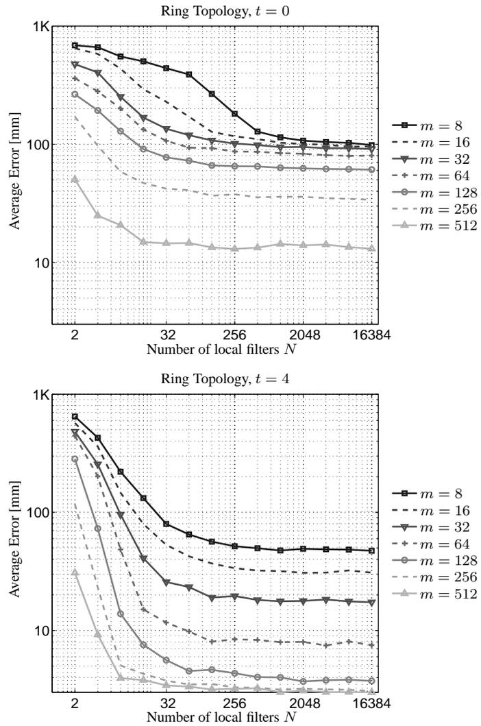
**Figure 3.7:** Average error for different  $(N, m)$  settings varying the number of shared particles  $t$ .
