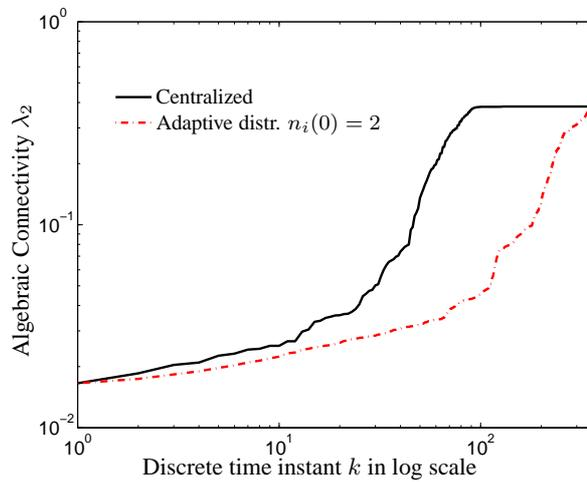
**Figure 4.7:** Algebraic connectivity as a function of time  $k$  for both the centralized and the distributed solutions of Figure 4.8.
