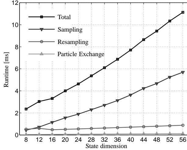
**Figure 3.8:** Runtime of the some of the kernels of the distributed computation Particle Filter implementation varying the state dimension in the setting  $N = 2048$  and  $m = 512$ .
