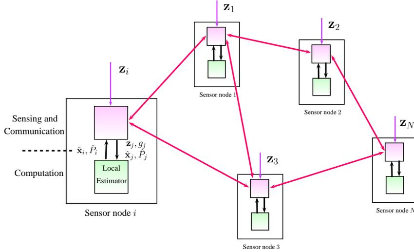
**Figure 2.1:** Proposed distributed (sensing) framework for the estimation problem. We note that each of the local estimators has the same input-output structure to allow the possibility to “plug and play” different local filters.
