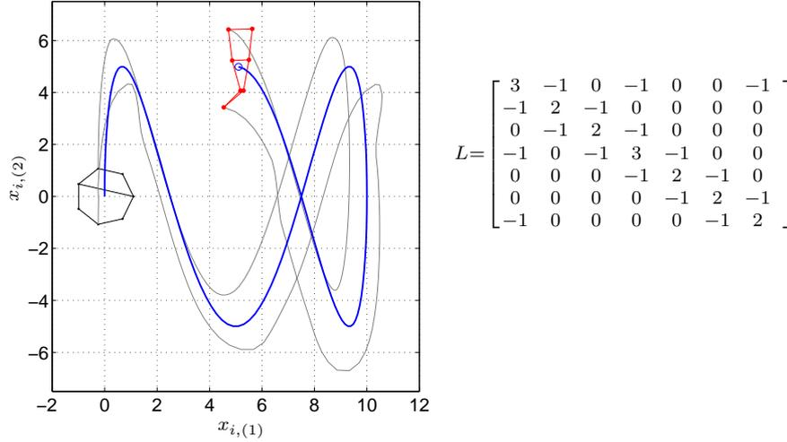
**Figure 5.1:** Representation of the trajectories of two robots while the target moves (blue thick line). The initial graph and positions of the robots are marked in black, while the final configuration is marked in red. The notation  $x_{i,(j)}$  indicates the  $j$ -th component of  $x_i$ .
