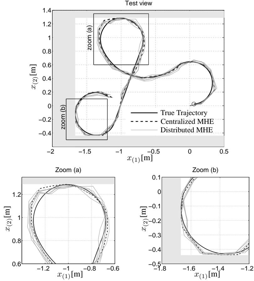
**Figure 2.4:** Results of a representative simulation run. The initial position of the robot is marked with a circle, while the shaded areas represent position constraints.
