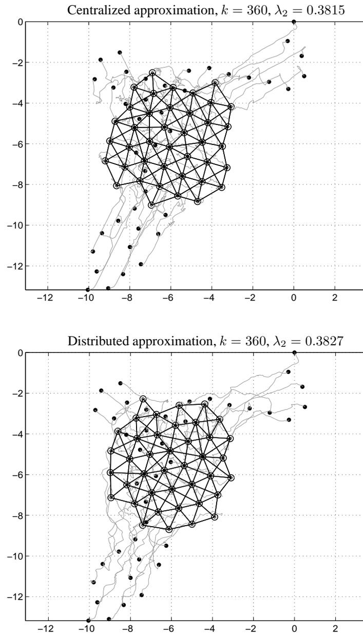
**Figure 4.8:** Simulation results of the centralized and distributed approach (adaptive case). The initial positions are marked with black dots. The final positions are marked with circles. The bold lines represent the final communication graph and the thin lines the agent trajectories.
