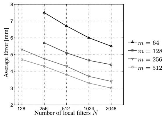
**Figure 3.4:** Averaged estimation error  $e$  in a number of experiments with different  $(N, m)$  settings. The standard deviation, not depicted, is around 1 mm.
