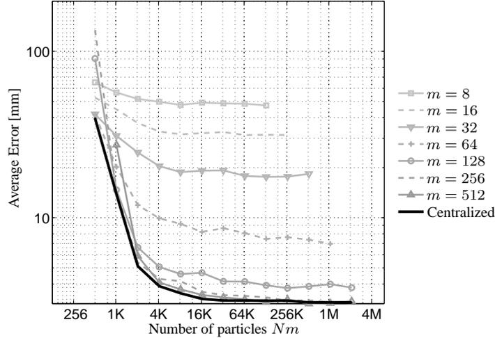
**Figure 3.10:** Comparison of the estimation error between distributed implementation and centralized one.
