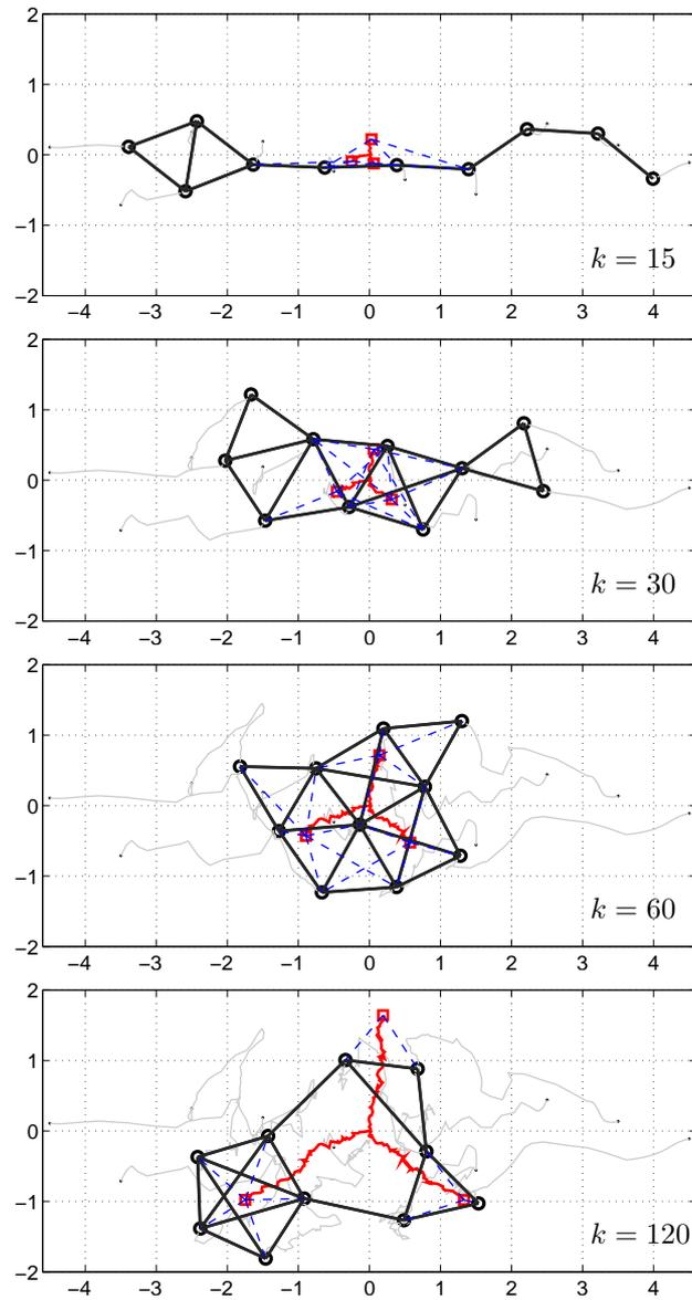
**Figure 4.12:** Distributed approximations at four different discrete time instants. The thin black lines represent the agents' trajectories, which start from the points marked with small black dots. The targets' trajectories are in red and start from  $(0,0)$ . Black circles represent the agents, squares the targets, solid lines are the communication links and dashed lines the detection links.
