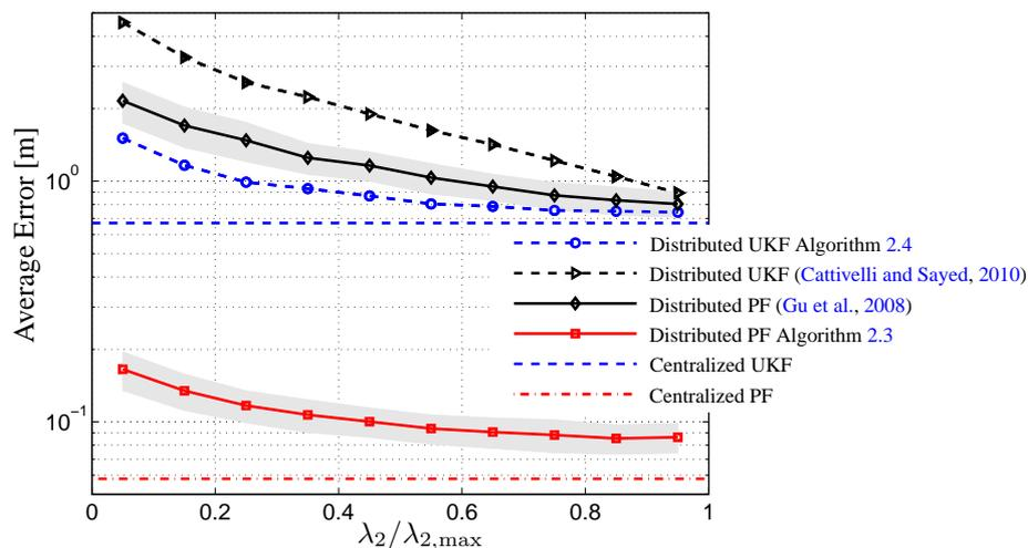
**Figure 2.6:** Comparison between the proposed algorithms and the one in the literature with respect to the normalized algebraic connectivity of the information exchange graph. The average error is computed as the mean error of the sensor averaging 2500 different simulations. The shaded areas are the standard deviations. The DUKF's standard deviation are not depicted. The straight lines correspond to the centralized UKF, and the centralized PF.
