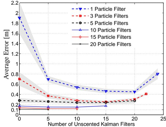
**Figure 2.7:** Results for different filters running on different sensors. The Average Error is computed as the mean error of the sensor averaging 1500 different simulations. The shaded areas are the standard deviations of the bold lines. Since the number of sensor is fixed ( $N = 25$ ), one can compute the number of EKFs present in the network from the knowledge of the number of Particle Filters and UKFs.
