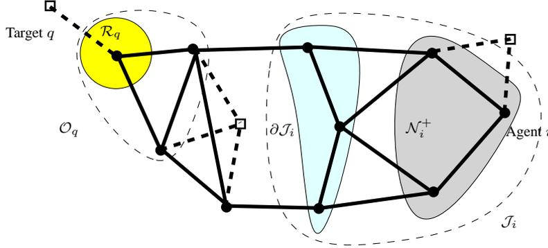
**Figure 4.10:** Notation for the distributed solution. The targets are represented via squares, while the agents are circles. Communication links are shown via solid lines and detection links via dashed lines.
