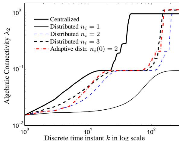
**Figure 4.6:** Algebraic connectivity as a function of time  $k$  for both the centralized and the distributed solutions of Figure 4.4 and 4.5.
