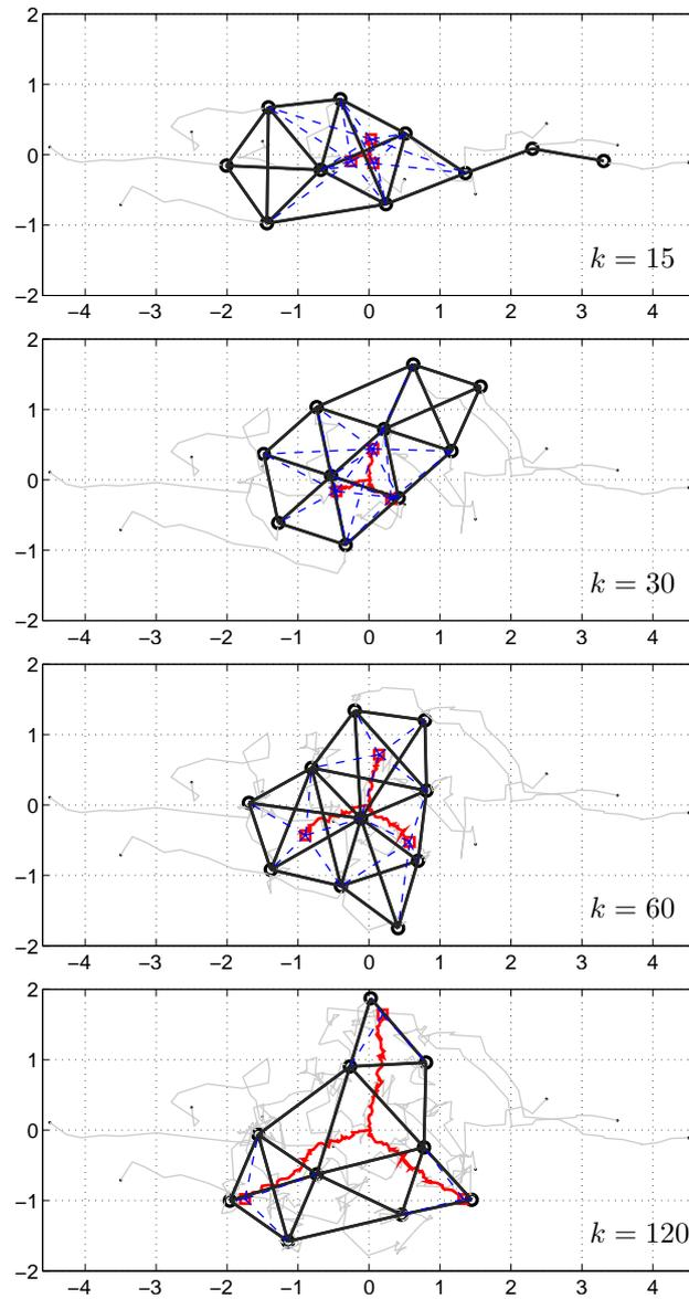
**Figure 4.11:** Centralized approximations at four different discrete time instants. The thin black lines represent the agents' trajectories, which start from the points marked with small black dots. The targets' trajectories are in red and start from  $(0, 0)$ . Black circles represent the agents, squares the targets, solid lines are the communication links and dashed lines the detection links.
