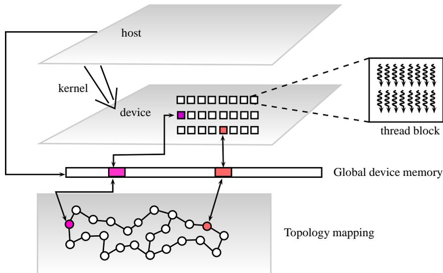
**Figure 3.2:** Basic concept of GPU architectures as available in CUDA. The global device memory is mapped into a specific topology representing data-exchange between thread blocks.
