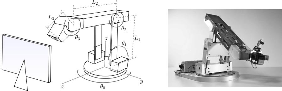
**Figure 3.3:** Robotic arm used for the experimental test. On the right the real tested and on the left a schematic representation showing the camera at the end effector, marked with a grey circle, and the monitor on which a moving object is displayed.
