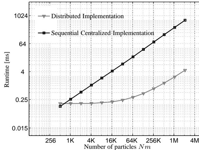
**Figure 3.9:** Runtime comparison of the proposed distributed implementation and a sequential centralized implementation. In the distributed one we fix  $m = 512$  and we vary  $N$ .
