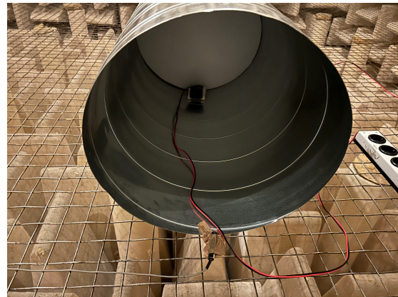
Figure 3.3: Speaker and insulation foam placement inside the big pipe. The foam is positioned in the middle of the pipe and the other speaker is positioned in the same manner on the other side of the foam layer.
