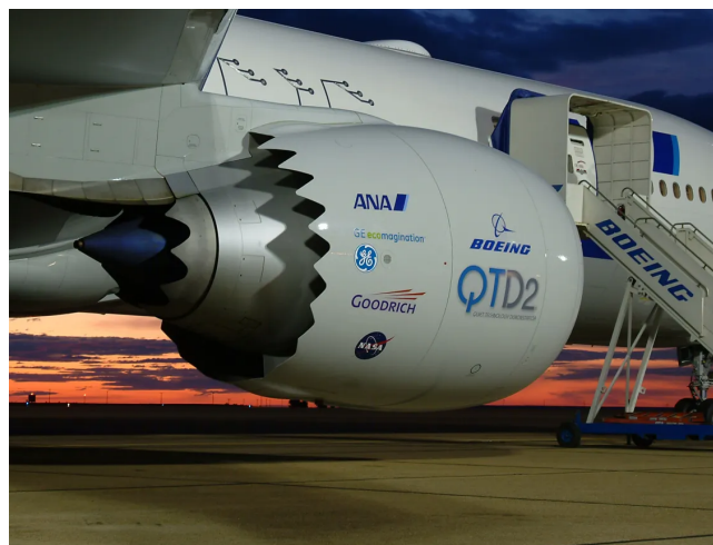
Figure 2.3: Chevrons on GE engine mounted on a Boeing 777 to reduce jet noise [28]
