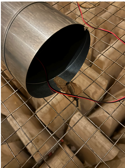
Figure 3.2: The reference microphone is placed at the exit of the pipe.
