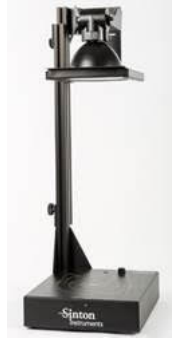
Figure 3.4: Quasi-steady state photoconductance measurement tool from Sinton instruments (Sinton WTC-120).
