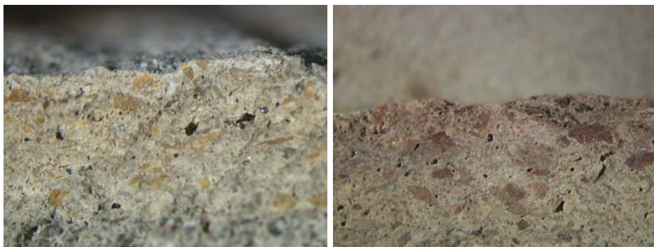
Figure 7.26 Stereo micrographic pictures from two differently coloured render samples of the emplacement of the Hofplein railway viaduct, both made with a greyish bottom layer (Portland cement based) and a coloured finishing layer with broken sandstone as aggregate (Pictures Laura Bolondi). a) Finishing layer is yellow-beige, the original colour (9 times magnification). b) The finishing layer is reddish due to colour changes of the sandstone aggregate caused during the fire in 1940.
