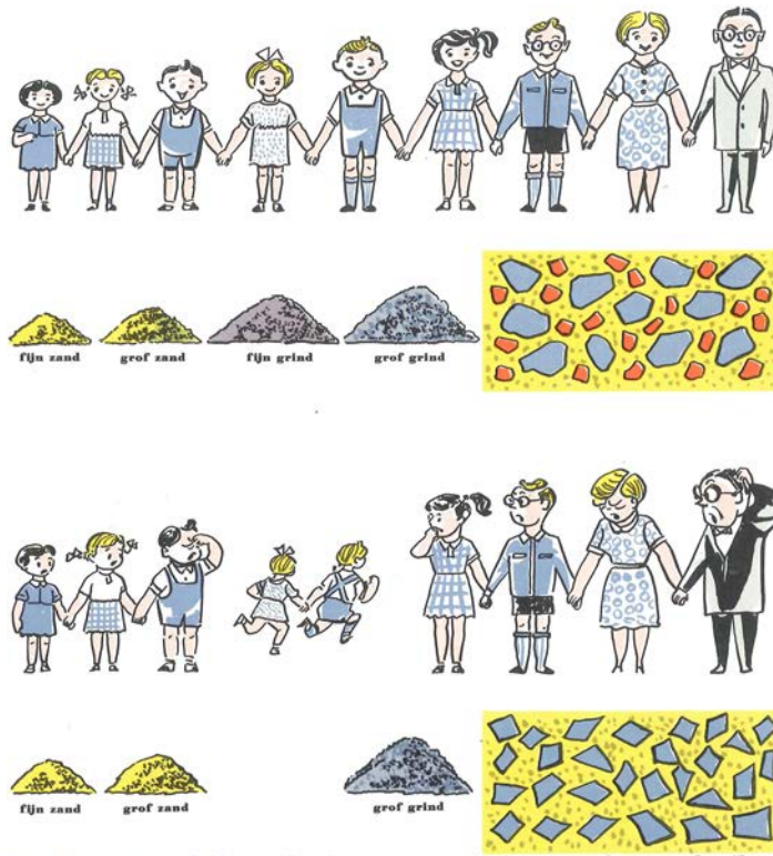
Figure 4.18 Popular illustration of the concept of continuous grading with all fractions present (top) and gap grading where some fractions are missing (bottom) (Anon., 1968, p. 13).
