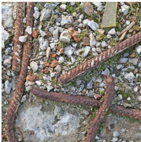
Figure 6.31 Ribbed reinforcement bars visible after demolition of a building on the Calve factory grounds probably dating back from the early 1960s (see Stenvert & Dekker, 2009)
