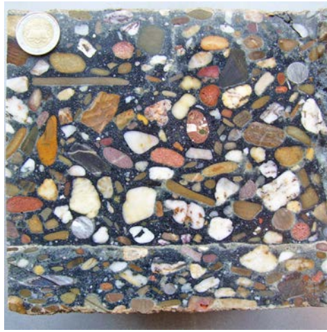
Figure 4.22 An early Dutch example dating from 1936 of gap-graded concrete made with blastfurnace slag cement (Sewage water reservoir, below the Jonas Daniel Meijer square, Amsterdam, picture 2008 by Timo G. Nijland).
