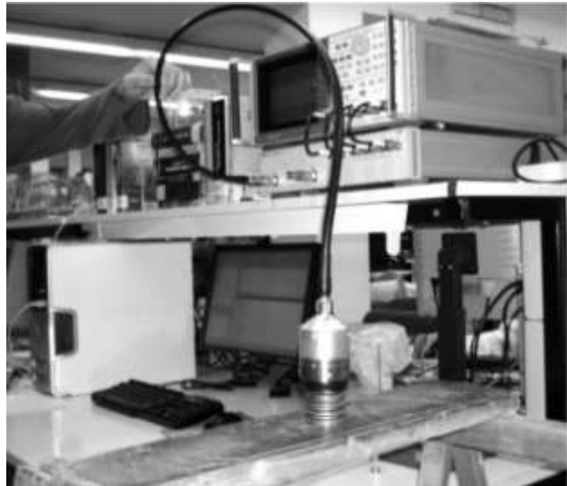
Figure 44: Experimental setup of open coaxial transmission line, source: (Torrents, Juan-García, Patau, & Aguado, 2009)
