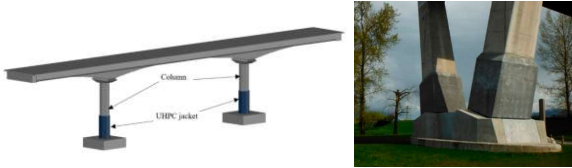
Figure 31: UHPFRC strengthened column bridge in Canada, source: (Kennedy, Habel, & Fraser, 2015)
