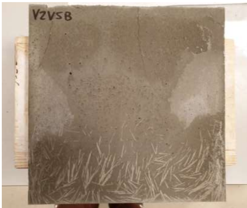
Figure 1: Steel fibers in UHPFRC plate specimen, picture taken by D. Kooreman
