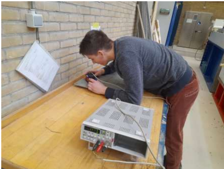
Figure 105: magnetic NDT method measurements with C-shaped ferrite core, picture taken by Y. Huang
