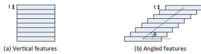
Figure 1: Staircase effect of printed layers on angled features results in increased roughness [9]
