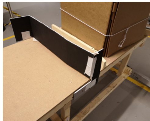
Figure 61 : Mockup of folding box guides
