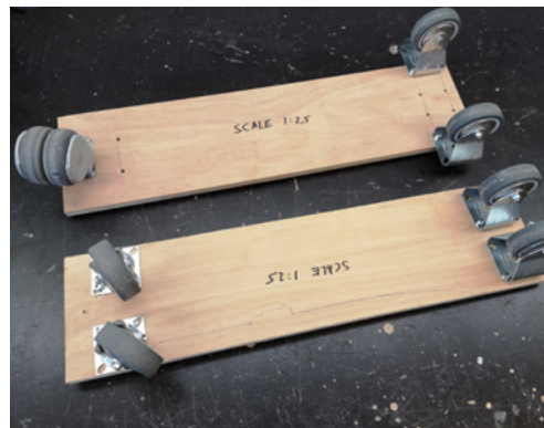
Figure 32 : Wheel configuration iteration
