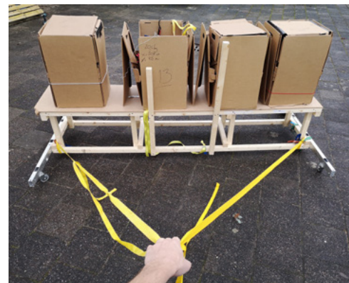
Figure 62 : Initial testing of towing feature
