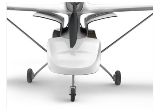
Figure 38 : Protruding wheel and wing strut
