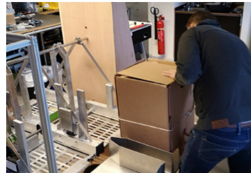
Figure 84 : Loading by sliding using UAV cargo bays
