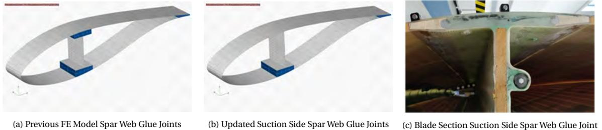
Figure 3.32: Blade Section Spar Web Suction Side Glue Joint Comparison
