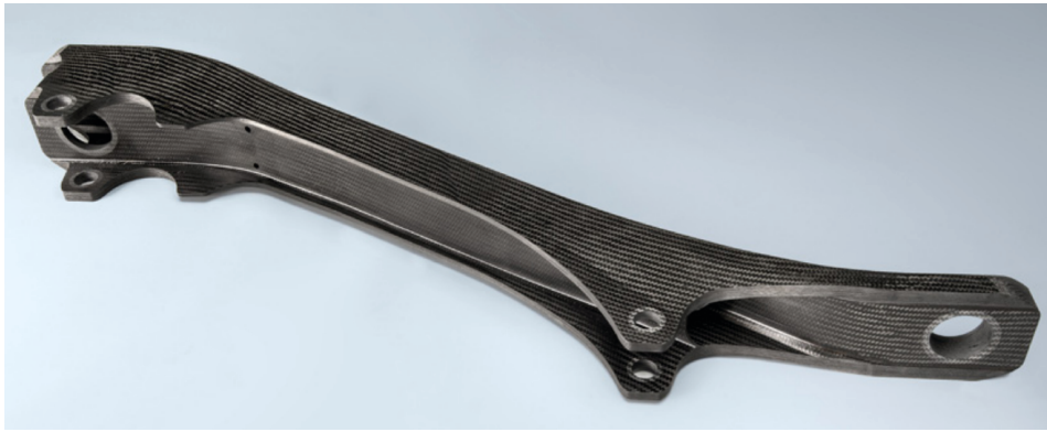
Figure 1.1: CFRP drag stay for the A350-1000, designed by FLG and NLR. Obtained from [4]
