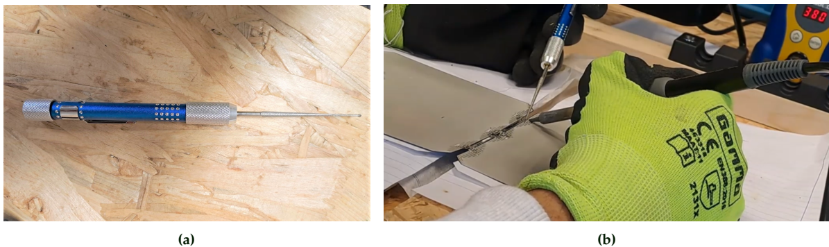
Figure 3.2: (a) Needle-file used for applying force on dog-bone, and (b) Desoldering process
