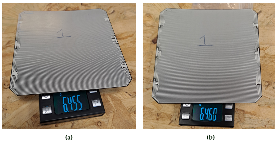
Figure 3.8: (a) Base weight of IBC solar cell, and (b) Weight of IBC solar cell with solder joints
