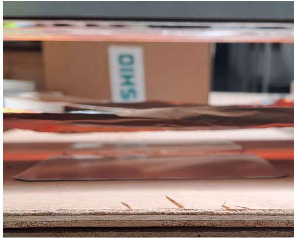
Figure 11: Solar cells soldered below the aluminum mask.
