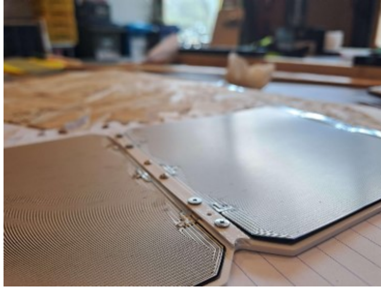
Figure 5.8: Initial Improved cell-bed with with single-strip based interconnection
