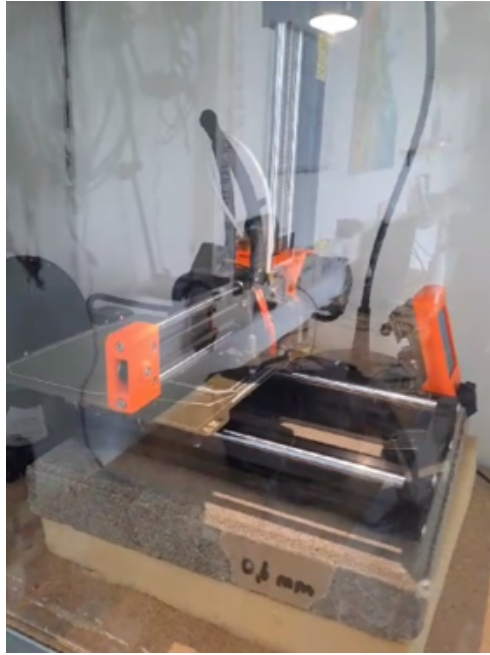
Figure 3.15: Printing improved cell-bed version 2 with ABS filament
