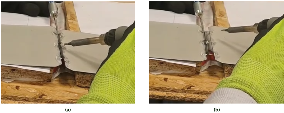
Figure 5.2: (a) Desoldering dog-bone soldered using SnBi solder alloy, and (b) Dog-bone desoldered from adjacent solar cell
