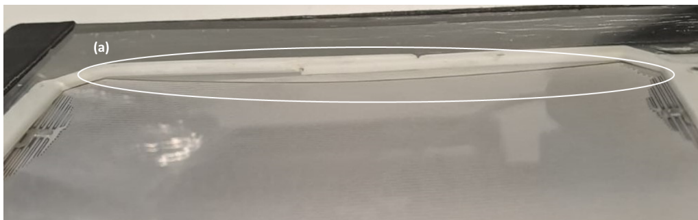
Figure 6.17: Warping of solar cell in the Cell-bed improved prototype
