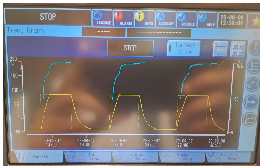
Figure 6.12: Trend lines depicting the thermal cycles (yellow, left y-axis) and change in relative humidity (blue, right y-axis)
