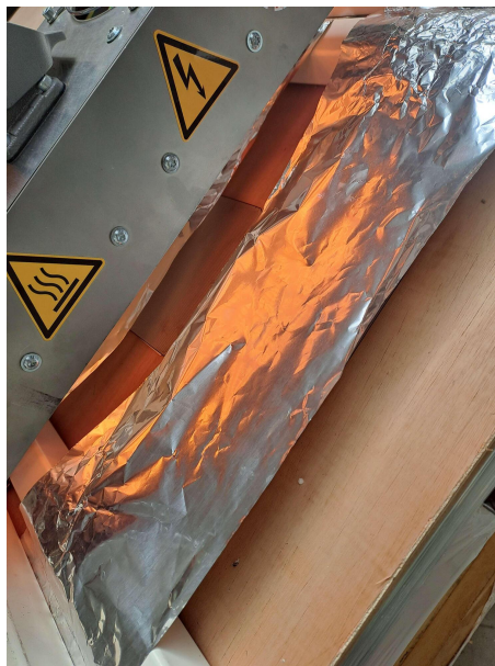
Figure 10: Aluminum foil mask placed above solar cells.
