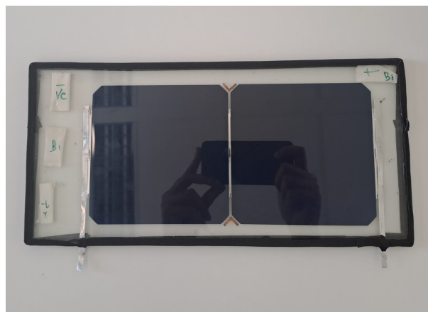
Figure 5.3: Prototype with cells soldered using Sn42Bi58 solder alloy
