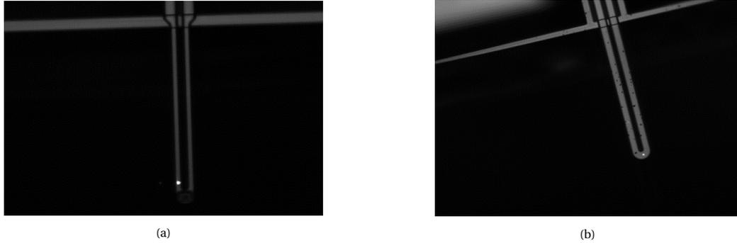
Figure D.2: (a) Old cantilevers with laser positioned on one leg. Laser point is clearly as wide as the leg of the cantilever. (b) New cantilevers with laser positioned at tip. The laser is now smaller than the width of the leg. Both images taken at 20X magnification.
