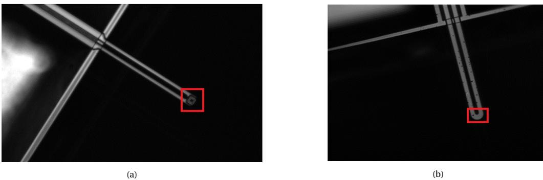
Figure D.1: (a) Old cantilevers with aperture at tip marked by the red box (b) New cantilevers without aperture at tip. The tip region is marked by the red box. Both images taken at 20X magnification.
