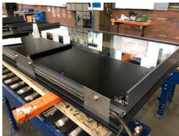
Fig. 25 – Installation of glazing and closure of backpan (source: own image)
