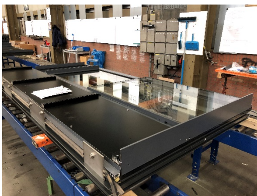
Fig. X – Installation of glazing and closure of backpan (source: own image)
