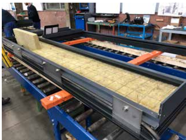
Fig. 25 – Installation of glazing and closure of backpan (source: own image)
