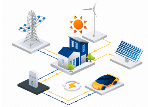
Fig. A1. Illustration of V2G integration. Adapted from Signature Electric (2018), “Vehicle-to-Grid: Delivering the Future of Energy.” Opportunities and Challenges of the Technology.
