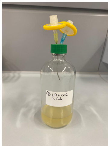
Figure 7.2: A photograph of the bottle used for the pure CO 2 atmosphere experiment. Each bottle is equipped with two needles fitted with 0.2 \mu m sterile filters, allowing the head-space to be flushed with nitrogen and then filled with the desired test atmosphere.
