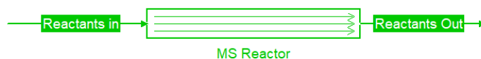
Fig. C.3. Visual representation of PFR component in process flowsheet environment of COCO™ simulator v3.2.0. Single phase PFR
