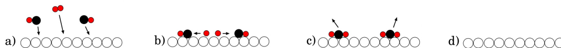
Fig. 2.7. Example process steps in catalytic reactions through adsorption with a single active site. a) Binding of molecules into surface layers. b) Splitting of molecules on the surface. c) Formation of new compounds. d) New formed species have weak bondings with the surface and are released leaving the catalyst “intact”.
