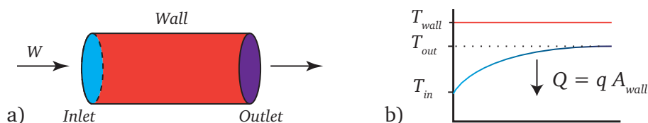
Fig. 2.24. Diagram for calculating U for a fixed temperature wall.
