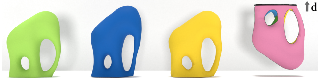
Fig. 3. Elephant model. (Green) Target shape \hat{X} . (Blue) Deformed shape \bar{X} before optimization has been performed, based on target geometry and panel initialization. (Yellow) Deformed shape \bar{X} resulting from optimization of rest shape X and orientation d . The shape is a close match to the target. (Far-Right) Final fabrication orientation d , suspension contact points denoted with thick black line. Panel segmentation corresponds to colors.
