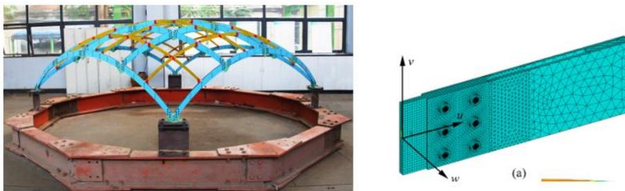
Figure 2.31: Grid shell and connection investigated by Ge et al. (2020)
