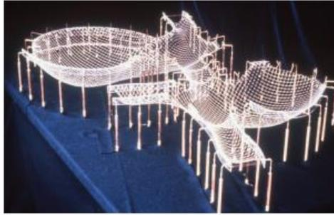
Figure 2.11: Hanging chain model of the Multihalle by Frei Otto (Adriaenssens et al., 2014)
