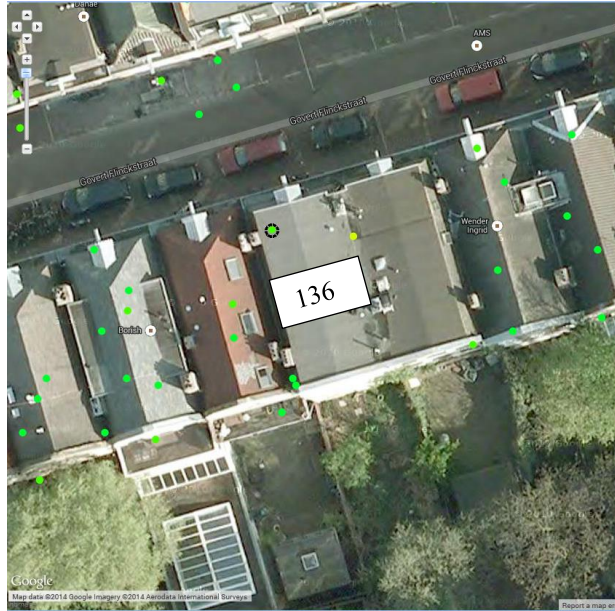
Figure 5 PS-InSAR reflection points on buildings, building 136 highlighted. The colour of the points indicate the linear deformation rate. Green is less than 2 mm/year, yellow is less than 4 mm/year.
