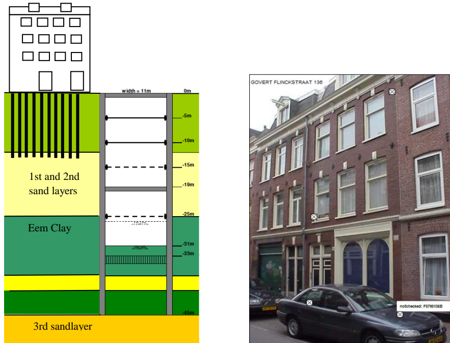
Figure 1 Cross section of Ceintuurbaan Station (left) and picture of Govert Flickstraat 136 (right). Squares with crosses are measurement locations (first and second floor prism locations and lowest level manual measurement bolts).
