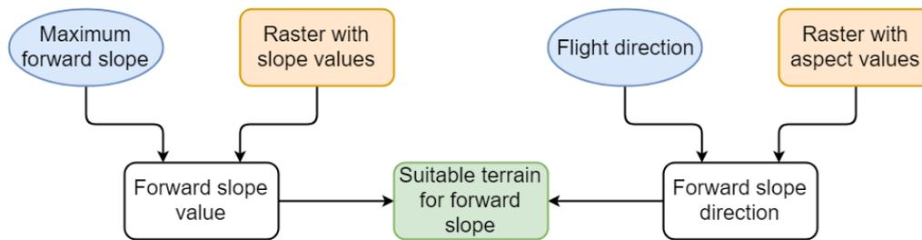
Figure 3.8: A visualization of how a suitable terrain is found for a forward slope. The raster with slope values and the raster with aspect values are combined with requirements for each of the rasters. The combination of the slope and the aspect will result in a suitable terrain. The suitable cells are given value 1. The other cells will get value 0.
