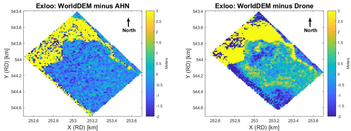
(a) Difference between the WorldDEM Digital Surface Model and the AHN2 Digital Surface Model. The color bar is limited so a more detailed overview is created of the potential touch down area.
