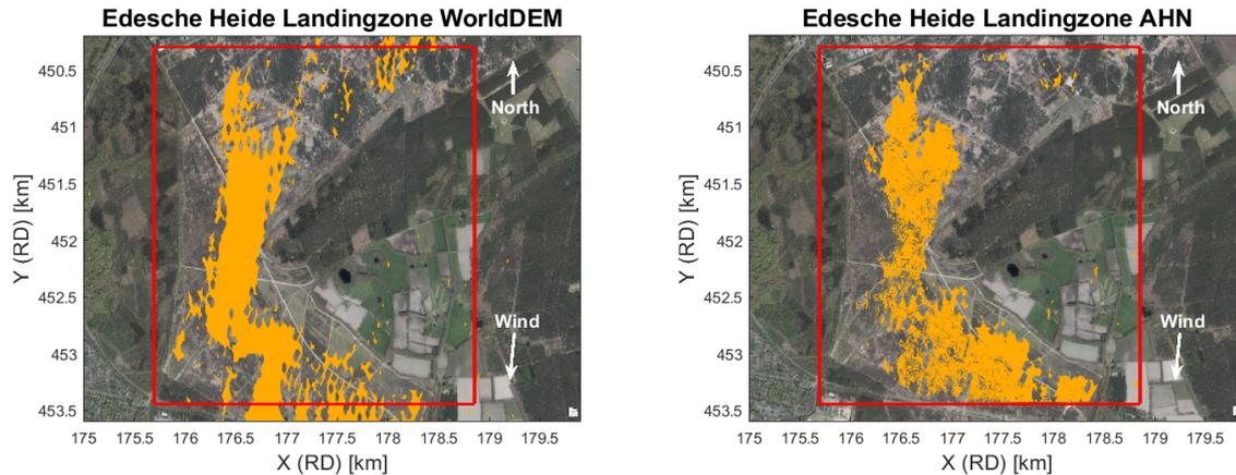
(a) The potential landing zones resulting from the new method with the input of the WorldDEM Digital Surface Model. (b) The potential landing zones resulting from the new method with the input of the AHN4 Digital Surface Model.
