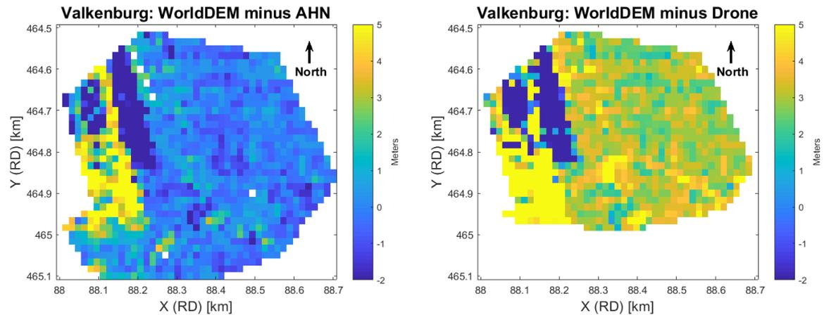
(a) The differences in height between the WorldDEM and AHN3 Digital Surface Model. The color bar is limited to the differences seen in the grass field. This way a more contrast rich figure is created.
