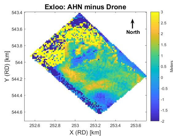
(c) Difference between the AHN2 Digital Surface Model and the Drone Digital Surface Model. The color bar is limited so a more detailed overview is created of the potential touch down area.
