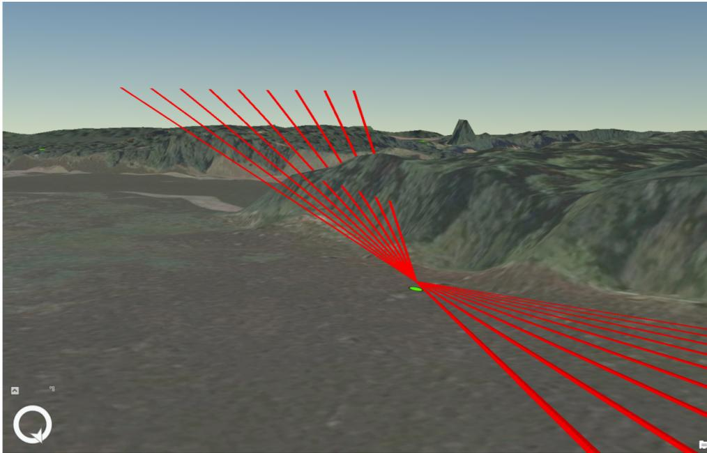
Figure 3.10: The sight lines are created 360 degrees around the observer point. The observer point is given in green. It is possible to select the sight lines according to the wind direction. A selection of the sight lines can be seen in red. Some sight lines are interrupted by the surroundings of the observer point. Only observer points with no interrupted sight lines are suitable regarding the shoot requirements.
