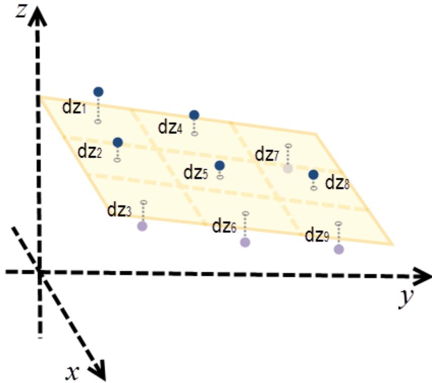
Figure 3.6: The 3x3 cell plane's best fit will be calculated using the least squares method [62]
