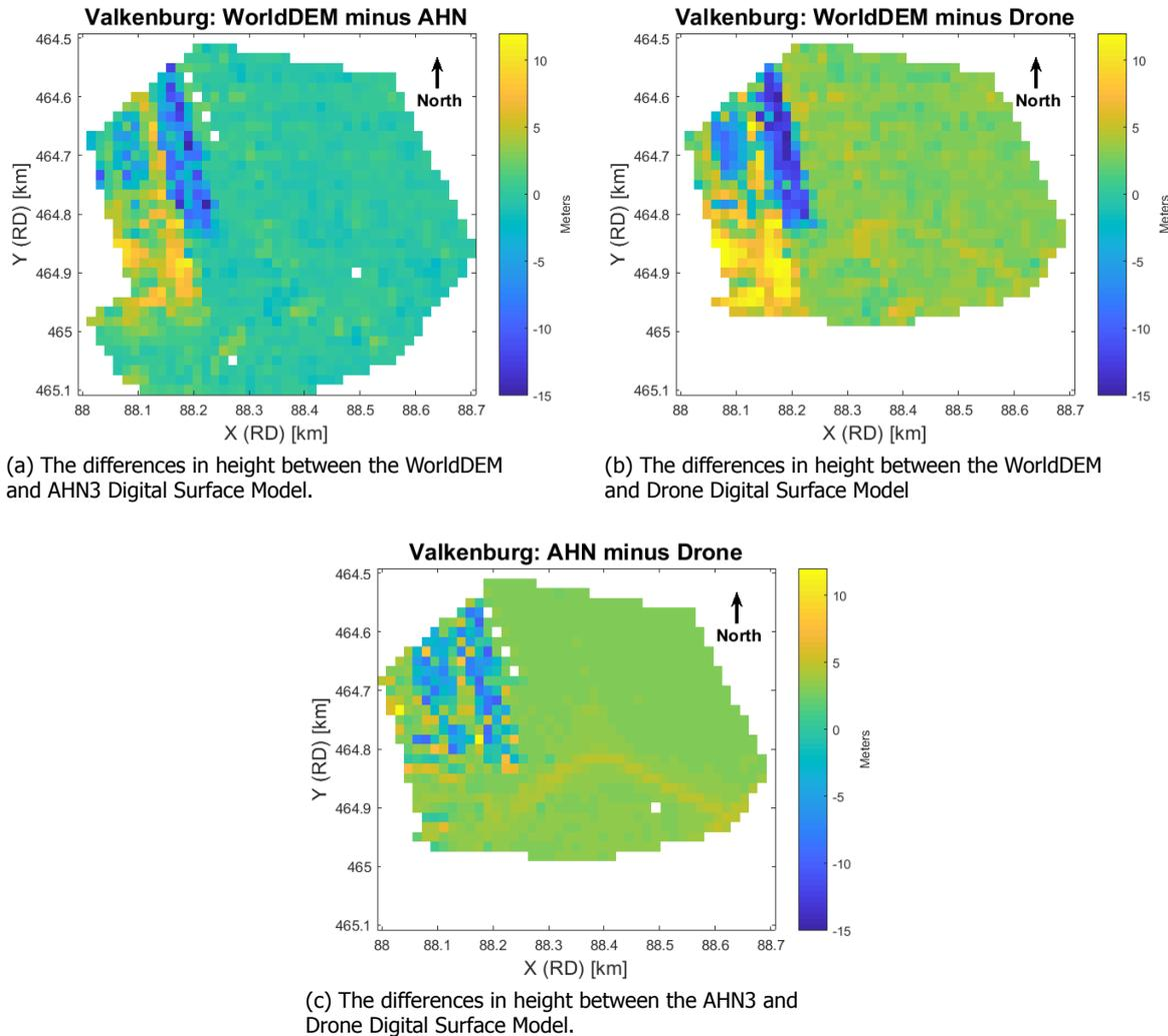
Figure 4.3: The differences between the three Digital Surface Models. The differences are given in meters. The largest differences, both positive and negative, occur at the location of the trees. The grass field and the concrete runways show relative low differences.
