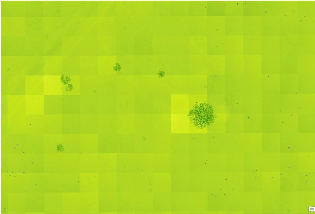
Figure 5.8: In this figure, the WorldDEM Digital Surface Model minus the AHN3 Digital Surface Model is visualized. The five darker green spots are freestanding trees. The darker the color green becomes the more negative the difference is. A negative difference means the AHN3 value is larger than the WorldDEM value.
