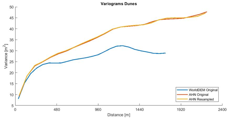
Figure 5.2: Variograms of the dune area in which the Pathfinders are interested. The empirical variograms of the WorldDEM, the original AHN3 and the resampled AHN3 Digital Surface Models are shown.
