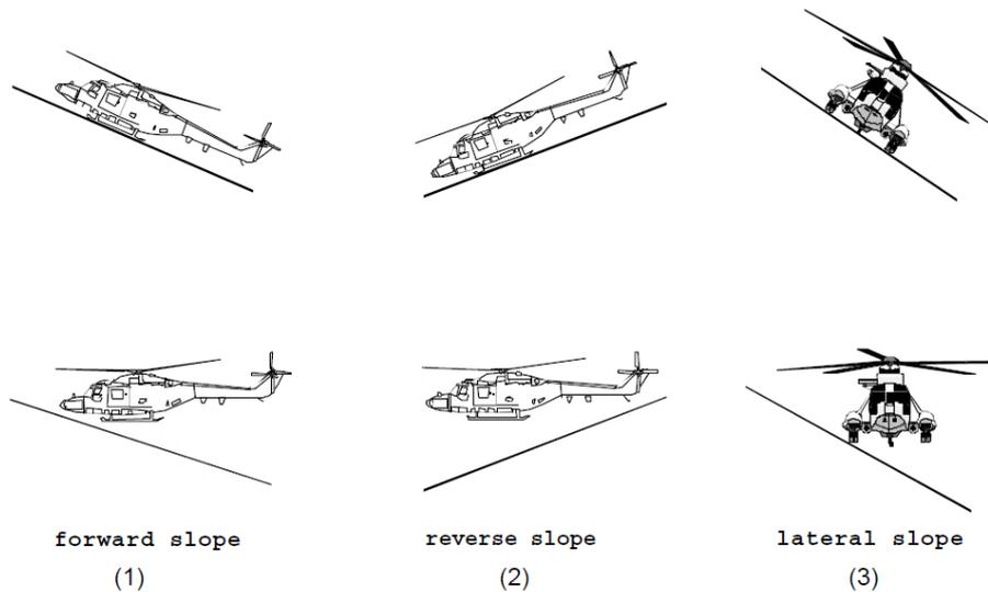
Figure 2.1: The different types of slope distinguished by the Dutch Military. The slopes are relative to the flying direction of the helicopter [4].
