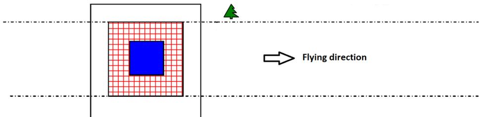
Figure 2.3: The search for obstacles is performed in the flying direction. This is done over the width of either the GCL or the FOO depending on the size of the landing point. In this figure landing point size 5 is displayed. Obstacles may be present outside of the strip, visualized by the dotted lines, like the tree in the image [4].
