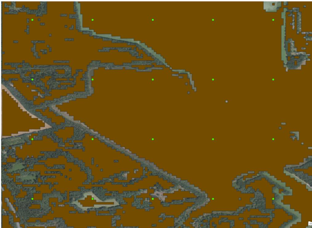
Figure 3.9: The area suitable regarding the slope and aspect requirements is given in brown. The green points are the observer points. The interval between the observer points can be adjusted.
