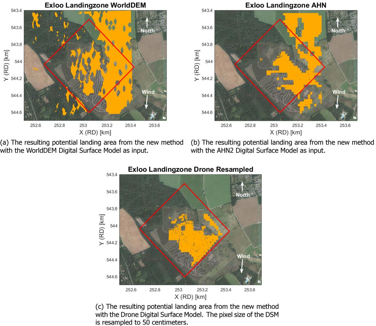
Figure 4.11: The resulting potential landing zones in orange for the Exloo case study. The area marked by the red square is the area available for all the Digital Surface Models. The wind direction is indicated by the arrow in the lower right corner.
