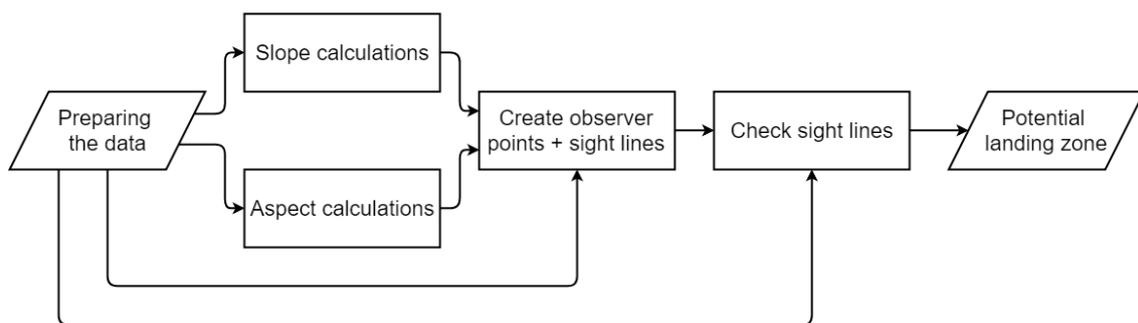
Figure 3.4: A flowchart of the steps taken to get from a DSM to a potential landing zone. First, the data is prepared. Then, the slope calculations and aspect calculations are performed. Next, the observer points and sight lines are created. Last, the sight lines are checked.
