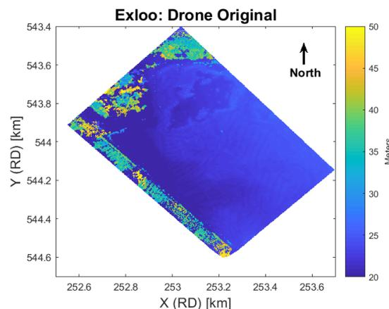
(c) Representation of the Drone Digital Surface Model of the heathland near Exloo
