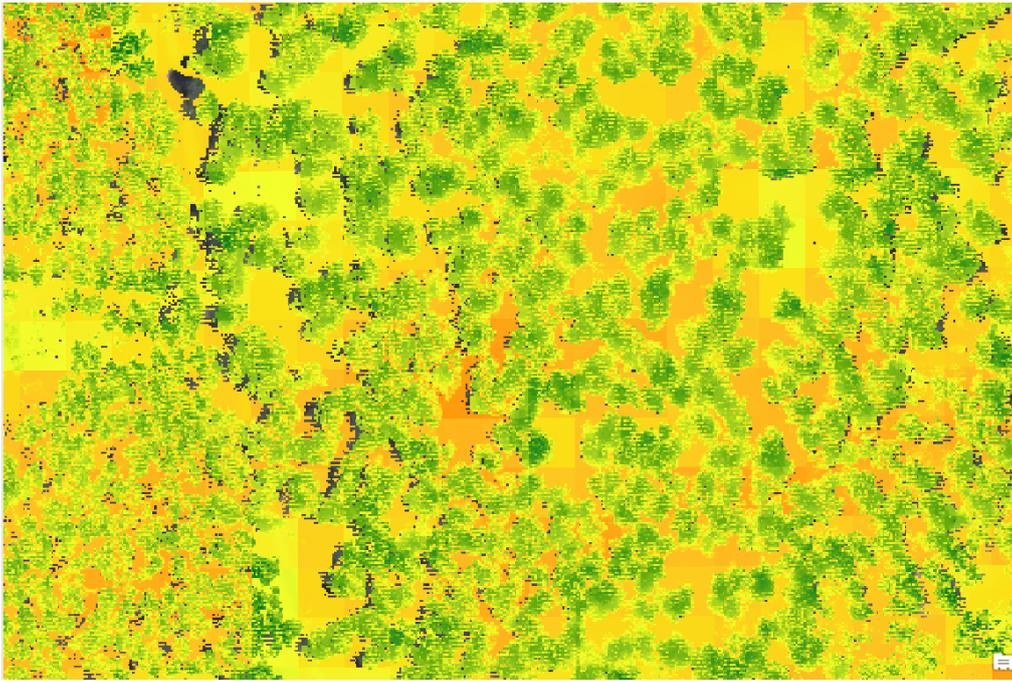
Figure 5.7: In this figure, the WorldDEM Digital Surface Model minus the AHN3 Digital Surface Model is given. The value of the crown of the trees in the AHN Digital Surface Model is higher than the value given by the WorldDEM. This is represented in the green colors. The areas between the trees are showing yellow and red colors. This is where the WorldDEM gives higher values than the AHN because of the averaging that happens due to the larger pixel size of the WorldDEM.
