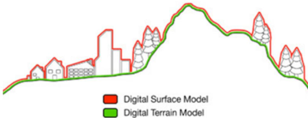
Figure 2.4: The term Digital Elevation Model (DEM) is both used for Digital Surface Model (DSM) and Digital Terrain Model (DTM). The difference between the two is whether objects on top of the ground level are taken into account [16].
