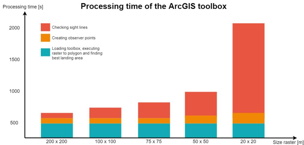
Figure 5.9: The processing time of the ArcGIS toolbox for different observer point raster sizes. The trend seen in raster size 200x200 meter to 50x50 meter is not representative for the processing time of the 20x20 meter.
