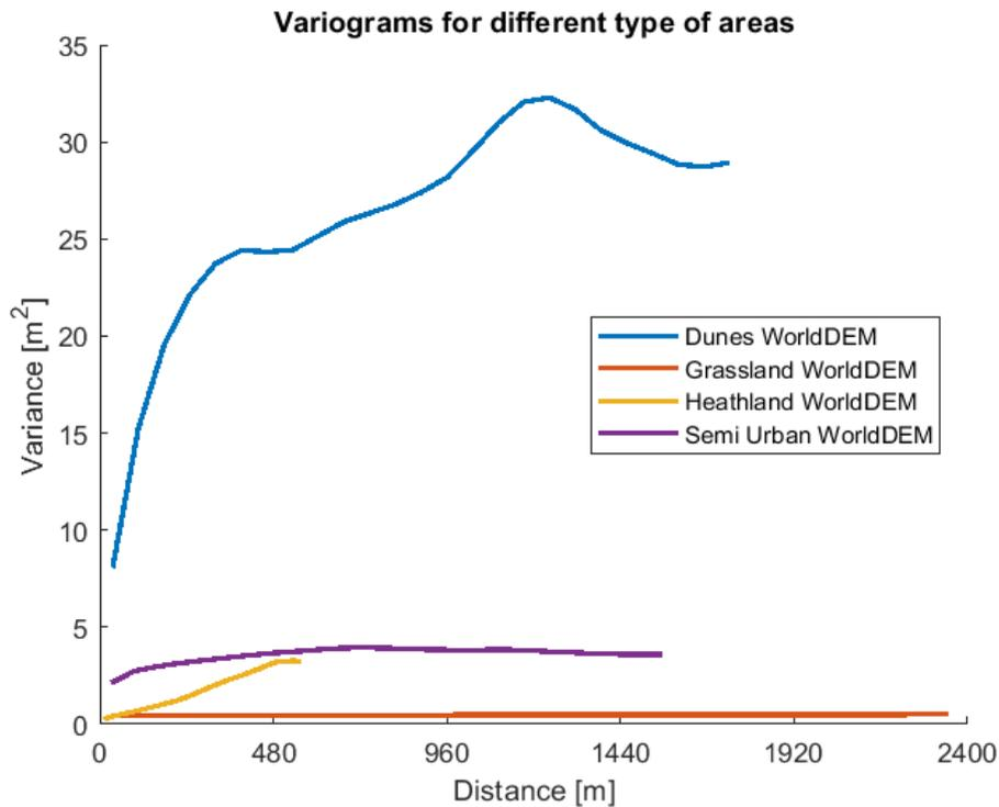
Figure 5.1: Variograms of the different types of areas in which the Pathfinders are interested. For all the variograms the WorldDEM Digital Surface Model is used. Not all variograms have to same length due to different size of the area type.
