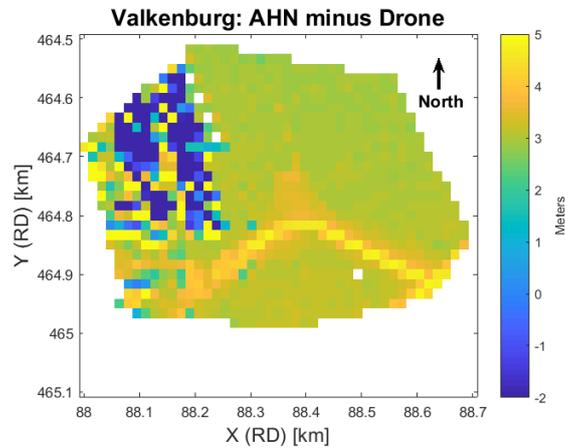
(c) The differences in height between the AHN3 and Drone Digital Surface Model. The color bar is limited to the differences seen in the grass field. This way a more contrast rich figure is created.
