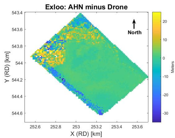
(c) Difference between the AHN2 Digital Surface Model and the Drone Digital Surface Model.
