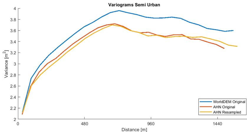
Figure 5.5: Variograms of the semi-urban area in which the Pathfinders are interested. The empirical variograms of the WorldDEM, the original AHN3 and the resampled AHN3 Digital Surface Models are shown.
