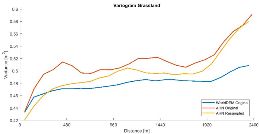
Figure 5.3: Variograms of the grassland area in which the Pathfinders are interested. The empirical variograms of the WorldDEM, the original AHN3 and the resampled AHN3 Digital Surface Models are shown.
