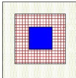
Figure 2.2: An example of a landing point. The area is divided in three parts. In blue the 'Hard Surface', in striped red the 'Cleared to Ground Level' and in dotted green the 'Free of Obstructions' [4].
