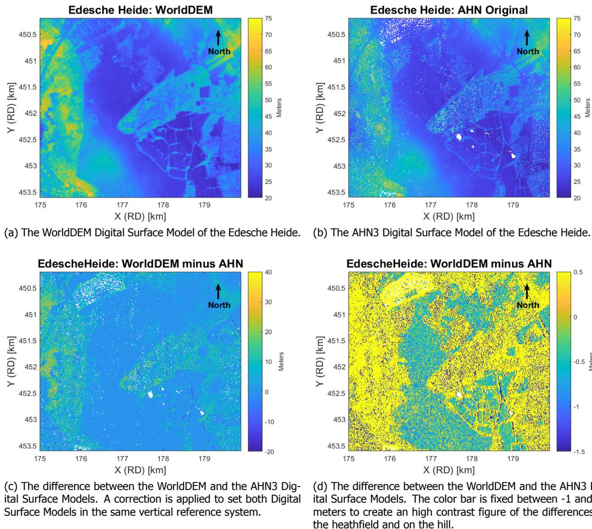
Figure 4.13: The original Digital Surface Models together with the difference between the Digital Surface Models. Two figures with the differences are included. One with the full range of differences and one with a limited range to be able to see the differences at the heathland in detail.
