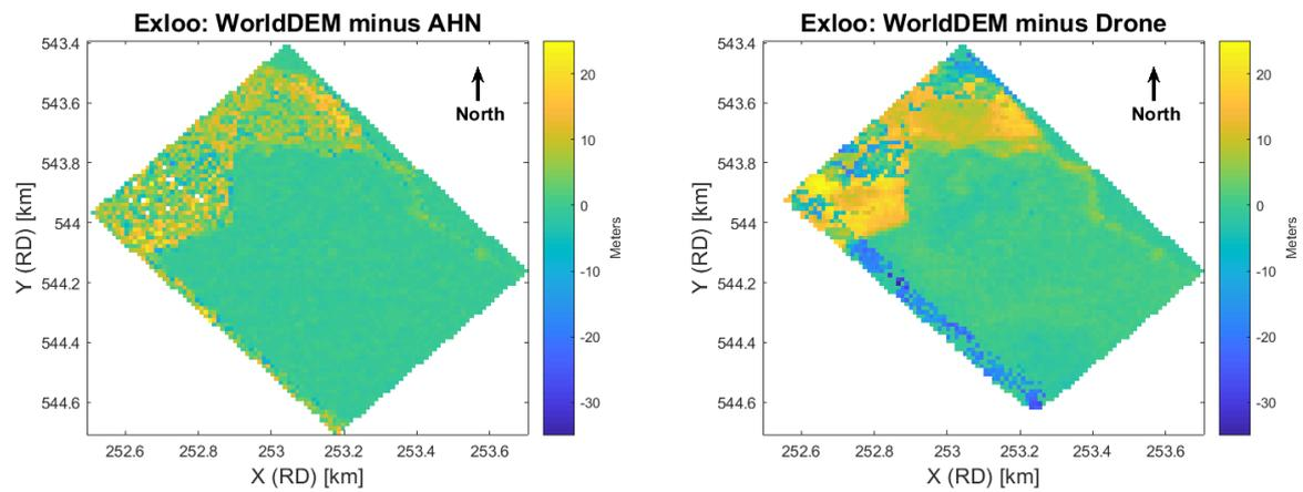
(a) Difference between the WorldDEM Digital Surface Model and the AHN2 Digital Surface Model.
