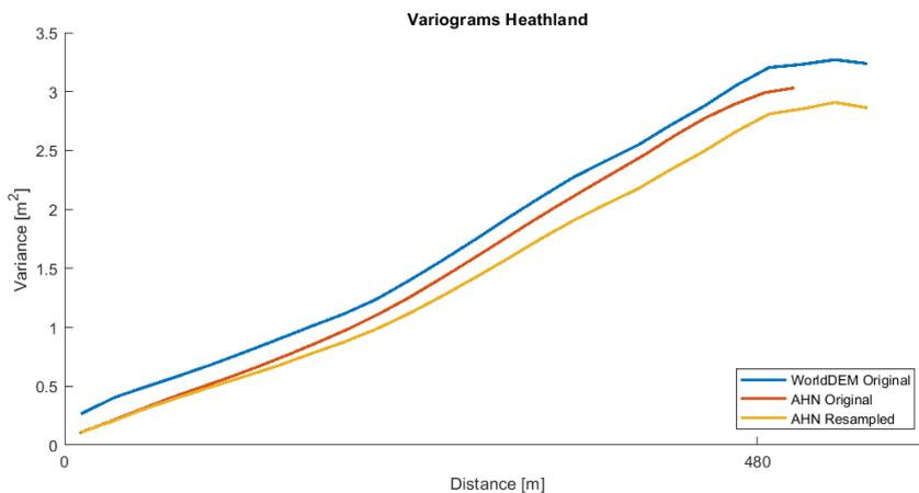
Figure 5.4: Variograms of the heathland area in which the Pathfinders are interested. The empirical variograms of the WorldDEM, the original AHN2 and the resampled AHN2 Digital Surface Models are shown.
