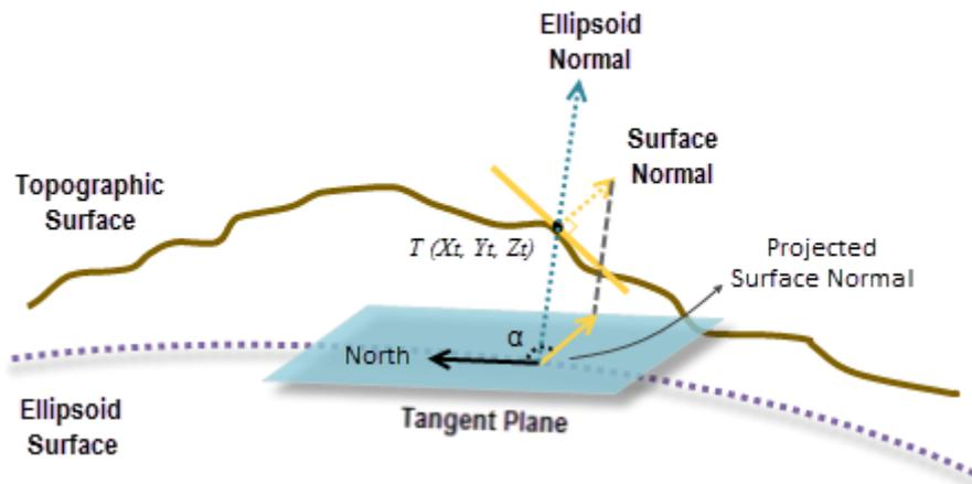
Figure 3.7: The computation of the aspect using the geodesic method visualized [63].
