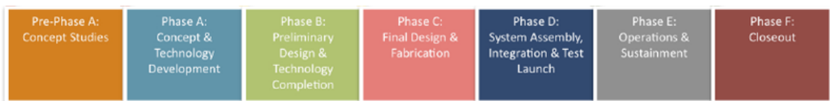
Figure 2.1: The space mission project life cycle from NASA. Adapted from https://ntrs.nasa.gov/
