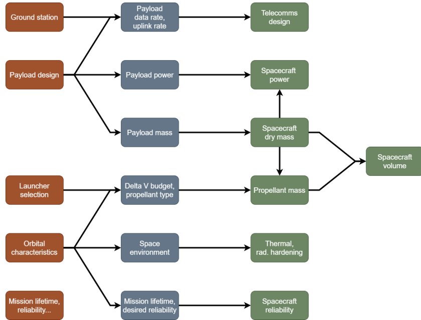
Figure 3.2: A graph visualizing the first-order system characteristics estimation process, for utilization in Valispace.
