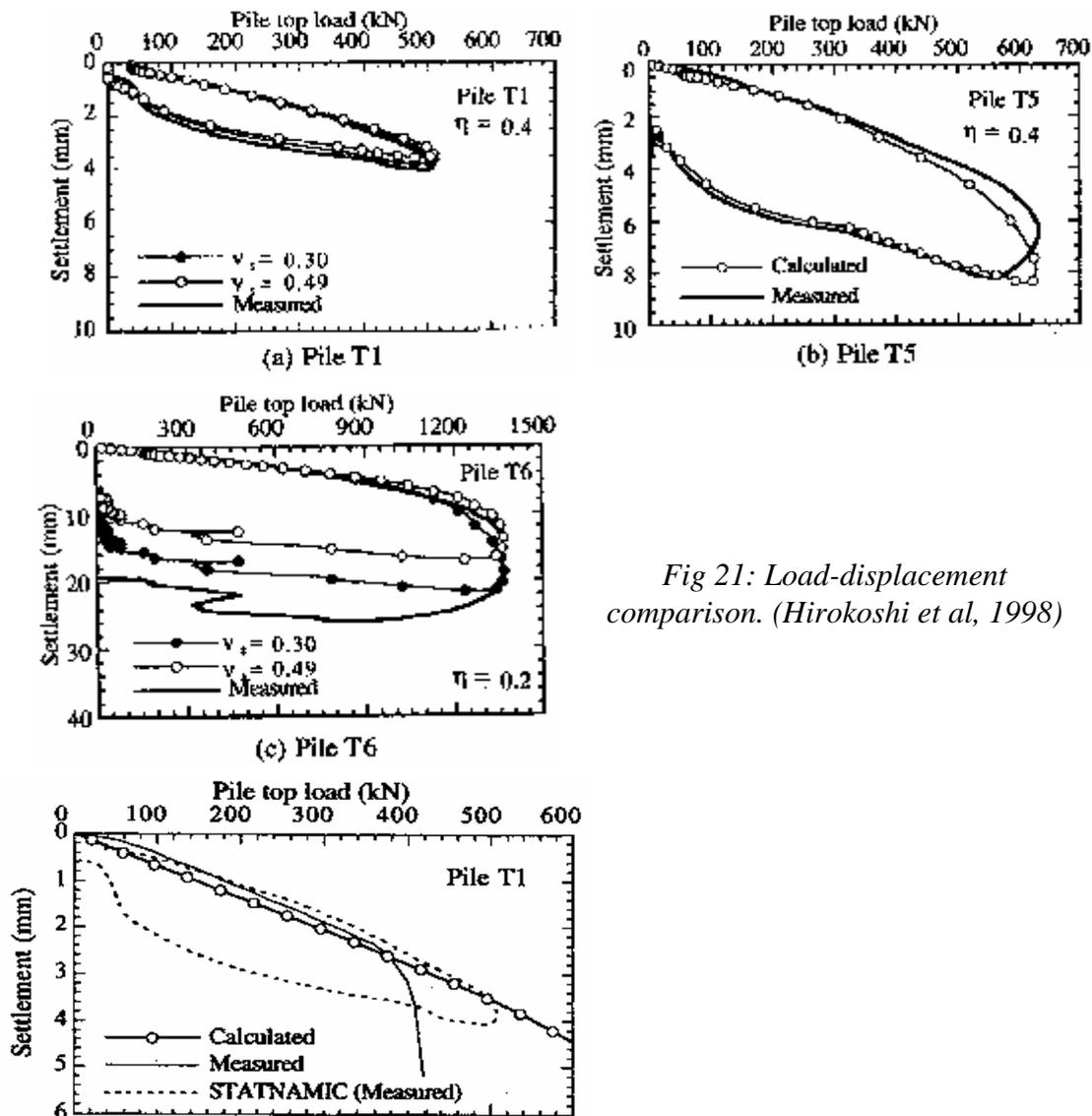
Fig 21: Load-displacement comparison. (Hirokoshi et al, 1998)
