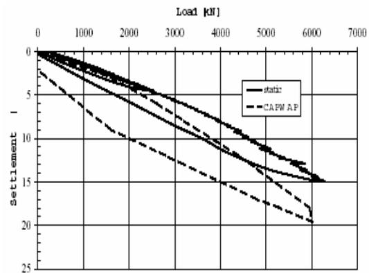
Fig 31: Typical load-displacement of concrete pile (Kirsch et al, 2000).
