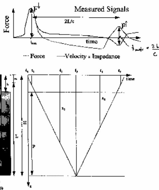
Figure 26: Quantities definition in signal processing method (van Foeken et al, 1996).
