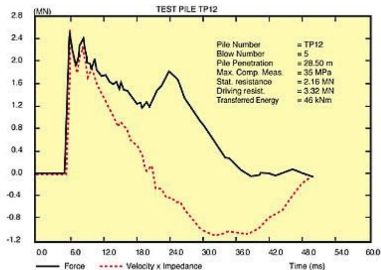
Figure 24: Typical PDA measured signal.
