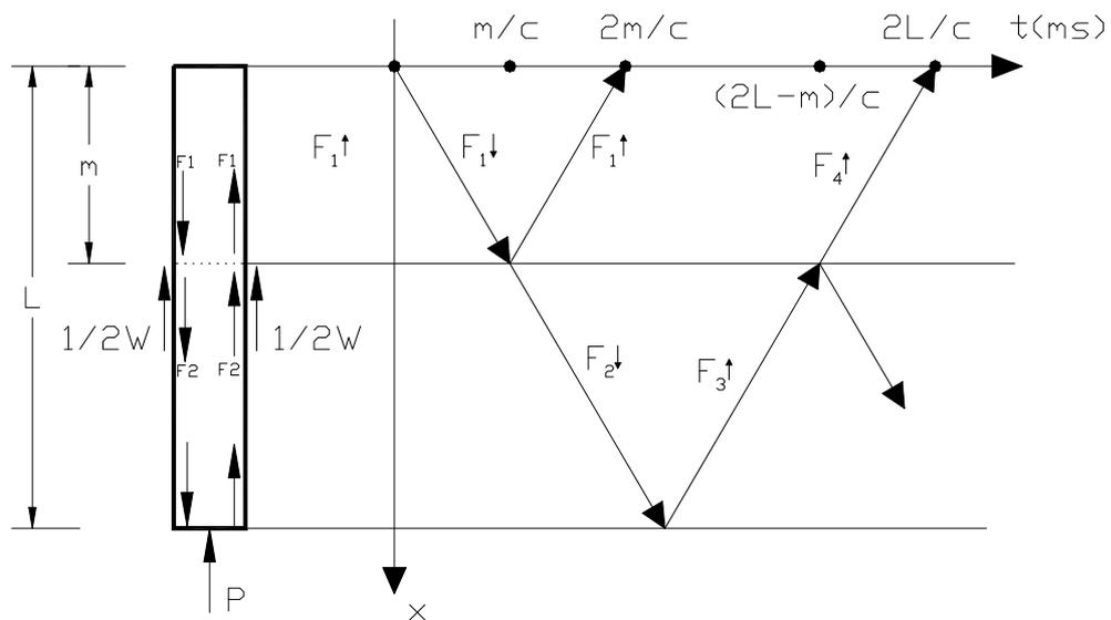
Figure 42: One wave propagation cycle in pile
