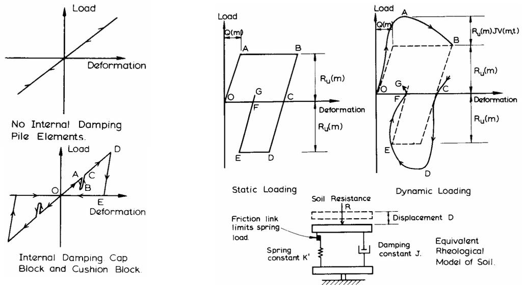
Figure 28: Load-deformation characteristics for pile and soil. (A.E.L. Smith – 1960)
