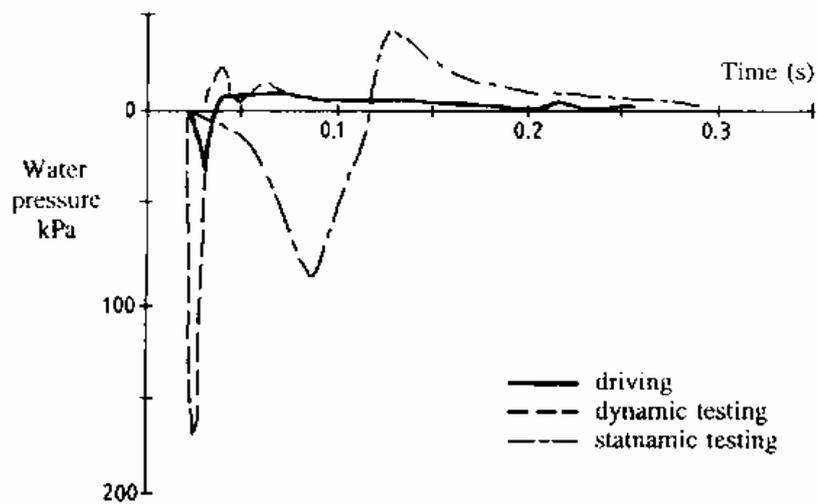
Figure 35: Pore pressure during pile driving, dynamic and quasi-static tests (Holscher, 1992).
