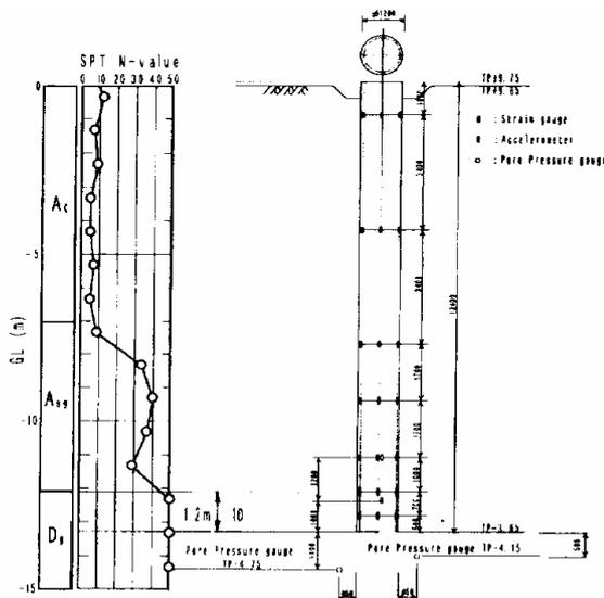
Fig. 12: Test pile and positions of measurement (Meada et al, 1998).
