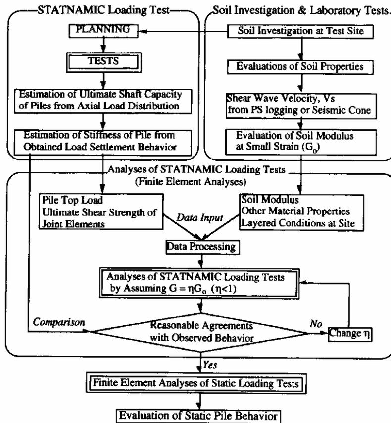
Fig 9: The finite element analytical sequence (Horikoshi et al, 1998).
