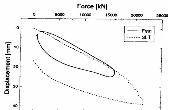
Fig. 13: Load-displacement relation (Meada et al, 1998).
