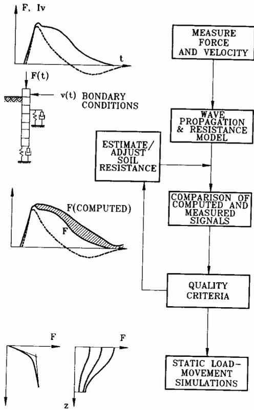
Figure 26: Numerical analysis procedure (A.E. Holeyman, 1992).
