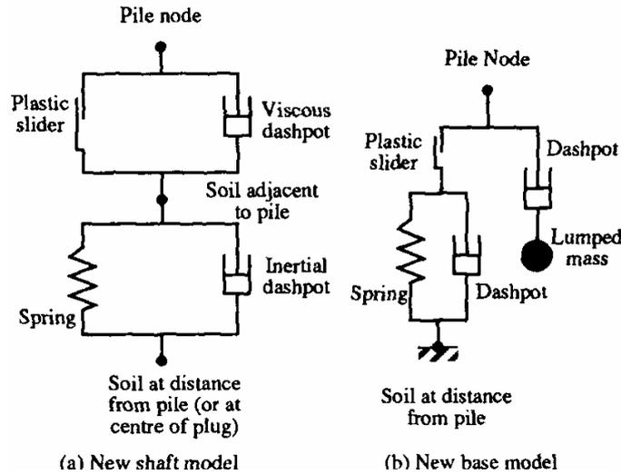
Figure 29: New shaft and base soil model.
