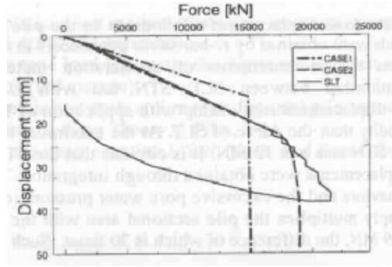
Fig. 17: Comparison between SMA and SLT (Meada et al, 1998).
