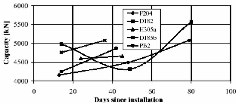
Figure 32: Set-up of the driven cast-in-place piles.
