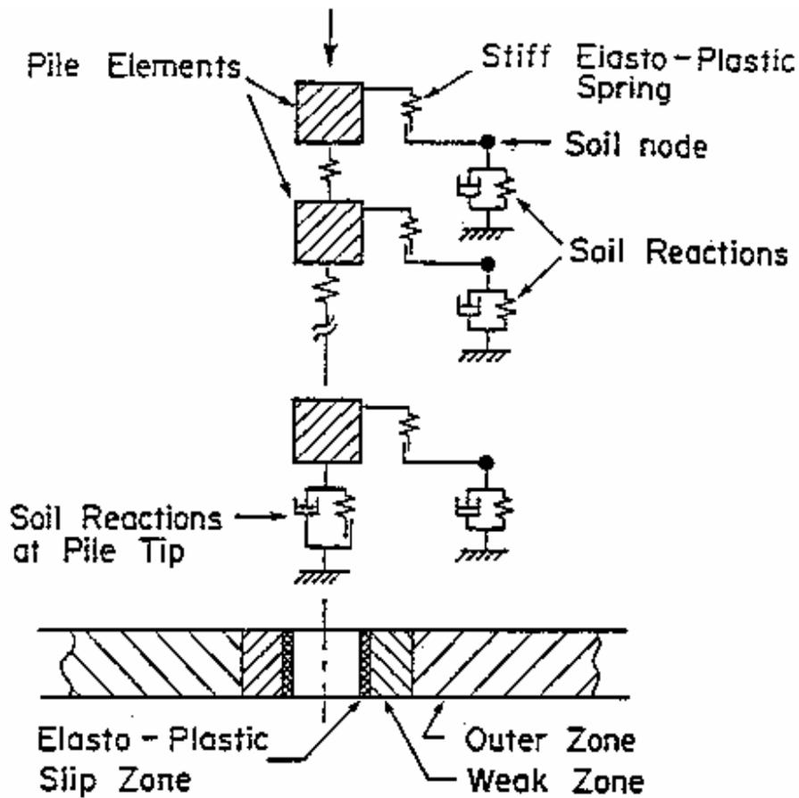
Figure 7: Pile – soil model (El.Naggar et al - 1992).
