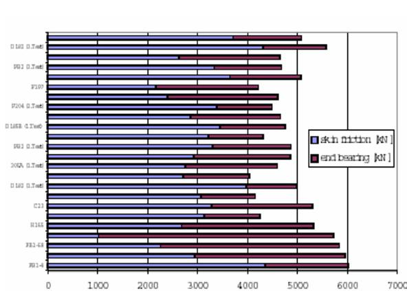
Fig 30: CAPWAP results of pile capacities. (Kirsch et al, 2000)
