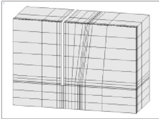
Fig. 33: 3D FE mesh for pile D182 with adjacent trench (Kirsch et al, 2000).
