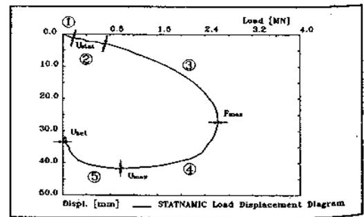
Fig 5: Force action on the pile and load-displacement diagram (P.Middendorp et al, 1992).
