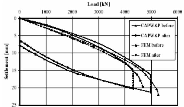
Fig. 34: Load-displacement curves of pile D182 (Kirsch et al, 2000).
