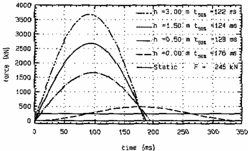
Figure 2: The force as a function of time for different drop heights. (Schellingerhout *et al*. 1996)
