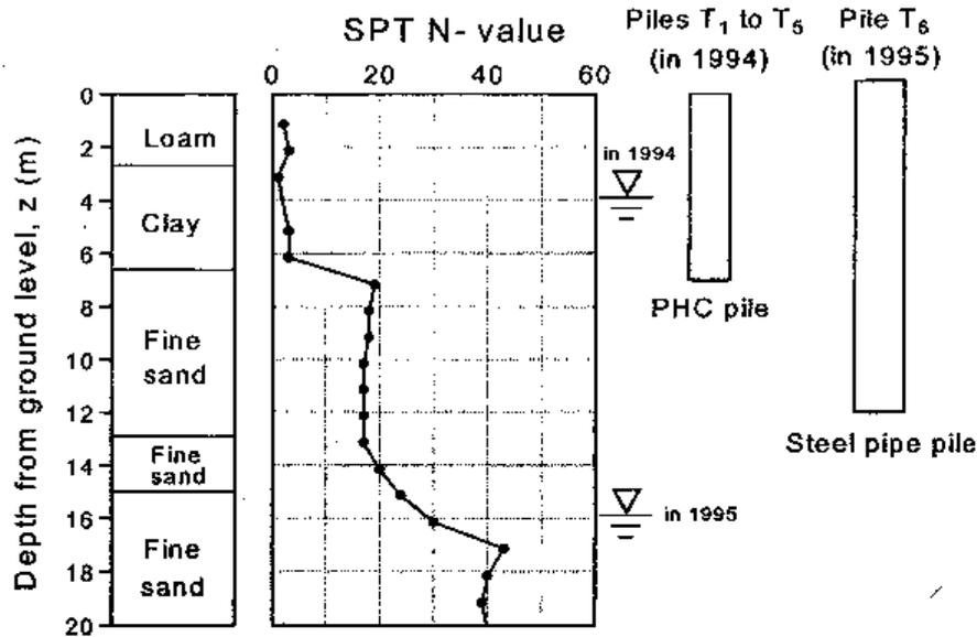
Fig 19: Soil profiles in Shonan test site (Hirokoshi et al, 1998).
