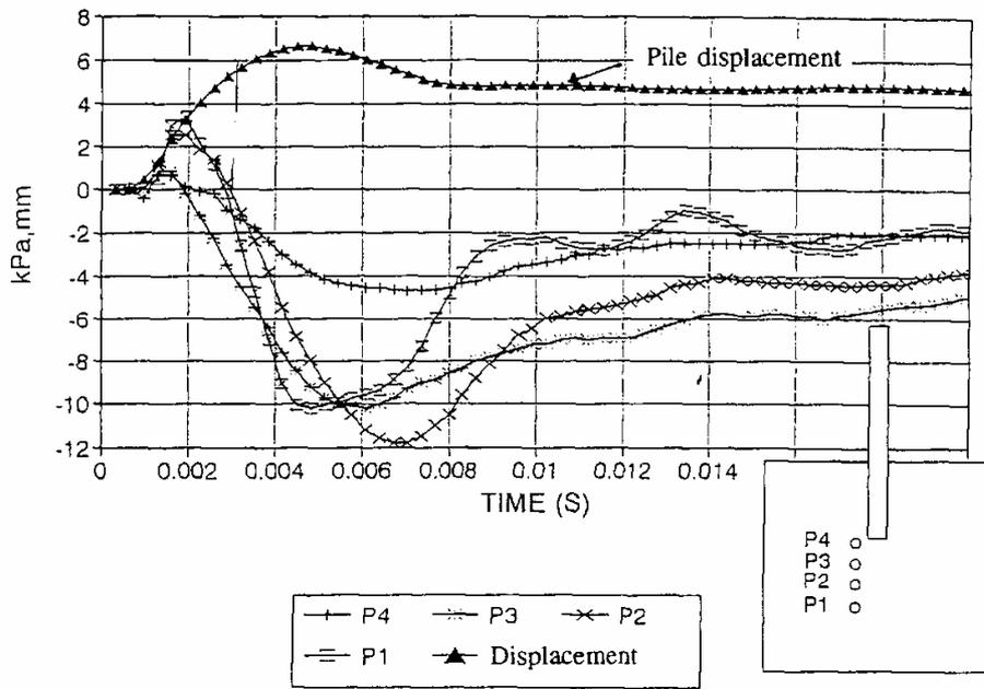
Figure 36: Typical pore pressure in Ottawa sand, 0,8m height (Eiksund et al. 1996).
