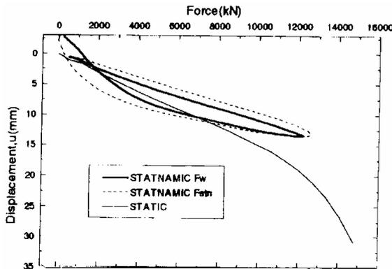
Fig. 16: Load-displacement comparison for SMA and SLT (Meada et al, 1998).
