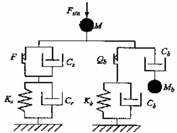
Fig 6: A new single mass model for static test (K.Kato et al, 1998)
