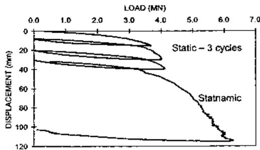
Fig 10: Static and STATNAMIC derived static load-displacement.
