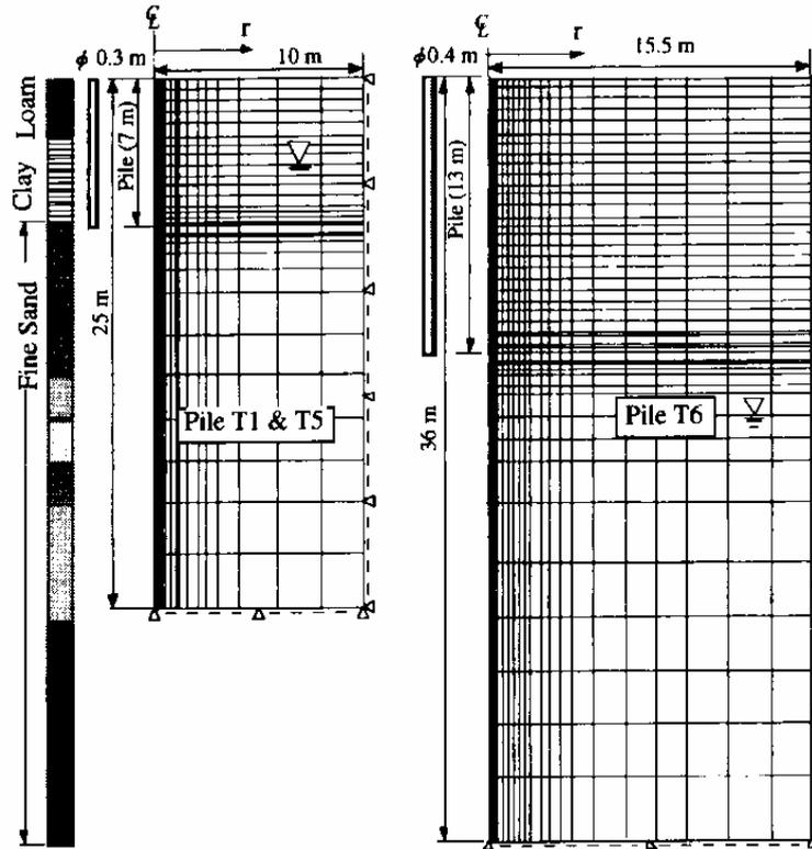
Fig 8: Finite element model (Horikoshi et al, 1998).
