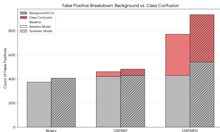
Figure 4.3: Breakdown of FP by error type across label setups. Background Error refers to non-litter objects detected as litter, while Class Confusion refers to correctly detected litter assigned the wrong material label. Hatched bars indicate models trained with synthetic data.
