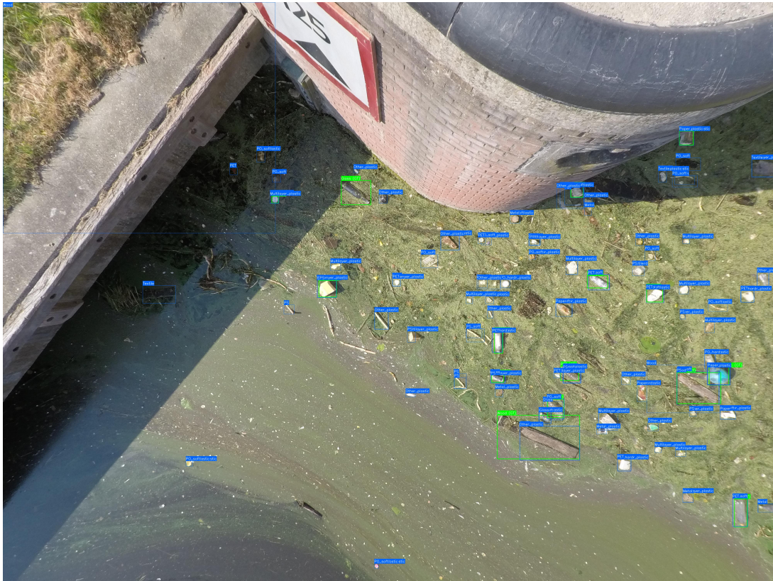
Figure 5.2: Example of "missing labels" in the RPD dataset (Amsterdam). The model's predictions (blue boxes) correctly identify numerous litter items that are missing from the ground truth (green boxes).
