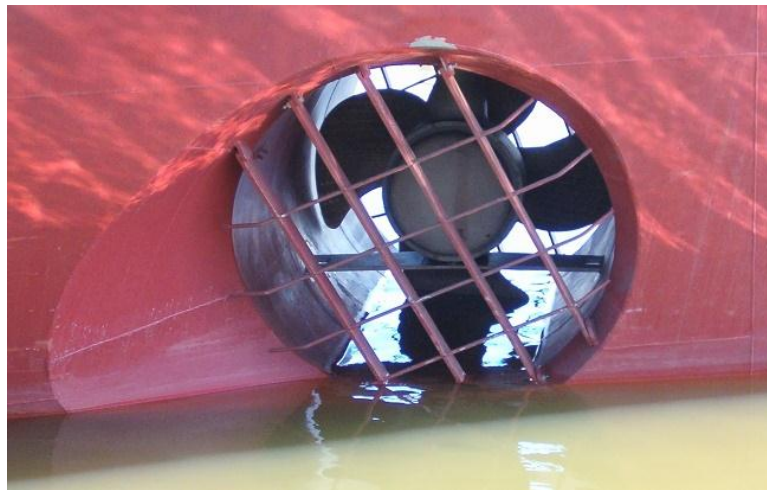
Figure 1.1 Bow tunnel thruster with protection grid. Picture adapted from [4].
