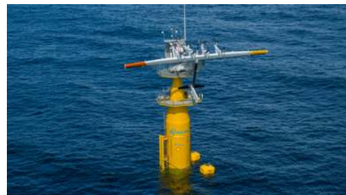
The Makani energy kite rests on its base station atop a floating platform during Makani's first offshore test campaign. August 2019.
