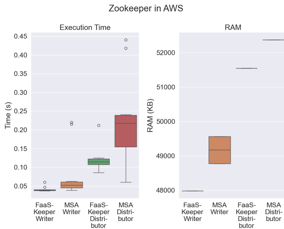
Figure 6.13: Execution time and RAM usage of Writer and Distributor in ZooKeeper
