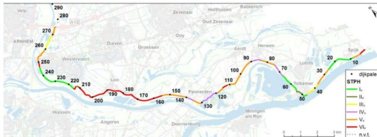
Figure 5.2: Assessment of the failure mechanism piping (STPH) of trajectory 48-1 (WRIJ, 2019)
