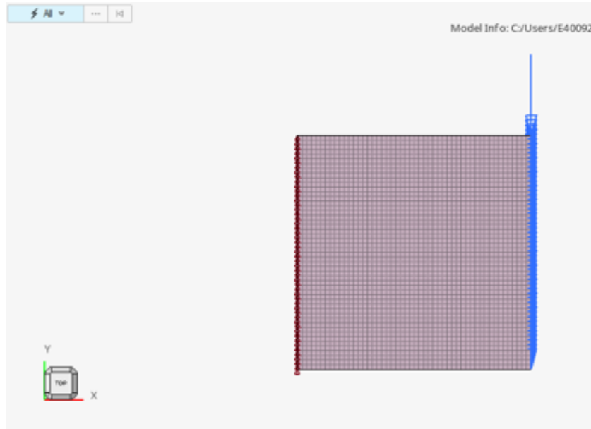
Figure 4.2: Altair Hyperworks model of cantilever plate
