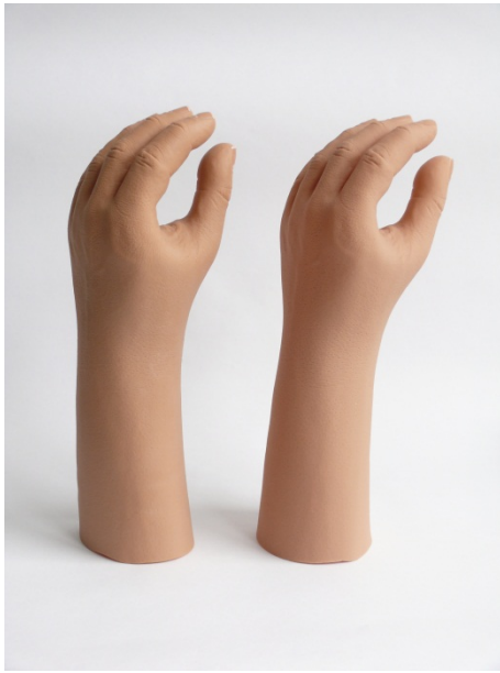
Figure 4 The RSLSteeper cosmetic gloves that were used in this study, the PVC glove (left) and the silicone glove (right).
