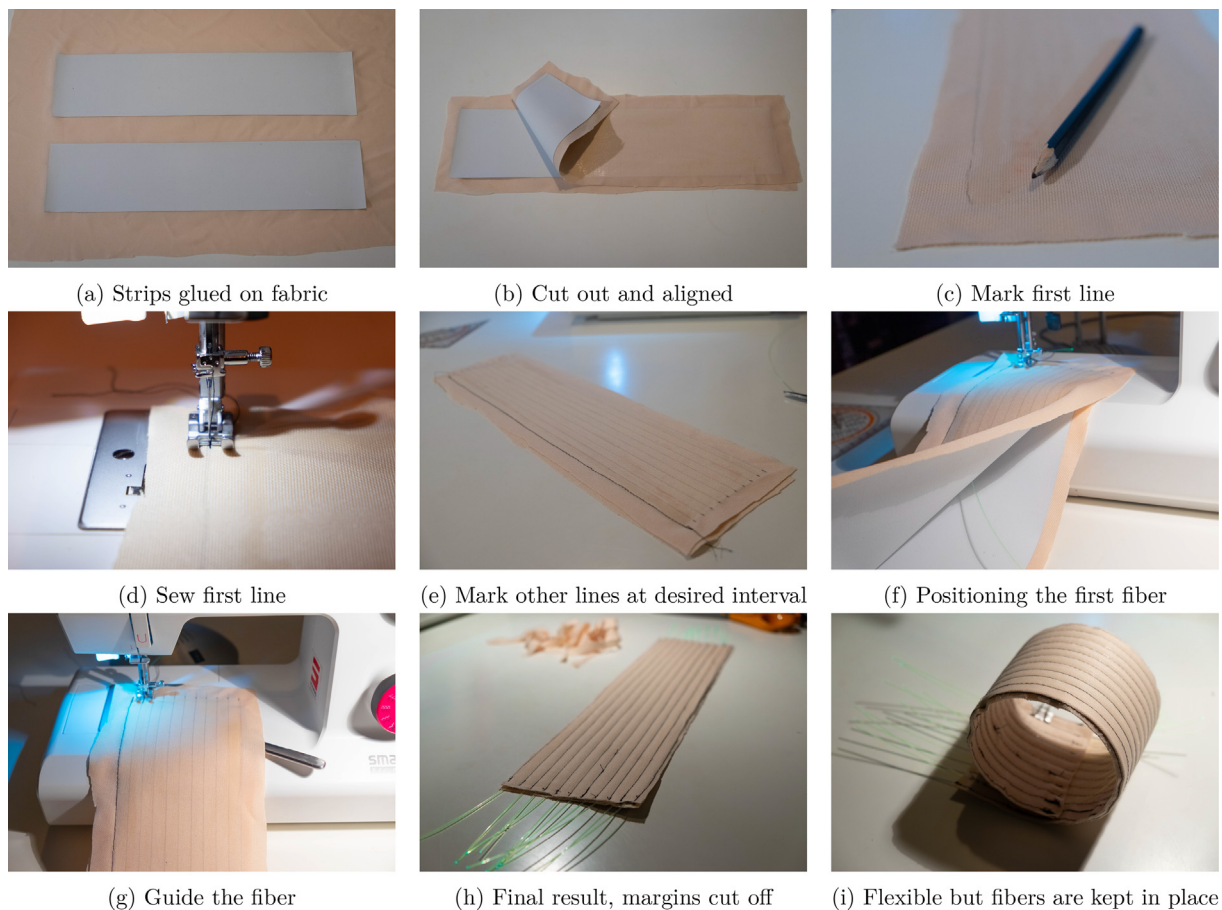
Fig. 4. Ribbon-detector Fabrication.
