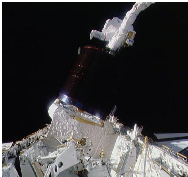
Figure 3.3: Westar VI being berthed in the cargo bay of Discovery using the Orbiter's robotic arm [16].
