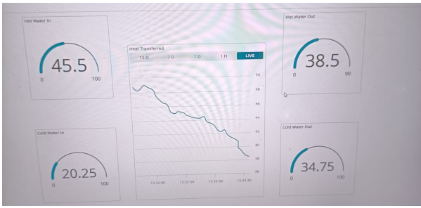
Fig. 9. Arduino IOT online portal overview. Left above indicates T_{\text{Dirty\_in}} , right above indicates T_{\text{Dirty\_out}} , left bottom indicates T_{\text{Clean\_in}} and right bottom indicates T_{\text{Clean\_out}} .
