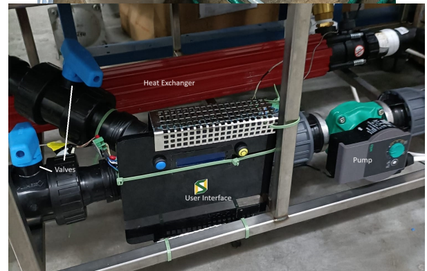
Fig. 8. Overview of the setup for the experiment at the GreenCycl Living lab facility. Underneath a close up of the valves (blue), the heat exchanger (red), the pump (green) and the display of user interface (with blue and yellow buttons).
