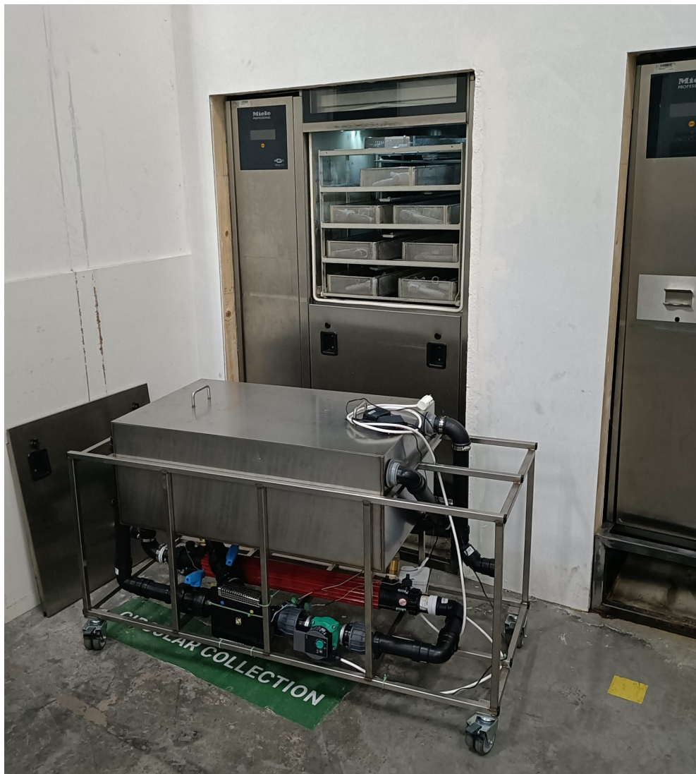
Fig. 13. The final prototype located in front of one of the Miele washer-disinfection machines. In the prototype, green indicates the pump, blue indicates the valves, red indicates the heat exchanger.
