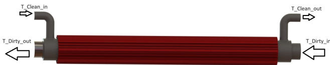
Fig. 7. K-type thermocouple sensor location used to determine the amount of heat being transferred between the mediums.
