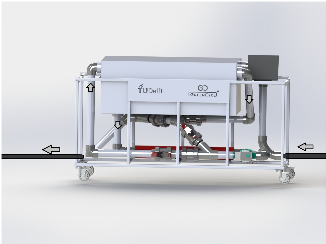
Fig. 10. Final Solidworks design of the mobile GreenCycl effluent heat retracting system. The arrows indicate the flow of the dirty water. The water is collected in the tank and flow through the pipes into the STHEX due to the force exhibited by the pump. The water reaches a 45 degree T-split and either passes straight back into the tank or lead outside the system into the drainage.
