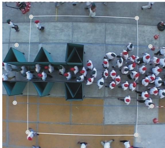
**Figure 4.3:** Example of the narrow bottleneck experiment
