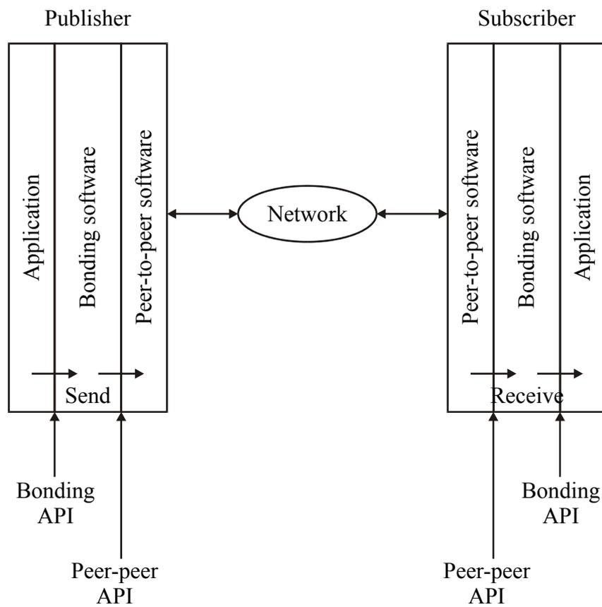
**Figure 7.5:** Overview of the communication between distributed applications (Boar 1993)
