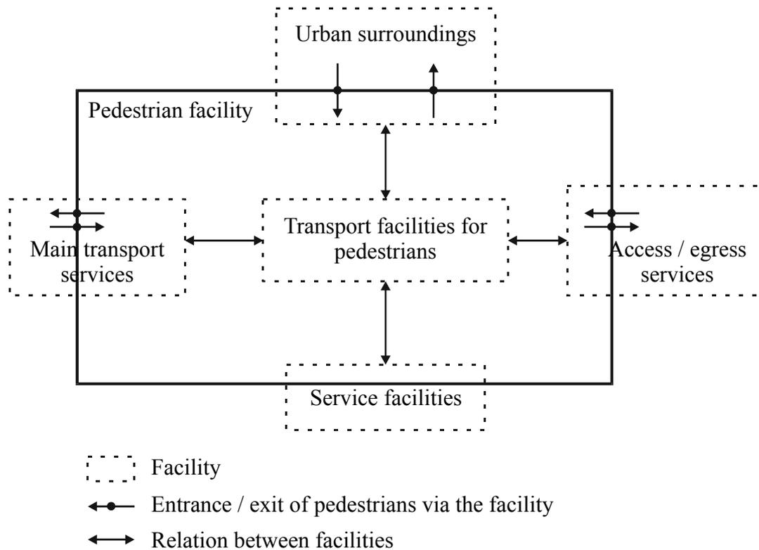
**Figure 5.4:** Generic functional decomposition of a pedestrian facility
