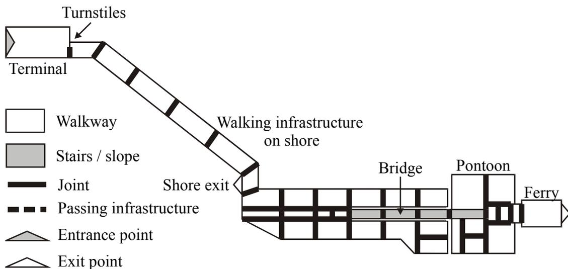
**Figure 9.14:** Infrastructure of Breskens: the terminal, the infrastructure on shore, the bridge, the pontoon, and the ferry
