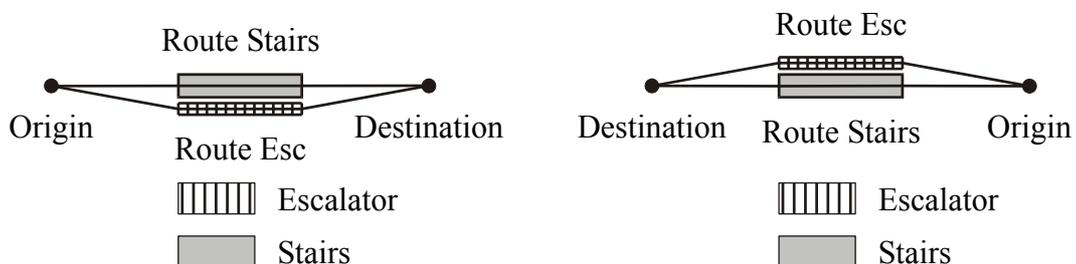
**Figure 8.5:** Route choice set between the platform and the concourse (left) and vice versa (right)
