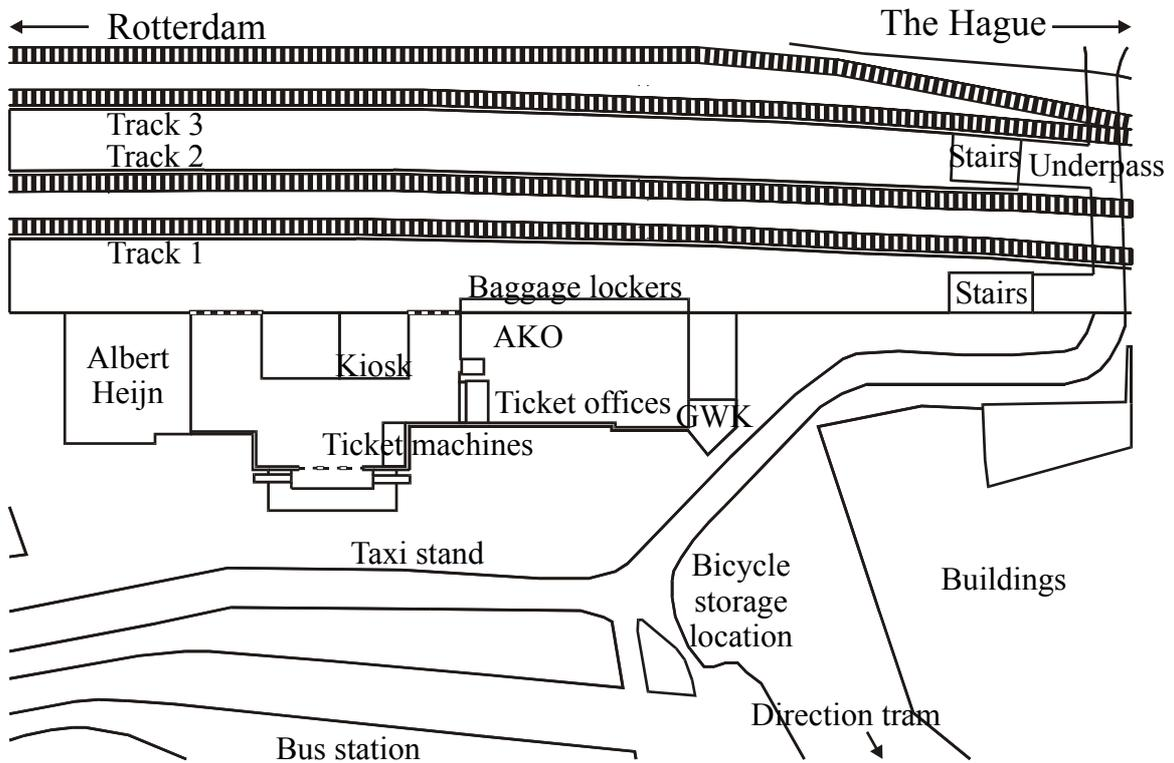
Figure E.2: Rail and pedestrian infrastructure at Delft Station
