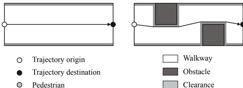
**Figure 5.12:** Examples of pedestrian trajectories around obstacles
