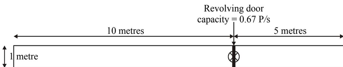
**Figure D.4:** Infrastructure for scenario 3: forming, stationary, and dissipating congestion
