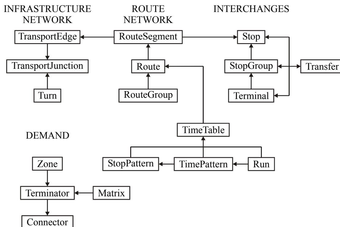
**Figure 7.2:** Object model for Transportation Object Platform (Nielsen et al. 2001)
