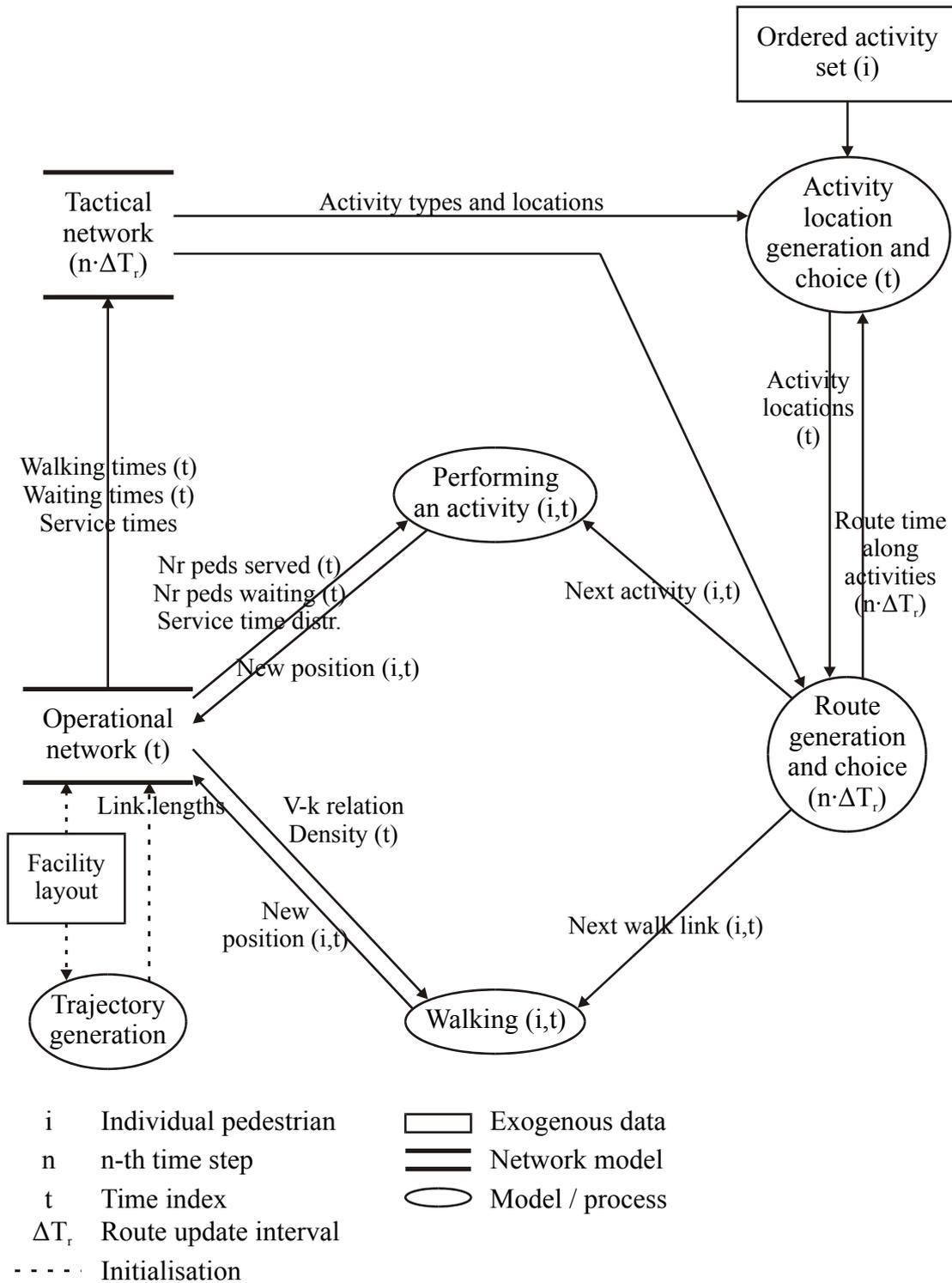
**Figure 6.1:** Overview of models and their interrelationships constituting the pedestrian flow simulation tool
