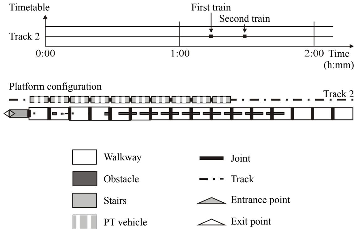
**Figure 8.6:** Overview of the configuration of Delft Station as input for the simulation tool
