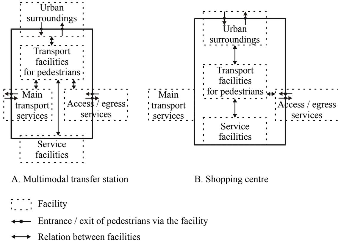
**Figure 5.5:** Functional decomposition of a multimodal transfer station and a shopping centre
