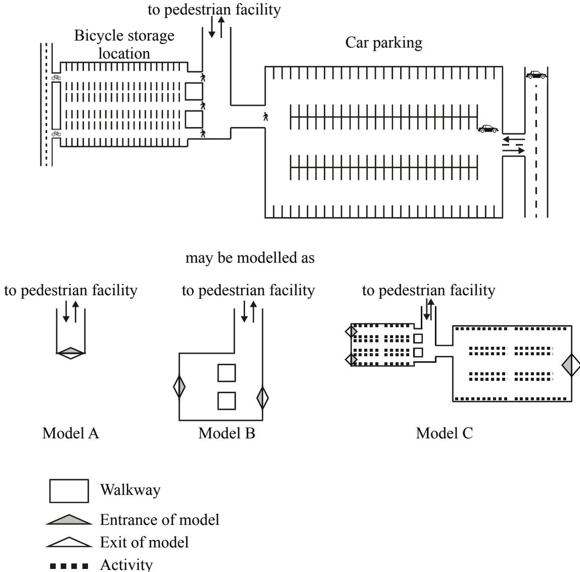
**Figure 5.7:** Different levels of spatial specification of a bicycle storage location
