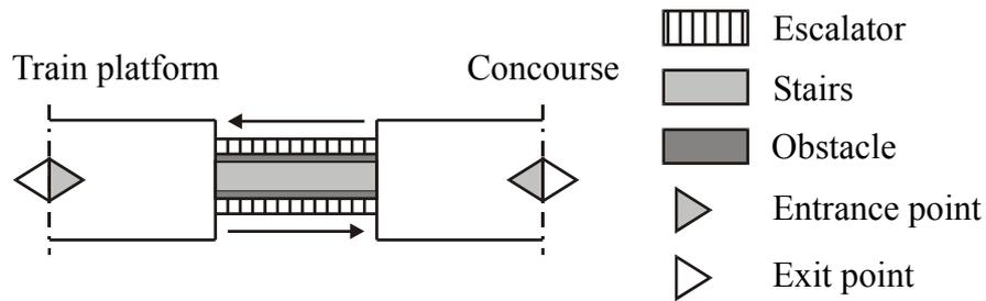
**Figure 8.4:** Infrastructure configuration for the validation of the route choice model
