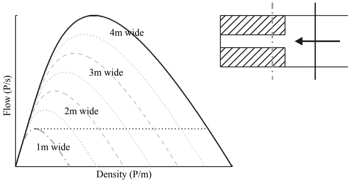
**Figure 4.12:** Traffic flow theory for pedestrian traffic
