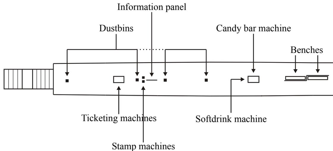
Figure E.4: Obstacles on platform 2 in Delft Station
