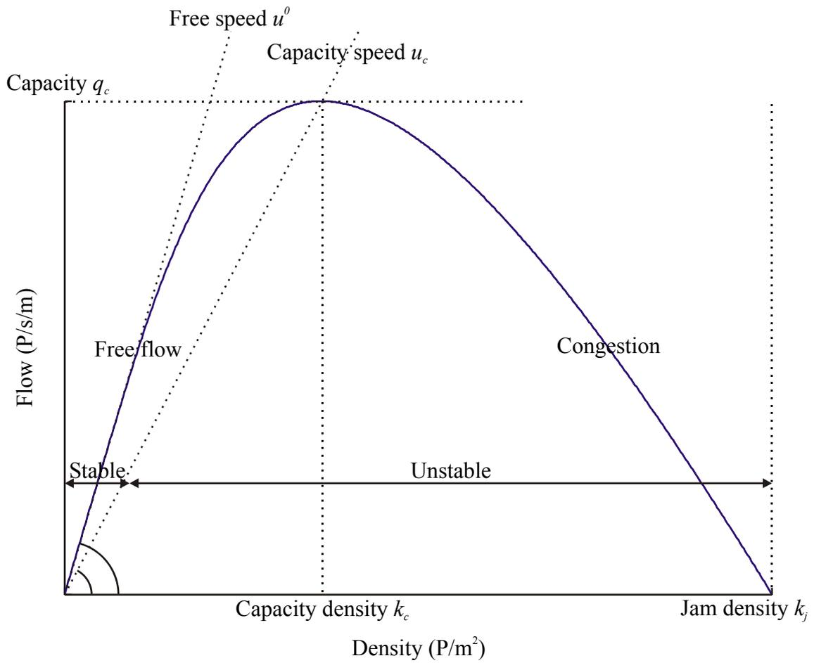
**Figure 3.4:** Flow-density relation for pedestrian traffic
