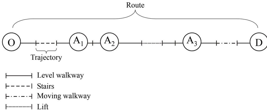
**Figure 5.11:** A route from origin to destination, consisting of activity locations and trajectories
