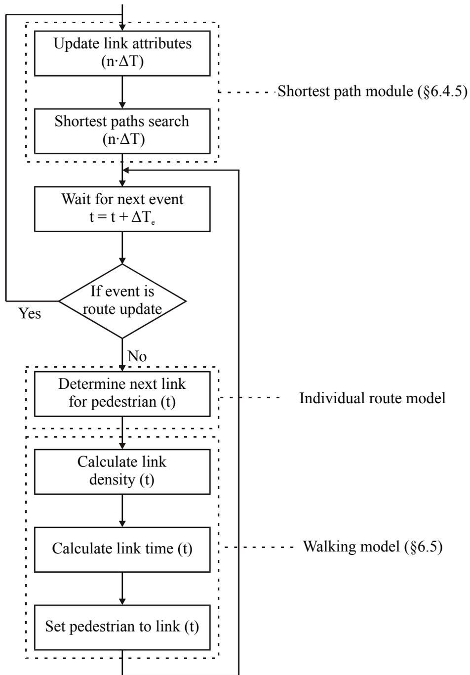
**Figure 6.17:** Flow diagram of the route choice model
