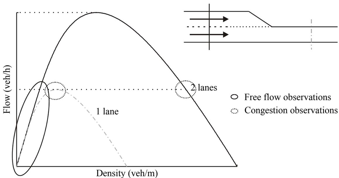
**Figure 4.11:** Traffic flow theory for car traffic
