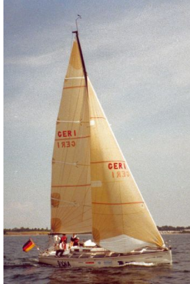
Figure 2.3: The Berlin Sail-Force Dynamometer DYNA while acquiring full-scale data under sails
