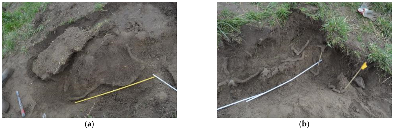
Figure 10. (a,b) Examples of excavated grouted animal burrows.
