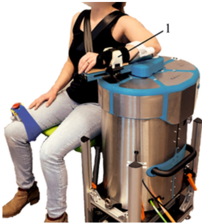
Fig. 1: A participant seated in the SEP with the forearm securely fixated with a clamp (1) and the shoulder abducted to 80°. The participant is strapped into the chair, and an emergency button is placed on the upper leg for safety [14].
