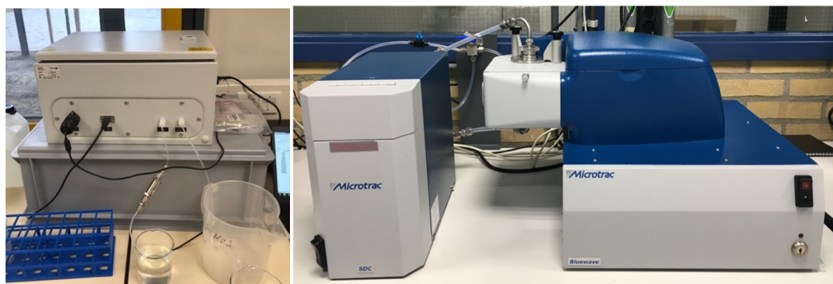
Figure 18: The PAMAS OLS4031 particle counter (left), and the BlueWAVE particle size analyzer (right, from Goess-Enzenberg, 2020) of the WaterLab
