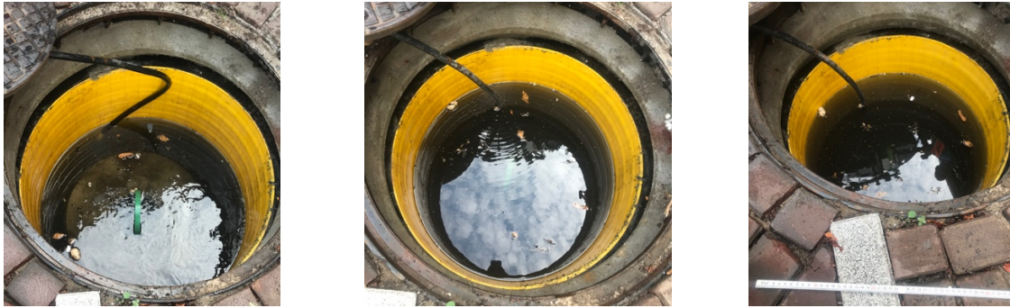
Figure D - 4: Darkening of water as solids are resuspended in the end shaft during pumping. Visible change in water level and colour shown at 10:20 am (left), 10:27 am (middle) and 10:30 am (right).
