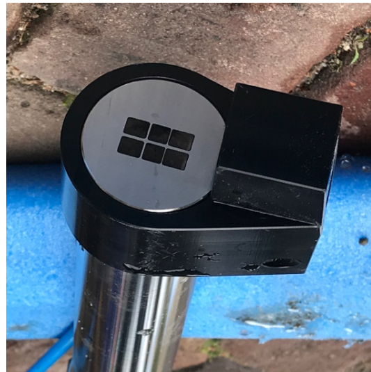
Figure C - 12: Turbidity sensor fouling ( top ), before ( left ) and after cleaning ( right )
