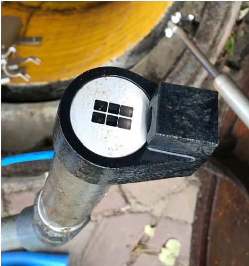
Figure C - 12: Turbidity sensor fouling ( top ), before ( left ) and after cleaning ( right )
