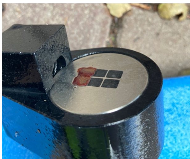
Figure C - 13: Biofouling on turbidity sensor 2 (MP2, September 9 th )
