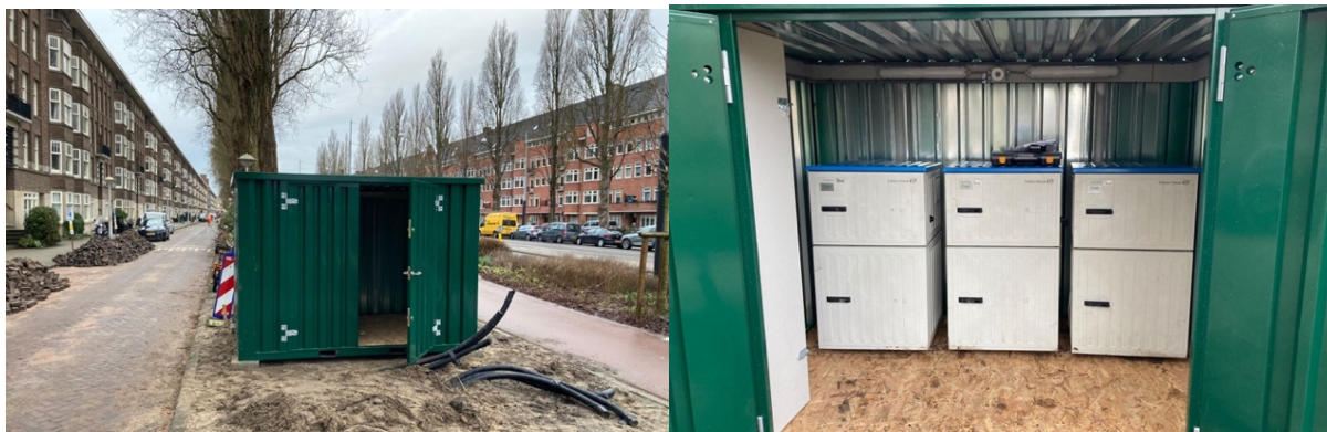
Figure 14: Installed instrumentation container adjacent to the service road (left) with samplers inside (right)
