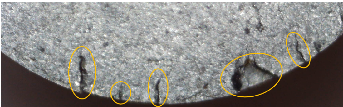
Figure 7.15: TB2 specimen showing multiple sharp, surface-connected discontinuities extending radially inwards from the specimen edge (highlighted)
