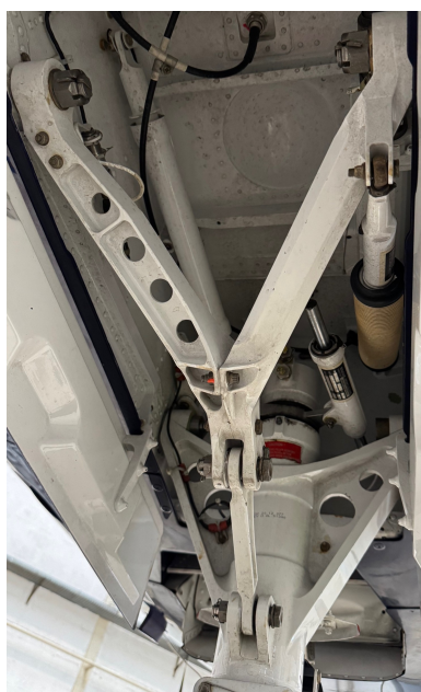
(a) Configuration A: compact, straight drag brace with over-centre locking mechanism
