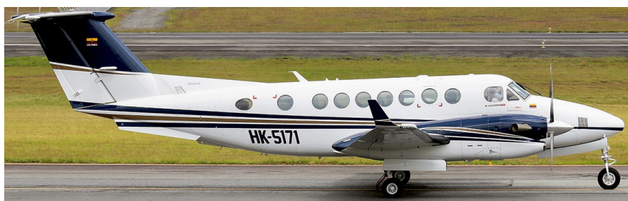
Figure 2.11: Beechcraft King Air 300 nose-wheel landing gear with forward-offset nose wheels and aft-folding drag brace [41]
