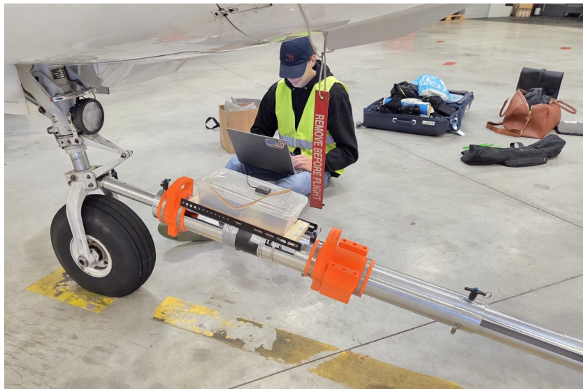
Figure 5.10: Wireless connection initialisation before towing manoeuvres
