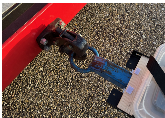
Figure 5.27: Towbar connection to towing vehicle via oversized ring (mechanical play)
