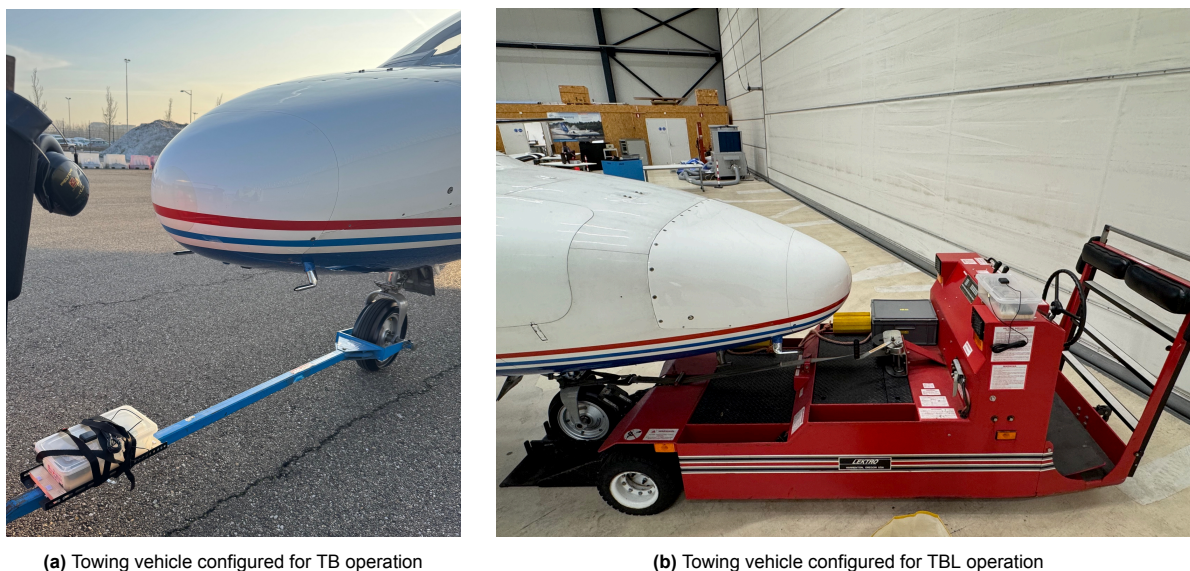
Figure 5.19: Same towing vehicle used for both experiments, shown in TB and TBL configurations
