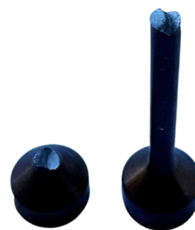
Figure 7.11: Fractured dog-bone specimen after fatigue failure
