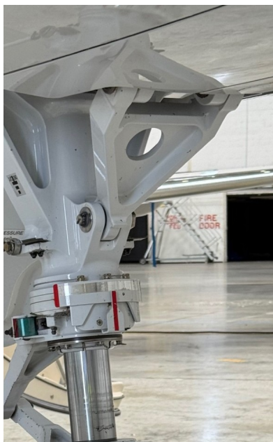
(b) Configuration B: forward-leaning V-shaped brace
