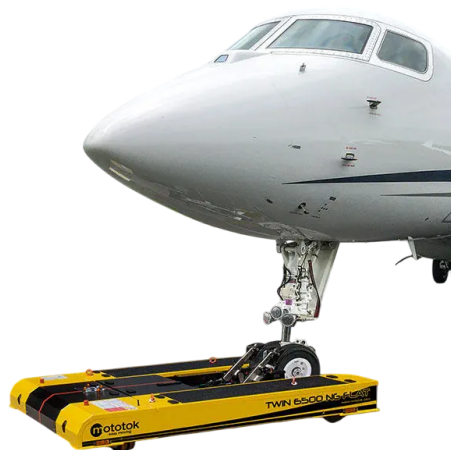
Figure 2.6: Towbarless towing configuration for GA aircraft [25]
