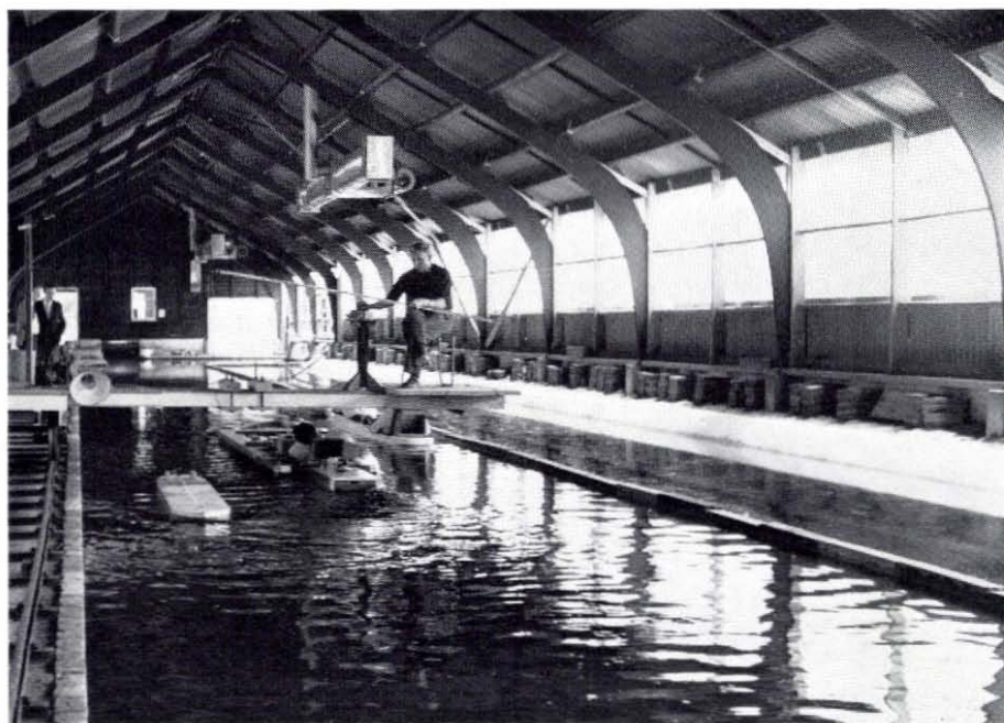
Photo 15. Model passing manoeuvre. The push tow and tow barge were steered by experienced skippers who determined the respective distances intuitively.
