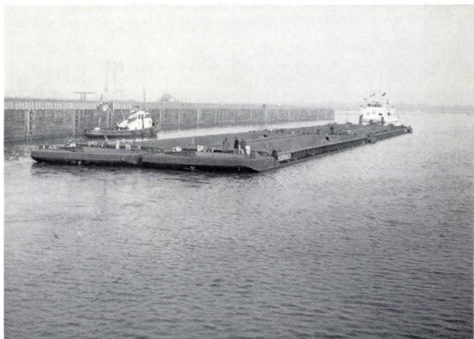
Photo 2. The push tow is not only considerably larger than other vessels but also different in shape, especially at the bow.
