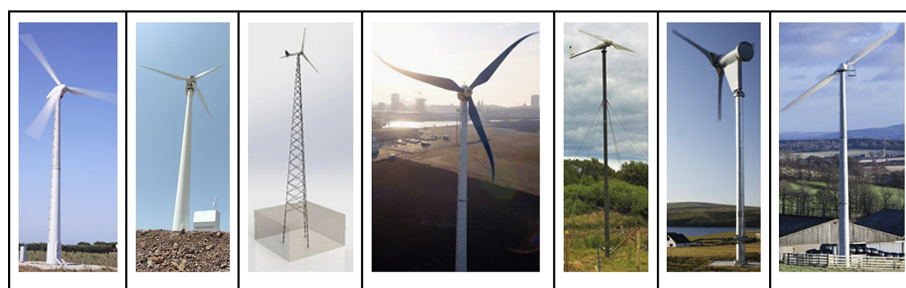
Figure 12. Common HAWT archetypes found on the current DWT market. From left to right: upwind, active pitch and yaw (photo credit: Tozzi Nord); upwind, stall-controlled and active yaw (photo credit: Eunice); upwind, stall-controlled and tailed passive yaw (photo credit: NREL pix 49511); downwind, stall-controlled and passive yaw (photo credit: Ecocycle – formerly XANT); upwind, tailed passive yaw, furling (photo credit: Bornay); downwind, pitch- or pitch-coning-controlled, passive yaw (photo credit: SD Wind, formerly Proven); downwind, stall-controlled, passive yaw and teeter (photo credit: Ryse Energy, formerly Gaia).
