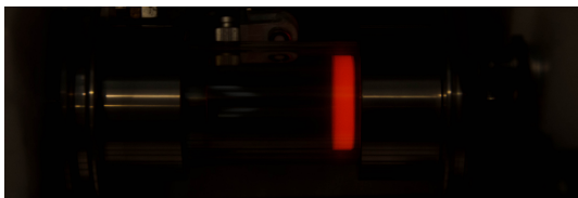
Figure 4.21: Incandescent glow of the cathode, after the plasma extinguished; ISO400, 1/30s, f5.6
