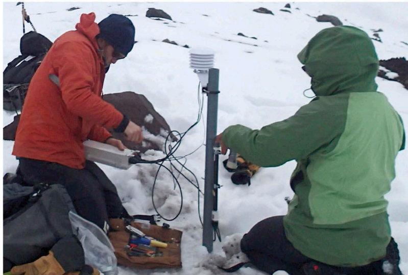
Figure 6. Andy Wickert (left) and Rachel McLaughlin (right) construct a glacier monitoring station to measure snow depth, ice melt, temperature and relative humidity on Volcán Chimborazo, Ecuador, where tropical glaciers are rapidly retreating (La Frenierre and Mark 2017). The monitoring station is built from off-the-shelf components, and is centred around an open-source ALog data logger (inside the white box in AW's hand) which records measurements at constant time intervals. Expanding use of low-cost, low-power and off-the-shelf environmental monitoring tools is critical for data collection in remote areas (Wickert 2014), especially those that are experiencing rapid environmental change which threatens communities with limited resources (La Frenierre and Mark 2014).
