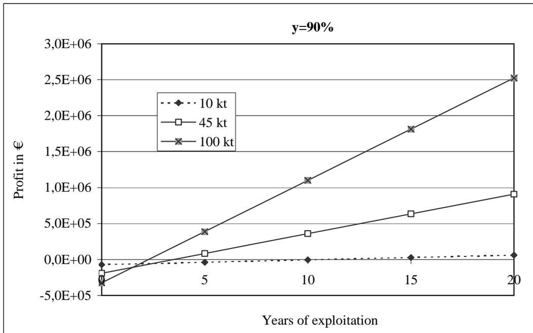
Figure 7.4: Profit over exploitation time with 90% yield for naphthalene and propene for a given capacity.
