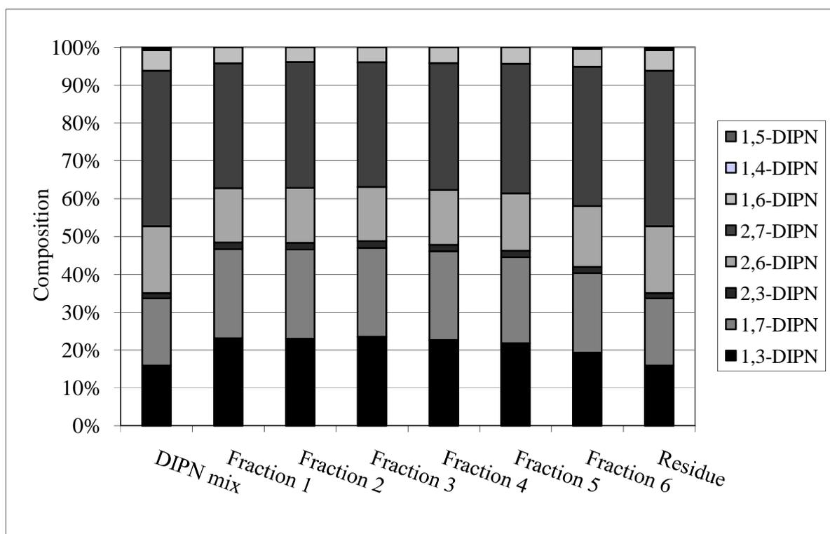
Figure 6.2: Composition of the different distillation fractions.
