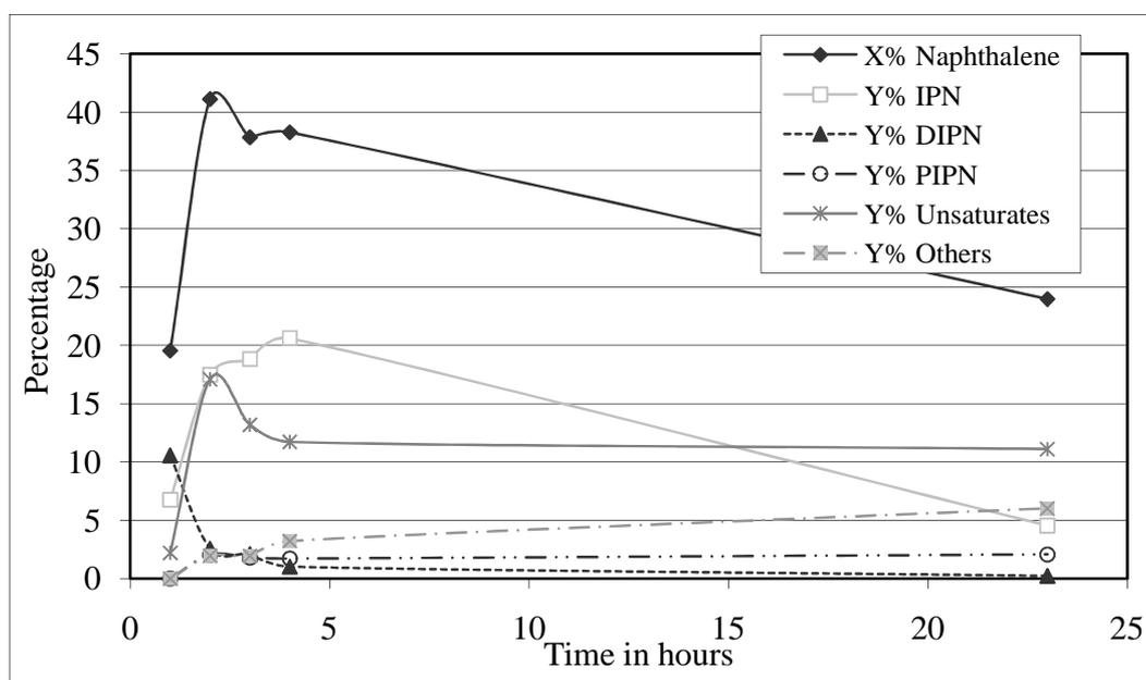
Figure 3.7: Naphthalene Conversion (X) and Yields (Y) to various product families in the isopropylation of naphthalene over H-Beta in time.
