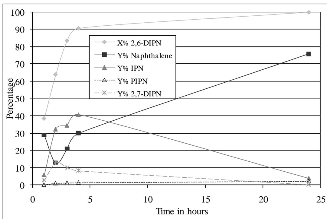
Figure 3.8: 2,6-DIPN conversion (X) and yields (Y) to various products in the isomerisation of 2,6-DIPN over H-Beta in time.
