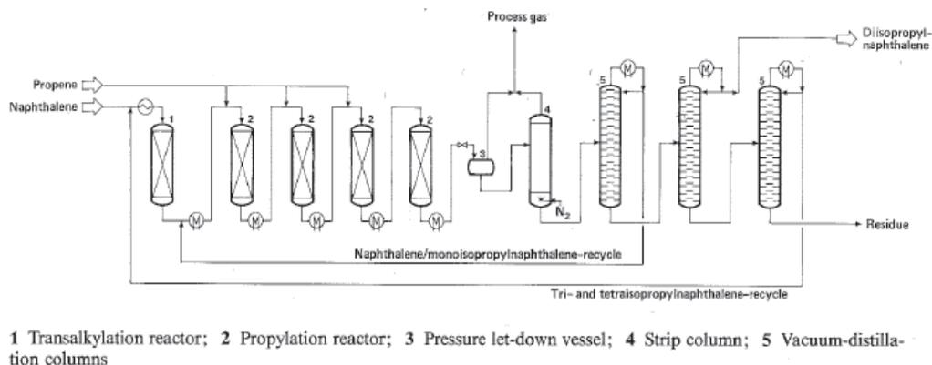
Figure 7.2: Flow diagram of the Kureha process
