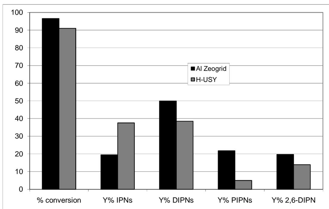
Figure 4.10: Product distribution over ZG (50) and H-USY in the isopropylation of naphthalene at 200°C after 24 h.
