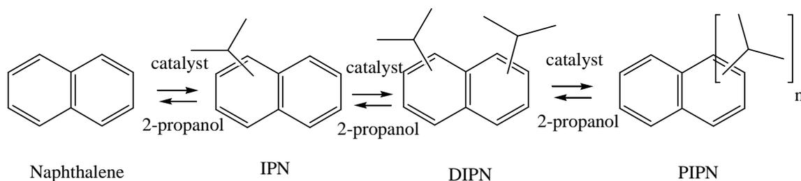
Figure 2.9: The different reaction steps in catalytic naphthalene isopropylation.
