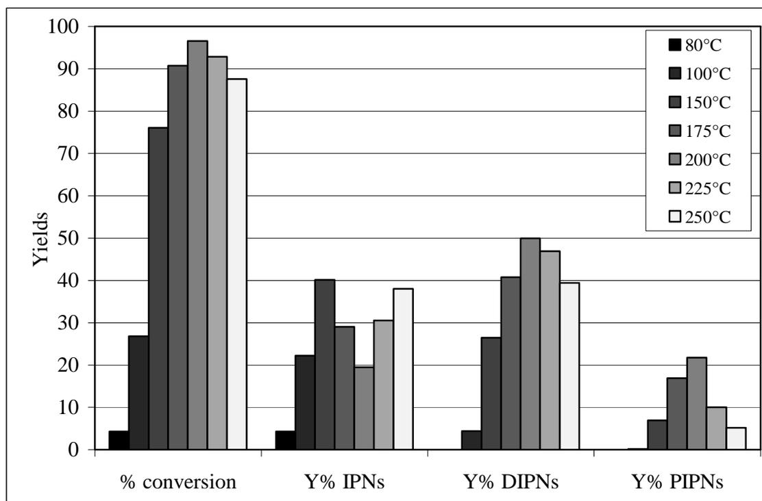
Figure 5.4: Yields towards specific families as a function of temperature in the isopropylation of naphthalene over the ZG (50).
