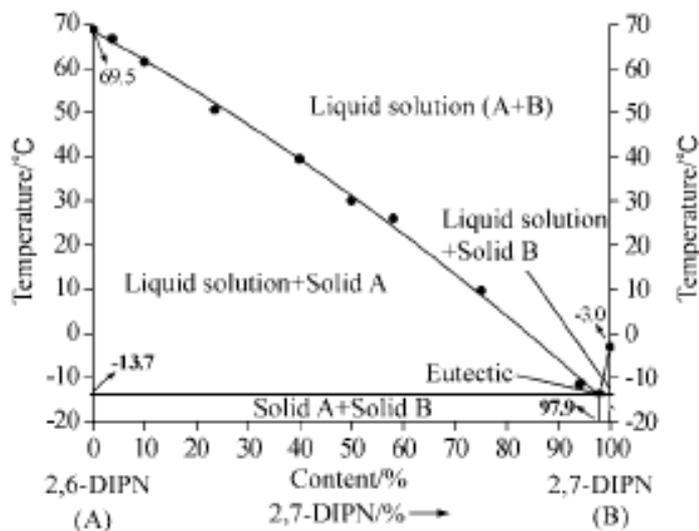
Figure 6.3: Phase diagram of the binary mixture as given in [4]
