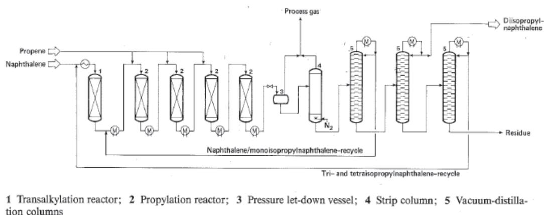
Figure 5.7: Flow diagram of the Kureha process
