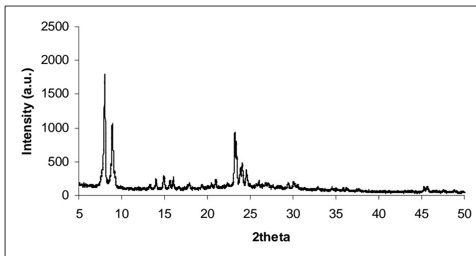
Figure 4.7: XRD pattern for the cZSM-5 (50) sample at high angle.
