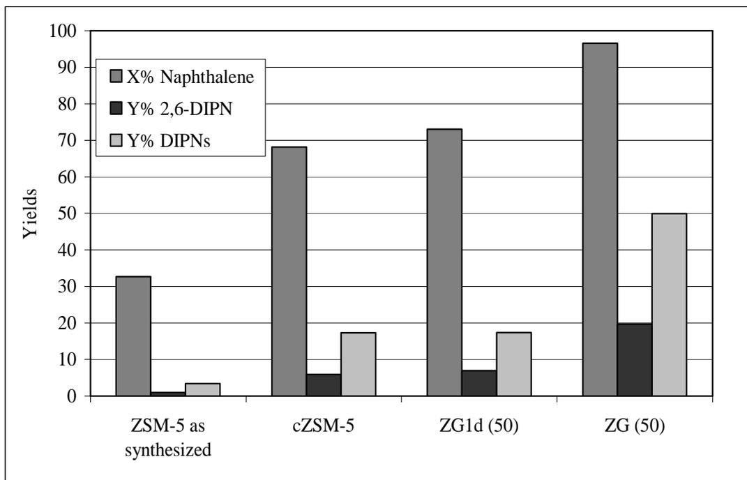
Figure 4.8: Naphthalene Conversion (X) and Yields (Y) of various products in the isopropylation of naphthalene over the four catalyst samples of Table 4.1.
