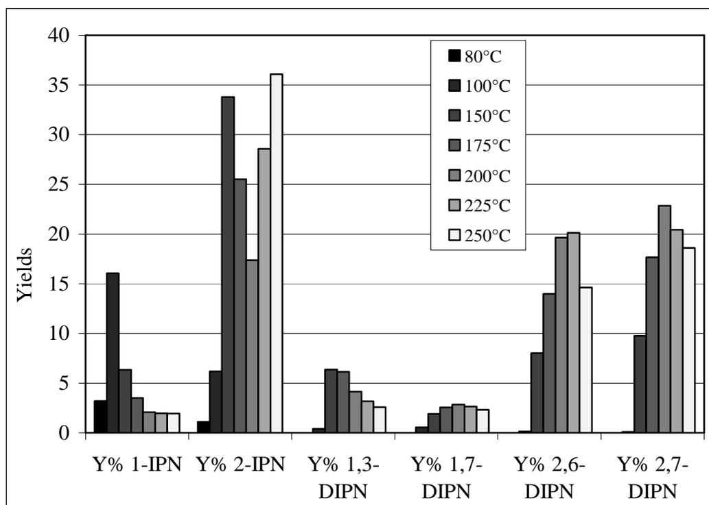
Figure 5.5: Specific yield as a function of temperature in the isopropylation of naphthalene over the ZG (50).
