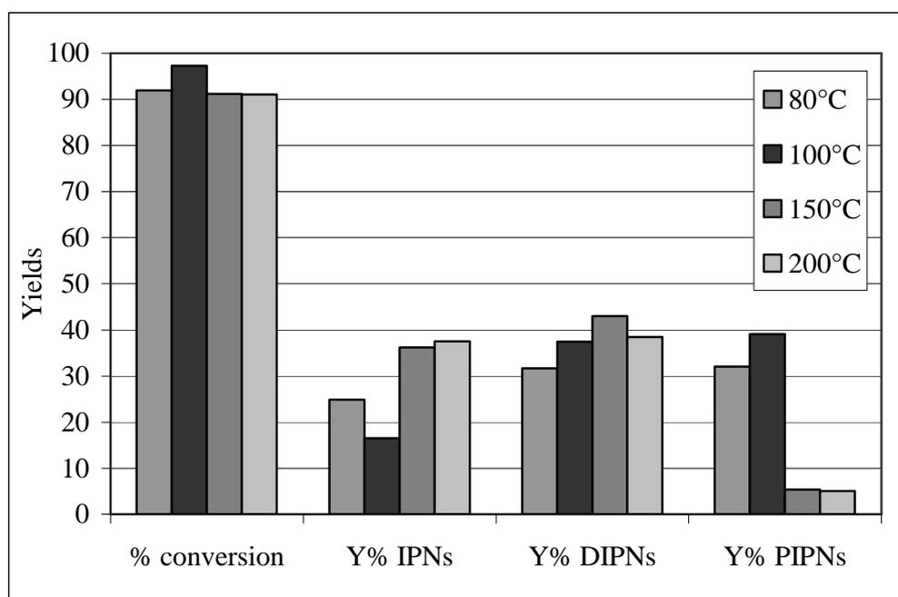
Figure 5.1: Yields towards specific families as a function of temperature in the isopropylation of naphthalene over H-USY.
