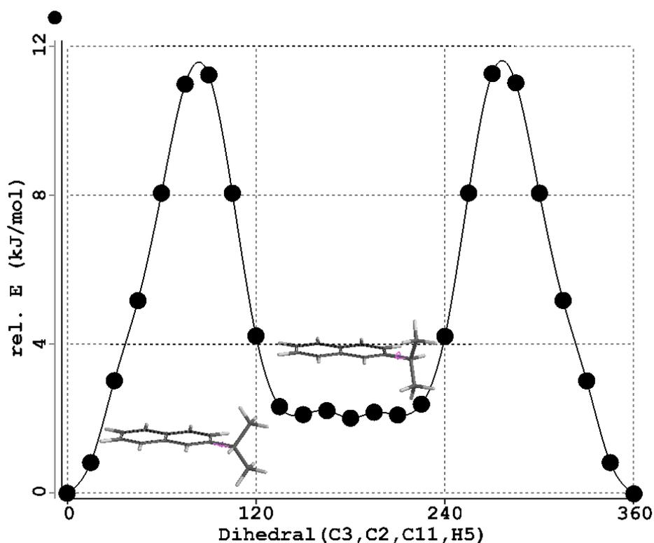
Energy diagram of complete rotation of the isopropyl group of 2-IPN (B3LYP/6-31G\*) showing the 2 conformers, differing  $\sim 2$  kJ/mol in stability, and separated by a rotation barrier of  $\sim 11$  kJ/mol.
