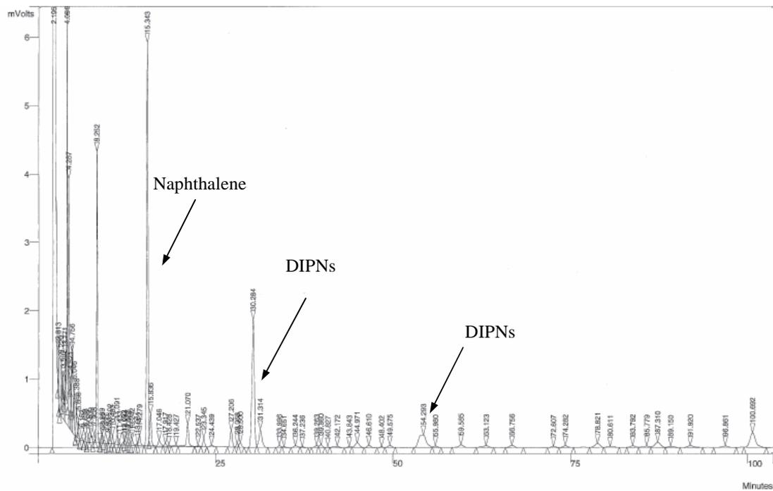
Figure 2.11: Chromatogram for the alkylation of naphthalene with 2-propanol over  $\text{AlCl}_3$  after 5 h.
