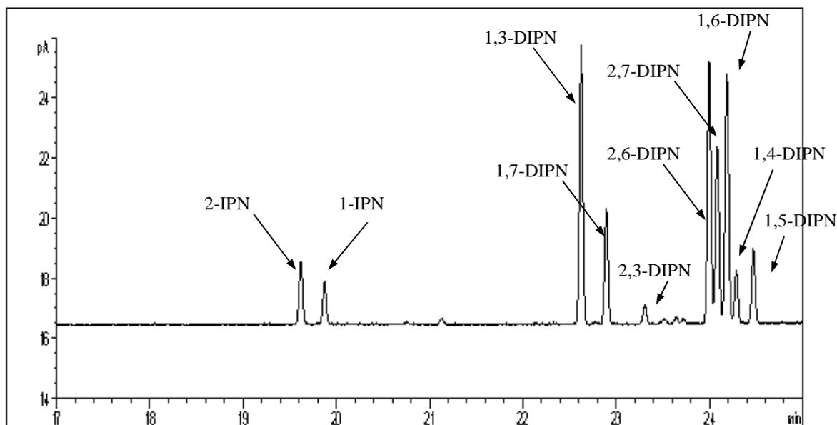
Figure 2.2: Typical chromatogram displaying the 2 IPNs and the main DIPNs.
