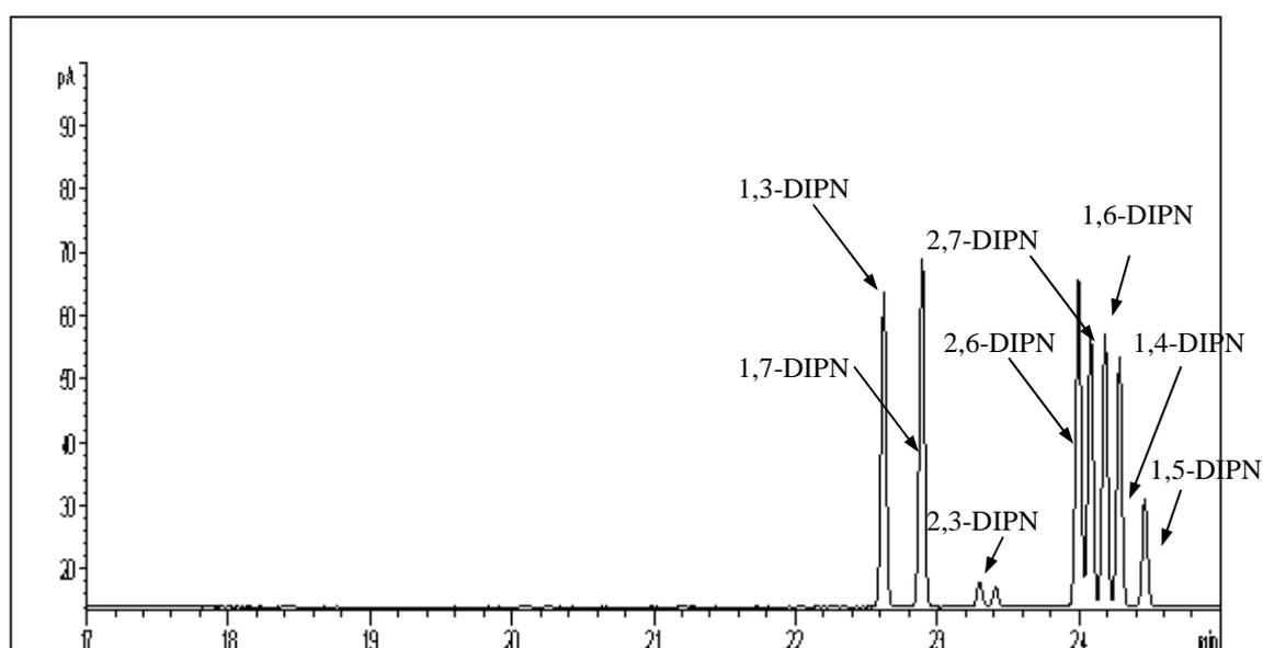
Figure 6.1: GC chromatogram of the commercial isomer mixture.
