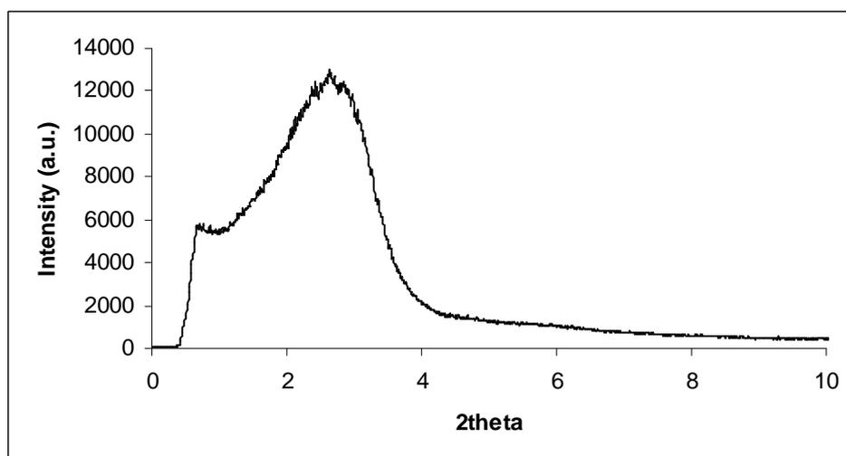
Figure 4.6a: XRD pattern for the ZG1d (50) sample at low angle.
