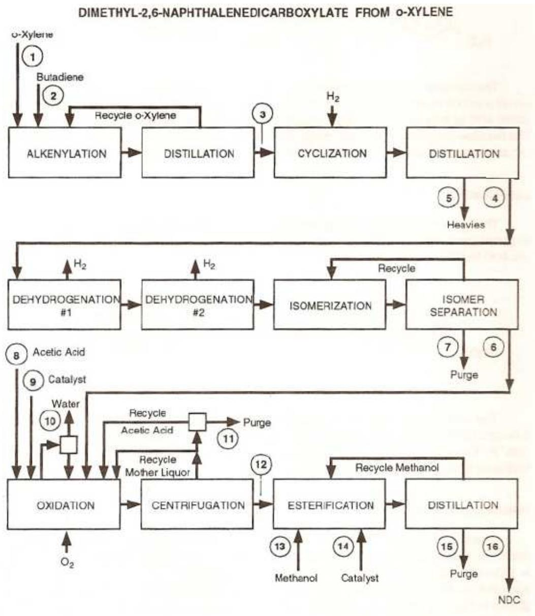
Figure 1.4: Block diagram from the Amoco process as presented in the SRI report [25]
