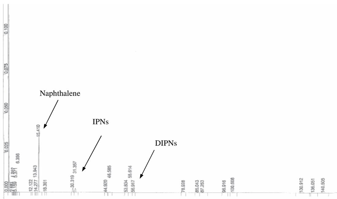
Figure 2.12: Chromatogram for the alkylation of naphthalene with 2-propanol over H-Mordenite after 20 h.
