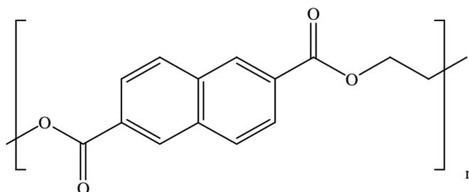
Figure 1.3: Structure of the PolyEthylene Naphthalate
