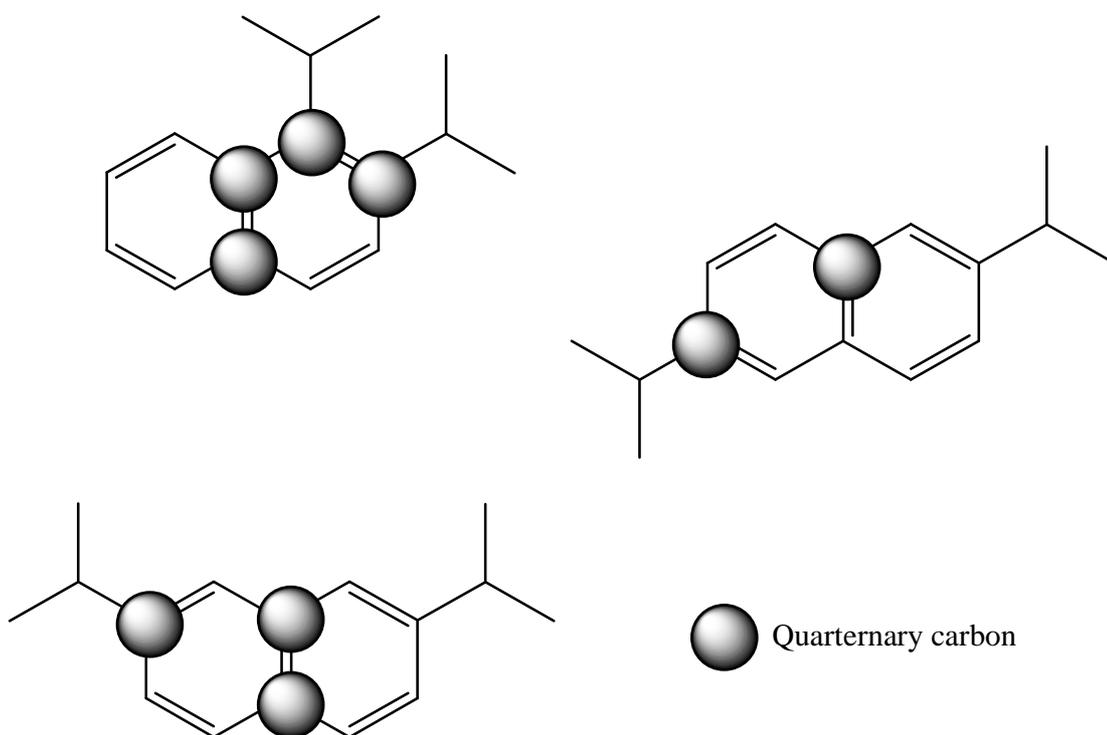
Figure 2.6: The different quaternary carbons with respect to symmetry.
