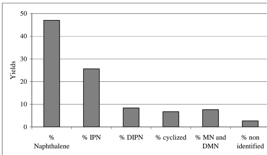
Figure 2.10: Product distribution of the alkylation of naphthalene with 2-propanol over  $\text{AlCl}_3$  after 5 h.
