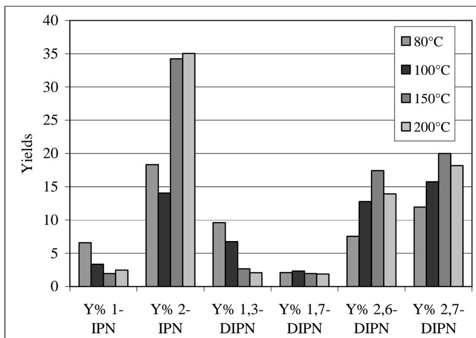
Figure 5.2: Specific yields as a function of temperature in the isopropylation of naphthalene over H-USY.
