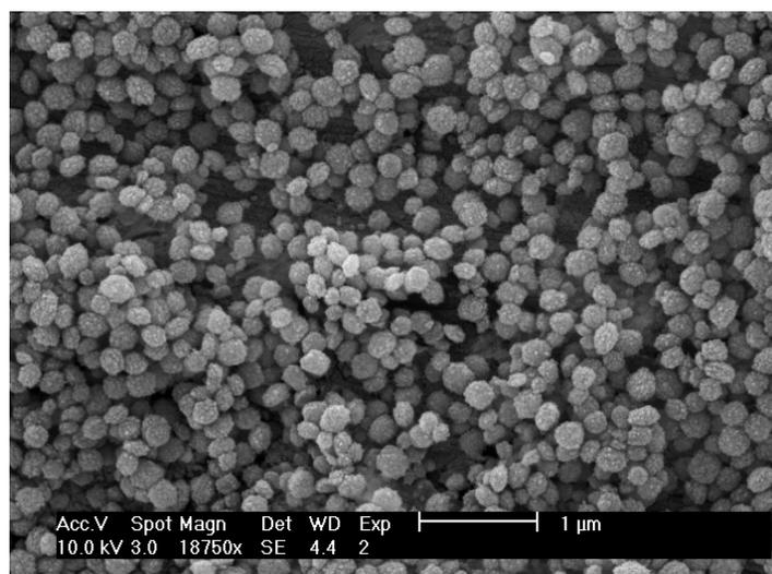
Figure 4.4: SEM picture of the cZSM-5 (50)
