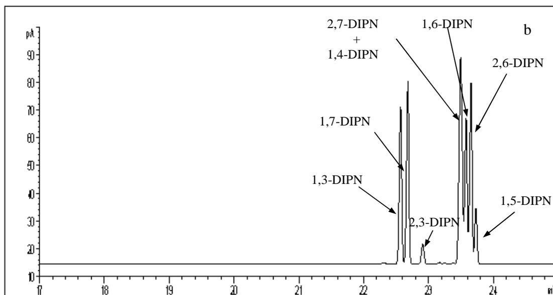
Figure 2.4: Chromatogram of a 2,6-DIPN/2,7-DIPN 1:1 mixture (a) and of the commercial DIPN mixture (b) on the CP-Sil-8 column.
