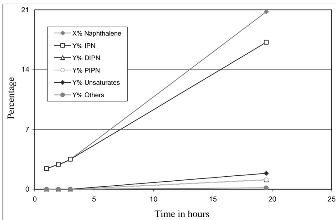
Figure 3.5: Naphthalene Conversion (X) and yields (Y) of various products in the isopropylation of naphthalene over H-Mordenite against time.
