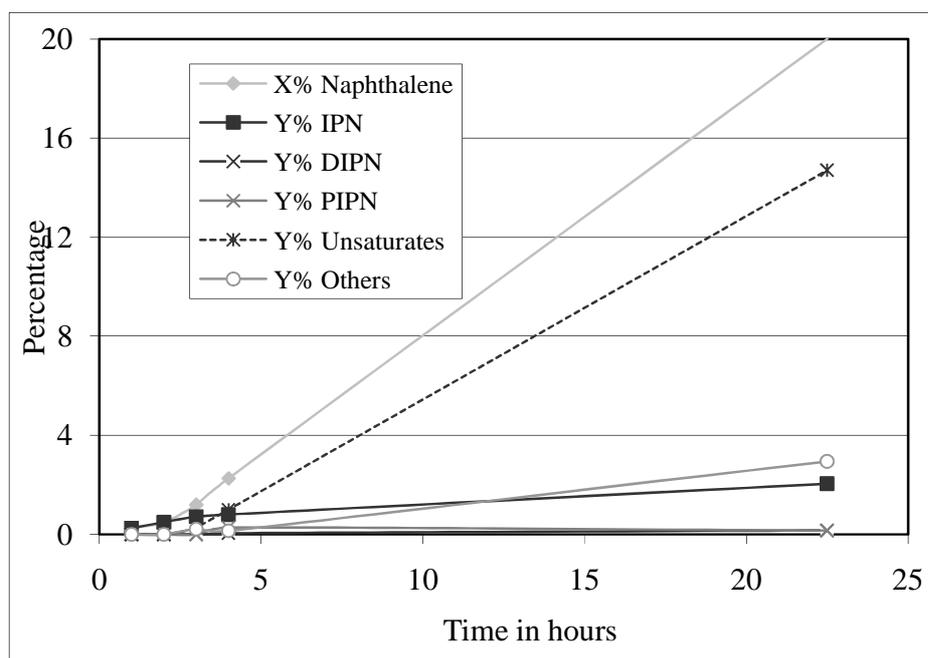
Figure 3.9: Naphthalene Conversion (X) and Yields (Y) to various product families in the isopropylation of naphthalene over H-ZSM-5 in time.
