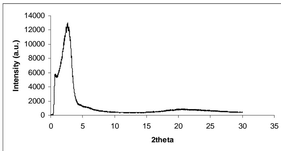
Figure 4.5b: XRD pattern for the ZG (50) sample at high angle.
