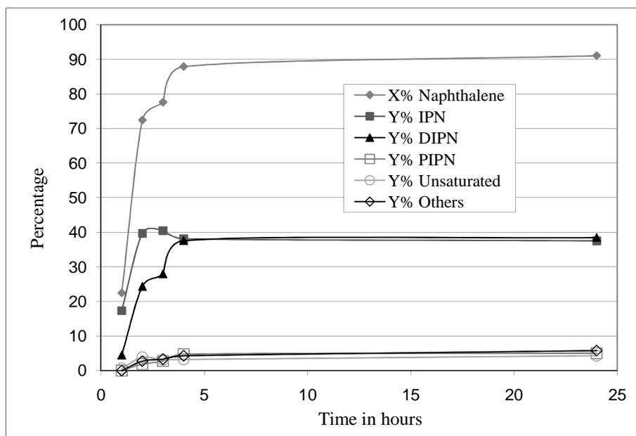
Figure 3.3: Naphthalene Conversion (X) and Yields (Y) of various products in the isopropylation of naphthalene over H-USY against reaction time
