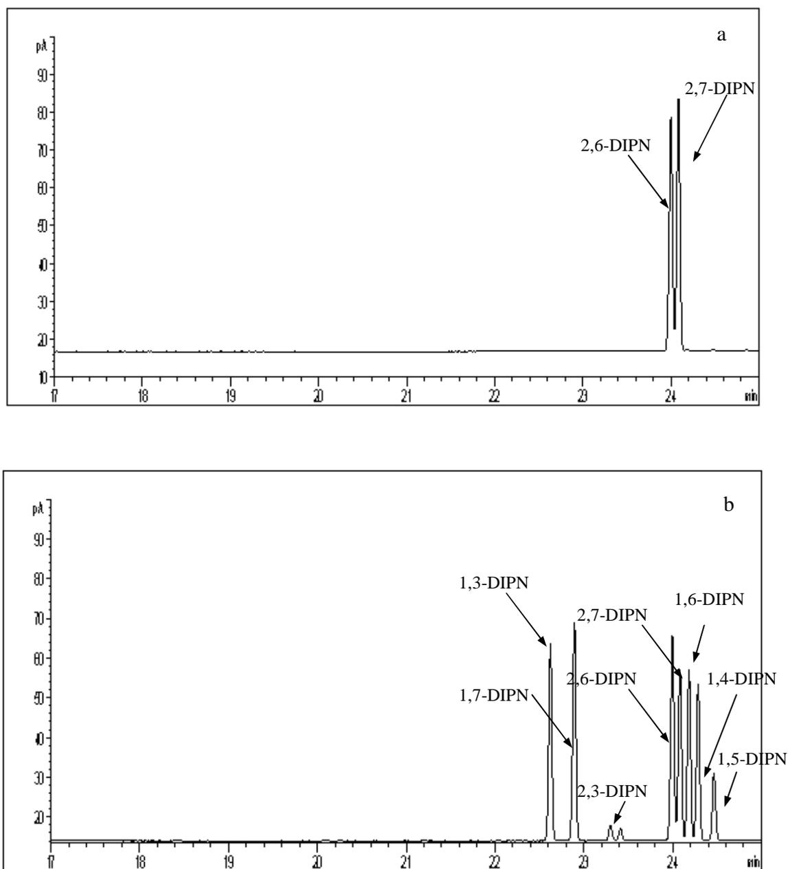
Figure 2.3: Chromatogram of a 2,6-DIPN/2,7-DIPN 1:1 mixture (a) and of the commercial DIPN mixture (b) on the CP-Wax-52 column.
