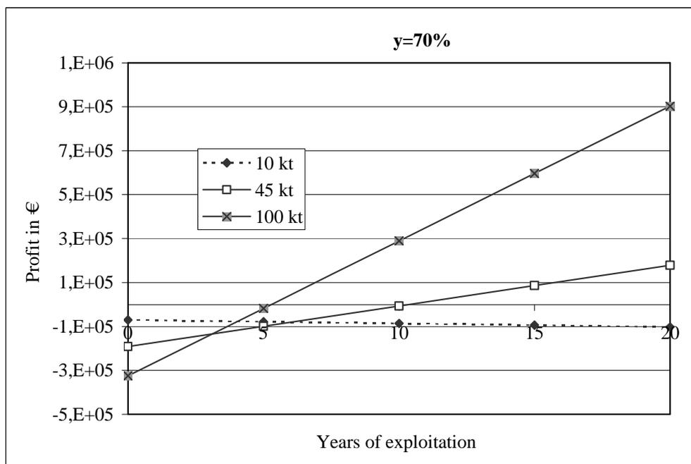
Figure 7.3: Profit over exploitation time with 70% yield for naphthalene and propene for a given capacity.
