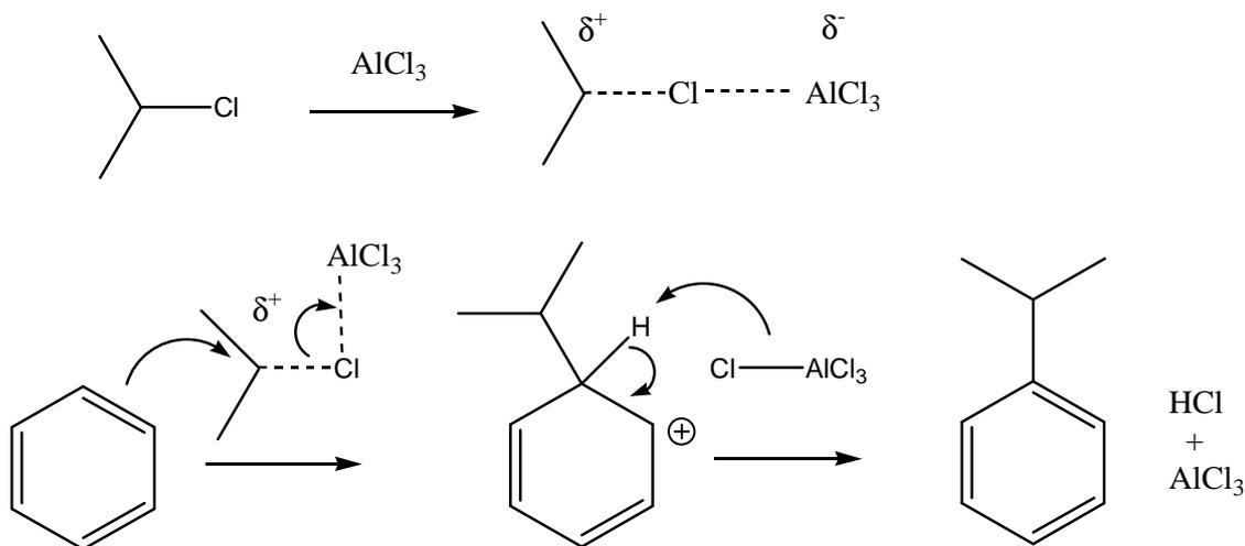
Figure 2.8: Friedel-Crafts classical alkylation mechanism with AlCl<sub>3</sub> as catalyst and isopropyl chloride as reactant.
