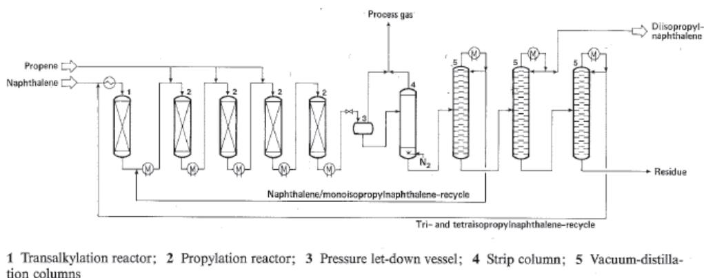
Figure 1.2: Flow diagram of the Kureha process
