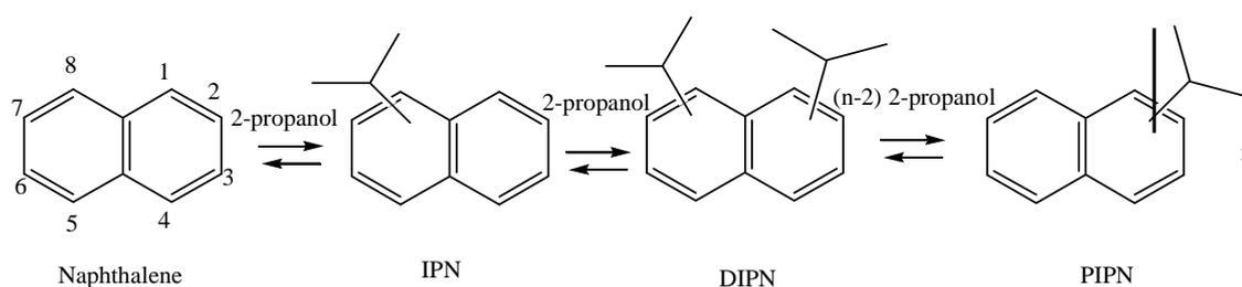
Figure 3.1: Consecutive reaction steps in catalytic naphthalene isopropylation.
