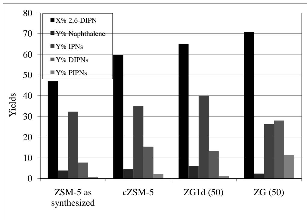
Figure 4.9: 2,6-DIPN Conversion (X) and Yields (Y) of various products in the isomerisation of 2,6-DIPN over the four catalyst samples of Table 4.1.
