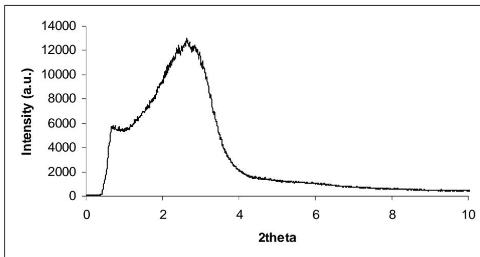
Figure 4.5a: XRD pattern for the ZG (50) sample at low angle.
