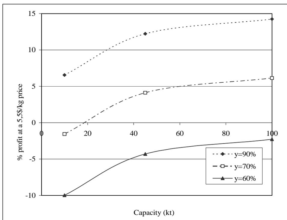
Figure 7.5: Profit percentage generated for a sell price of 5.5 €/kg as a function of production capacity.
