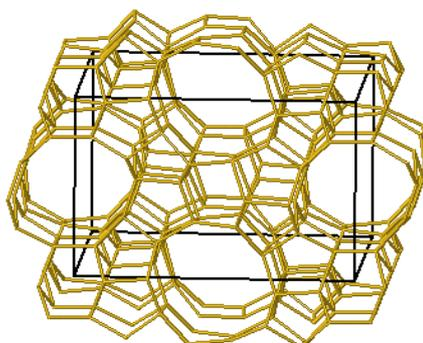
Figure 2.16: unit cell for an MFI-type zeolite.
