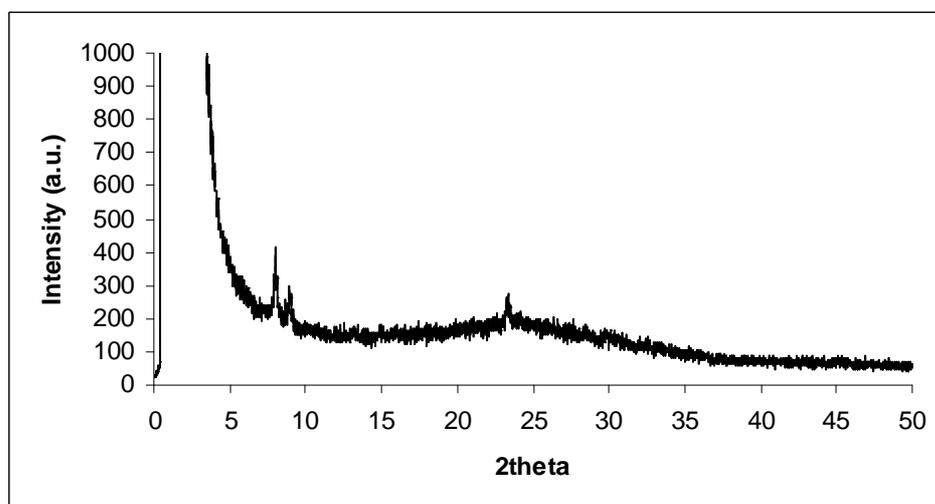
Figure 4.6b: XRD pattern for the ZG1d (50) sample at high angle.
