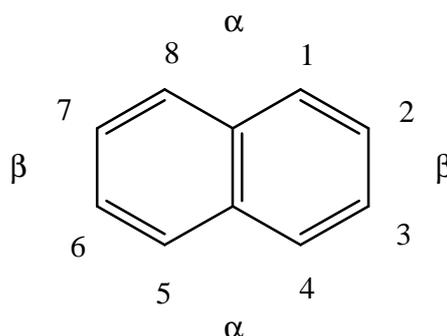
Figure 2.1: Nomenclature for substituent positions of naphthalene.
