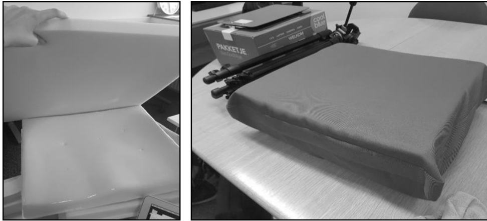
Figure 5: On the left: the prototype after thermoforming and adding the foam layer. On the right: the final model where the shape is hidden not to influence participants' expectations
