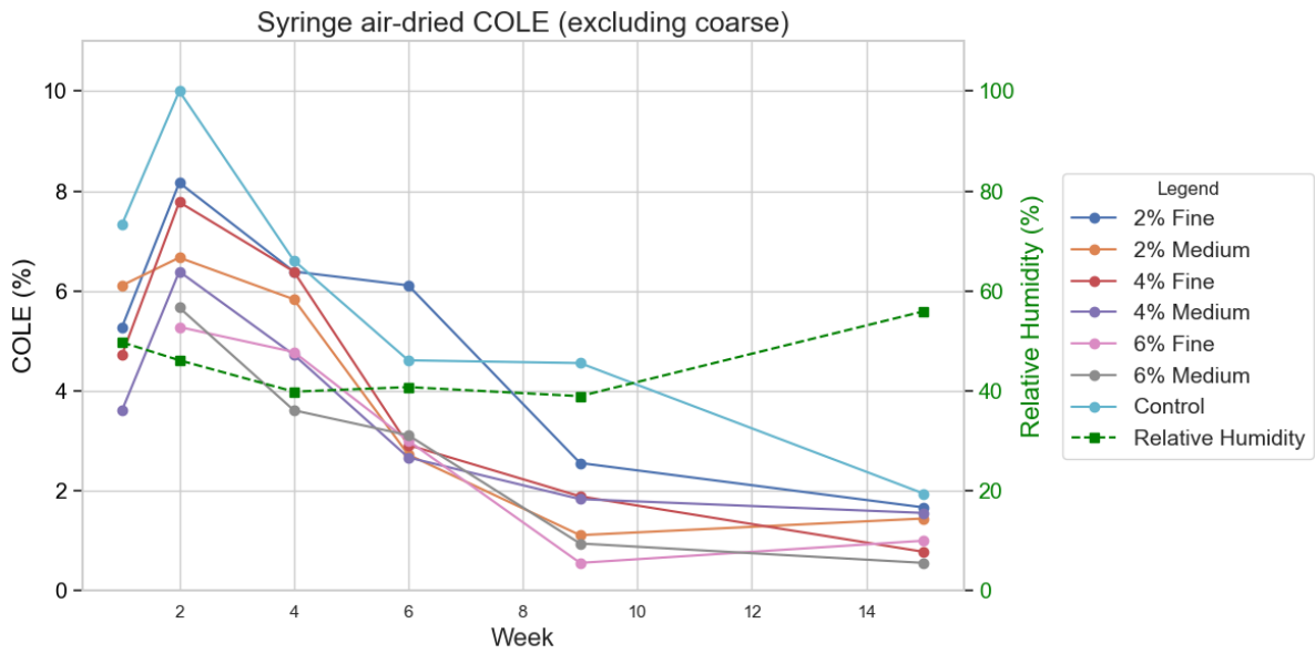
Figure E.3: Air dried syringe COLE and room relative humidity
